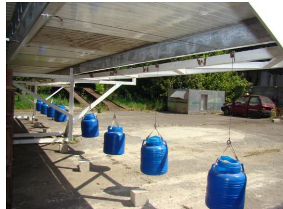
Distributed load applied to tested specimen
