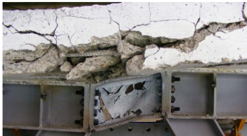
Failure mode of the detachable link (composite beam)
