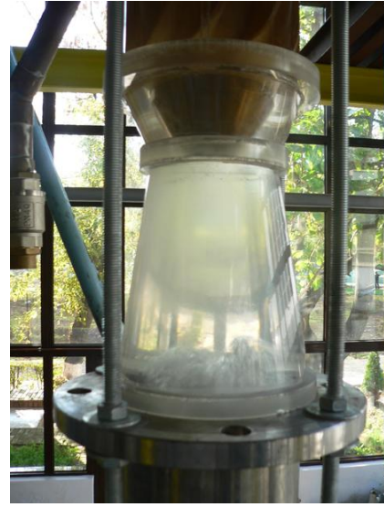
Vortex rope mitigation in the draft tube cone of a Francis turbine operating at partial discharge using the jet control technique.
