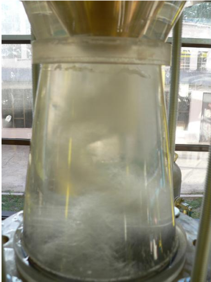
Vortex rope mitigation in the draft tube cone of a Francis turbine operating at partial discharge using the jet control technique.
