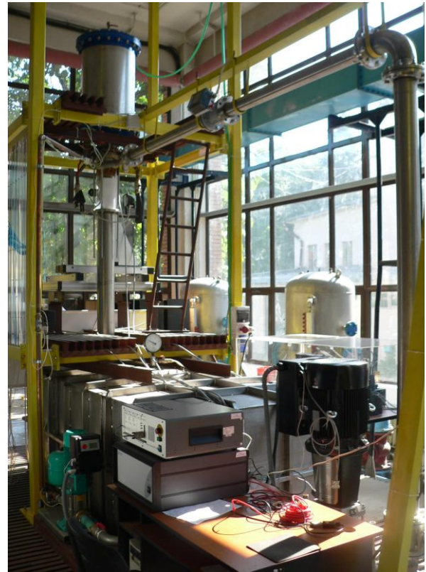
Closed loop test rig for experimental investigations of swirling flows and laser system to measure the velocity profiles
