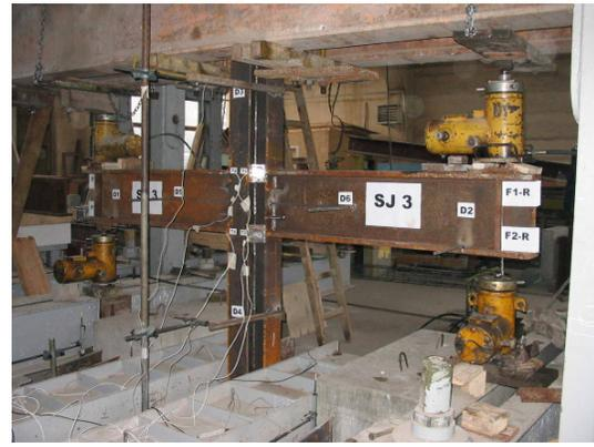
Figure 2.34. General view of testing equipment for asymmetrical load
