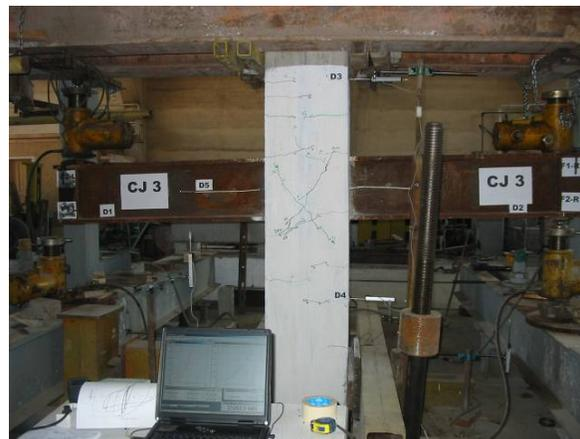
a. Distribution of cracks at the composite steel concrete joint during asymmetrical load test
