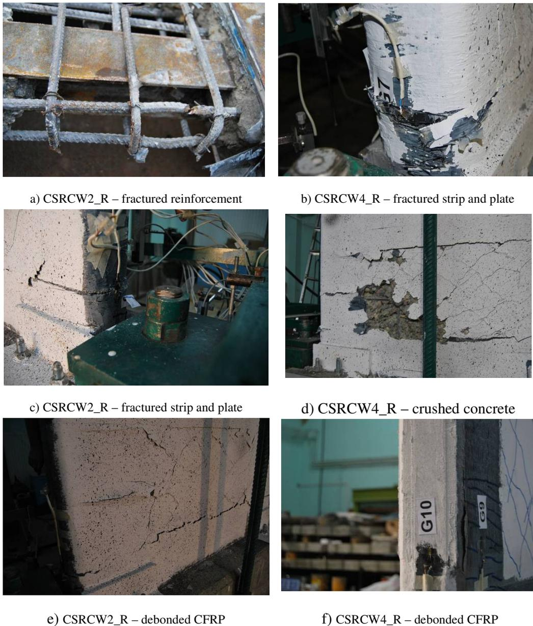
Figure 3.29 Failure details
