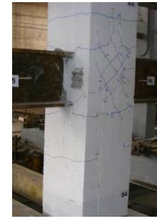
*c. Cracks distribution at failure*
