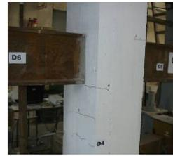
*b. Distribution of first cracks in joint and column*
