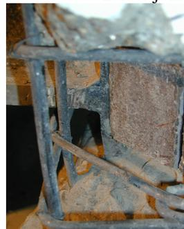
b. Tearing of vertical stiffener
