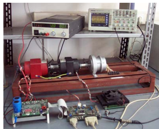
Testing the dynamic performances of a SR drive
