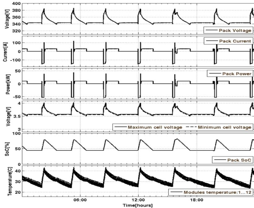
Fig. 4.16. Example of a repeated fast charging test cycling of the Kokam battery with a charge energy of 13 kWh (50 % of SOC) at constant current of 2C (150A) & discharging with C/3(25A).
