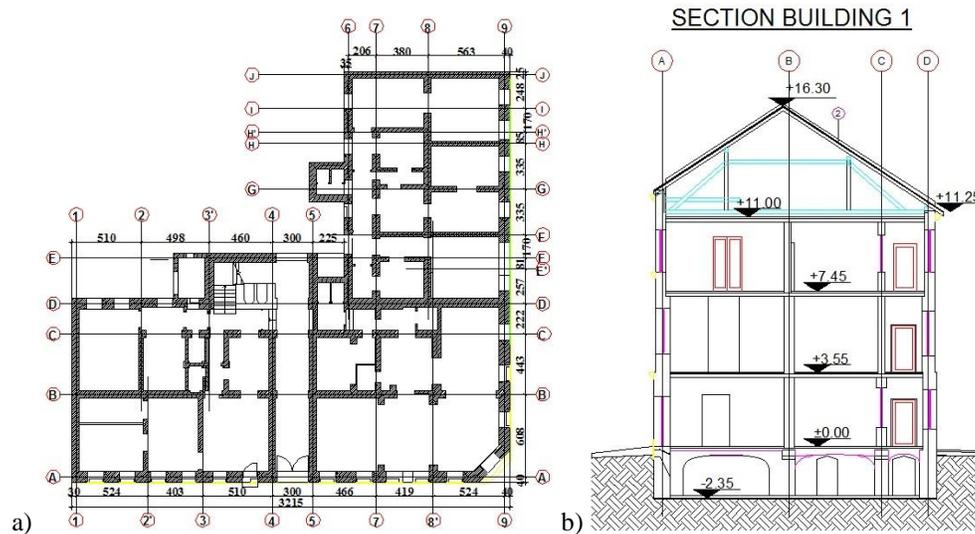
Fig. 5.16 Vertical and horizontal section of the building
