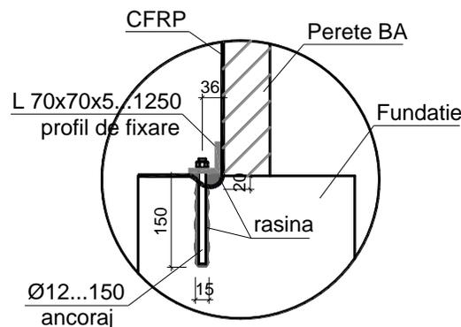
Fig. 2.8 Anchorage system of the carbon fibre strips
