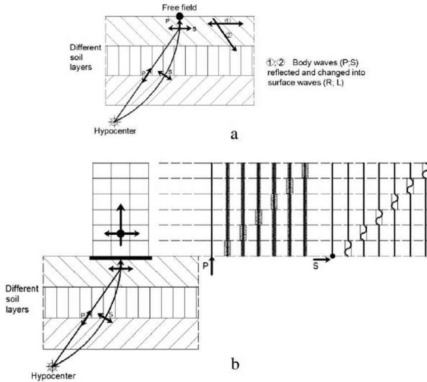
Fig. 3.39 Ground motion types: a) free site, b) site with structures
