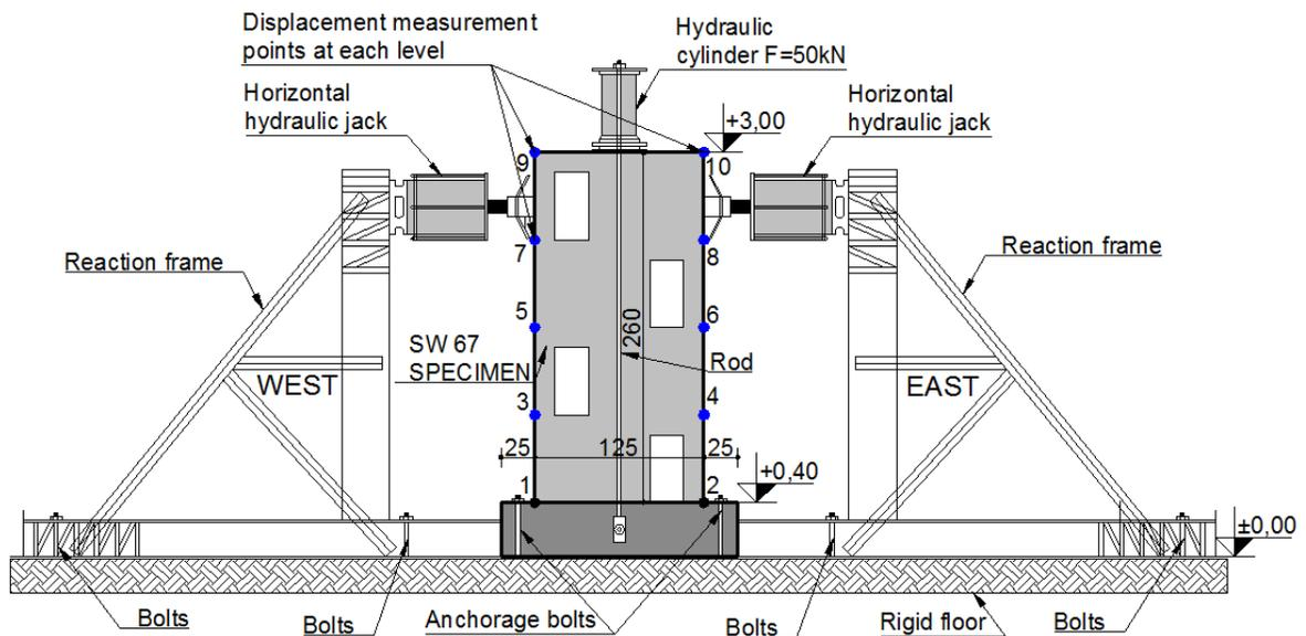
Fig. 2.5 Testing methodology
