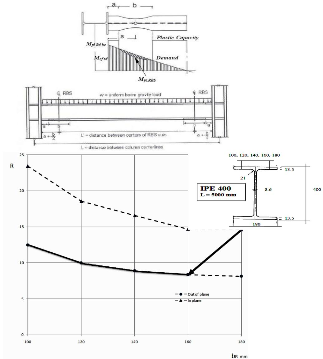
Fig. 11 Rotation capacity for RBS
