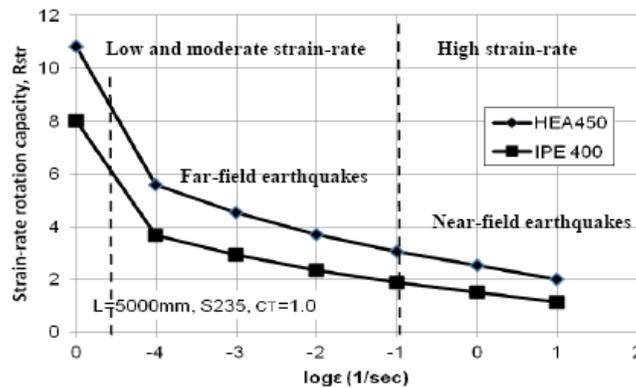
Fig. 3.44 The effects of the strain-rate on the rotation capacity
