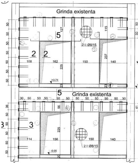
**Fig. 2.29** Reinforcement of the shear walls
