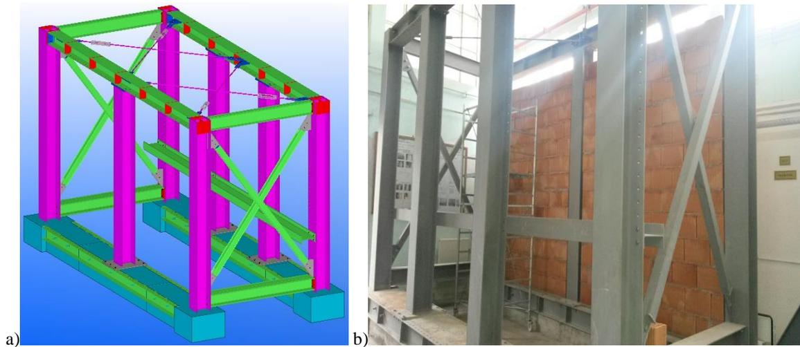
**Fig. 2.61** Experimental test stand a) Project phase, b) Complete phase with infill panel
