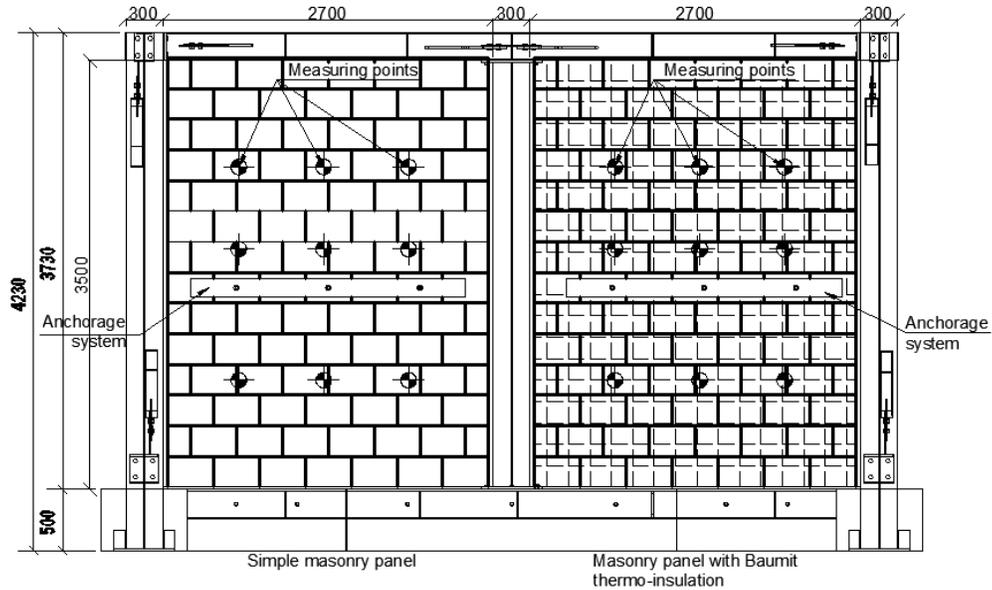
Fig. 7.1 Dimensions of the wall specimens
