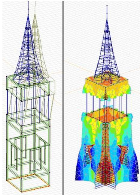
**Fig. 4.10** The deformed shape and state of efforts in the tower
