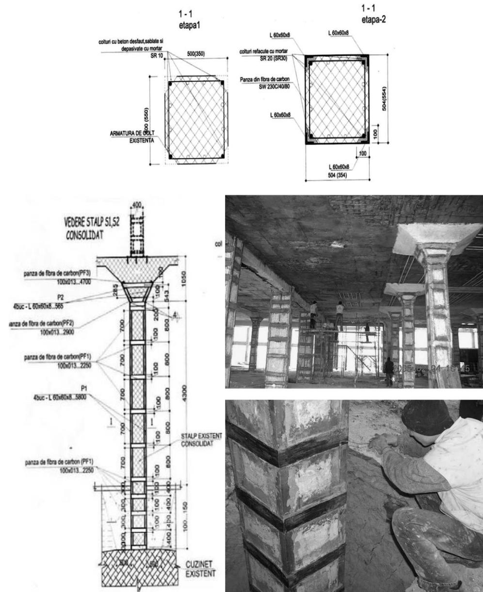
Fig. 2.46 Strengthening of columns
