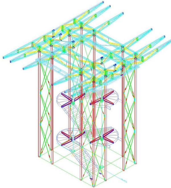
**Fig. 2.32** Steel structure of central tube
