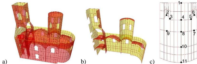
**Fig. 5.7** a) meshed structure; b) longitudinal section; c) measurement points of the unitary efforts
