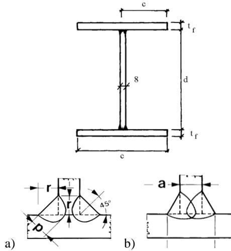
**Fig. 3.12** Welded I sections with a) fillet weld type, b) penetrated welds
