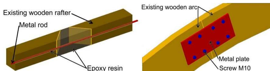
**Fig. 6.11** The consolidation solution of the wooden arches and rafters
