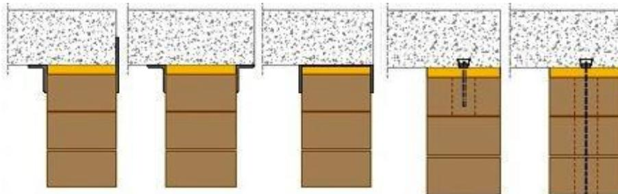
**Fig. 2.54** Horizontal displacement joint: current shelf angle connection and new solution with sliding connectors
