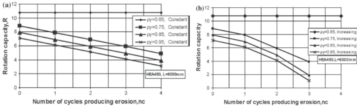
Fig. 3.36 Influence of the yielding ratio on the rotation capacity of HEA beams
