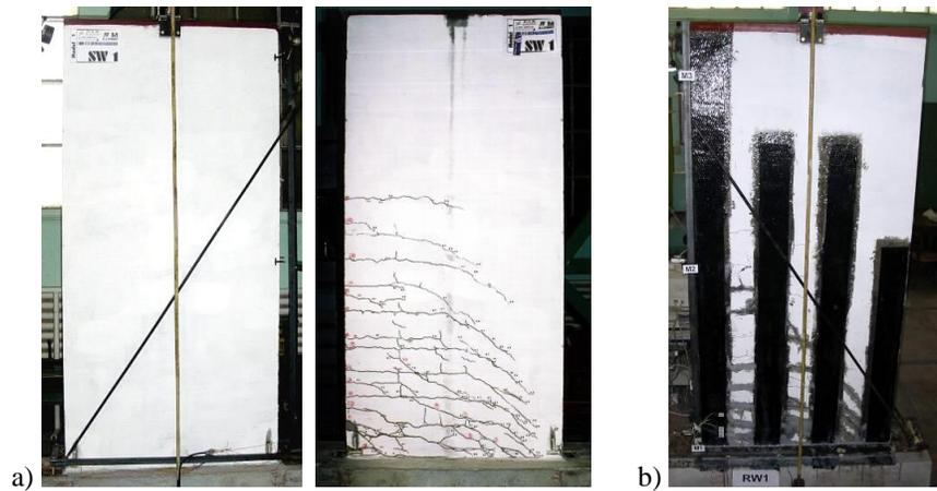
**Fig. 2.9** Test models a) before and after testing (SW1); b) after consolidation (RW1)
