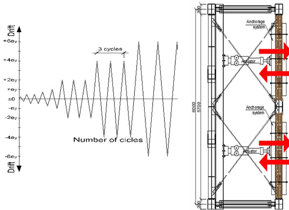
Fig. 7.2 Loading protocol and testing procedure
