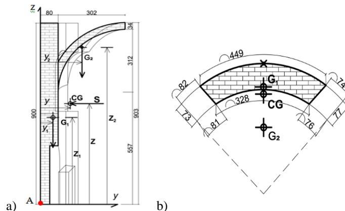
**Fig. 5.13** Failure block no. 4; a) vertical section b) in plan dimensions and positions of centres of gravity
