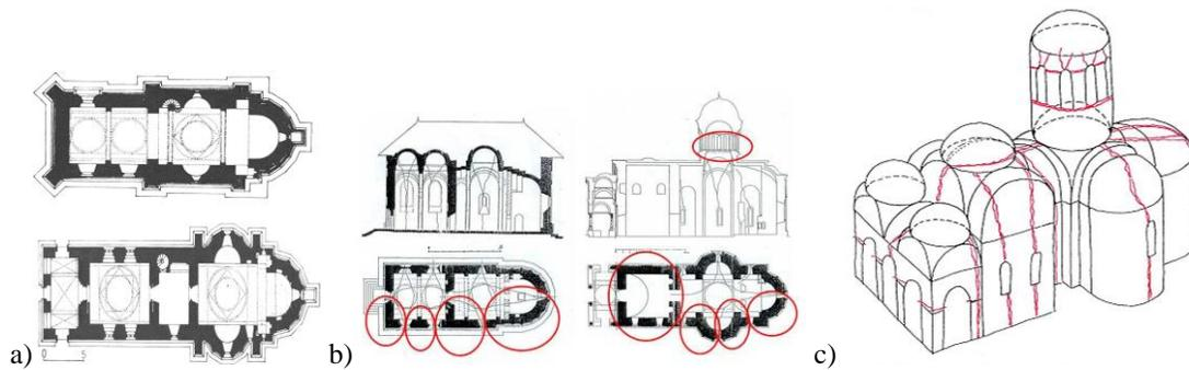
**Fig. 5.4** a) typical plans of Romanian orthodox churches; b) damage of Borzesti and Cozia churches due to 1977 Vrancea earthquake; c) failure blocks of Romanian orthodox churches [5.16]
