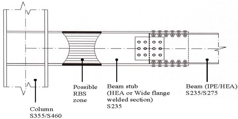
**Fig. 3.34** Structural detail enhancing the local cyclic ductility
