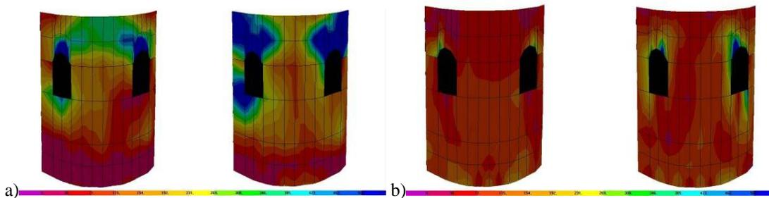
**Fig. 5.10** Stress diagram for East wall a) Tension stress S11; b) Compression stress S22
