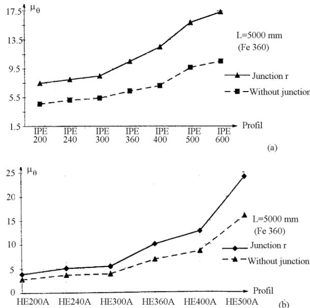
**Fig. 3.9** Influence of the junction on the rotation capacity of the steel hot-rolled I-beams
