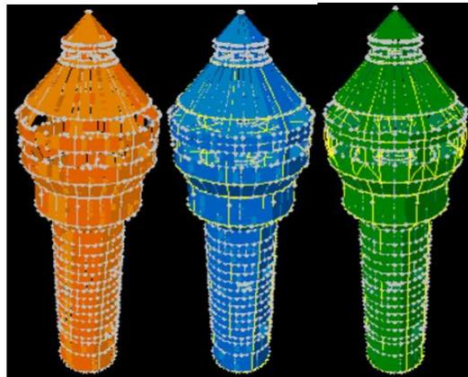
Fig. 4.7 Seismic Deformed shape of unconsolidated tower and solution 1 and 2 of consolidation
