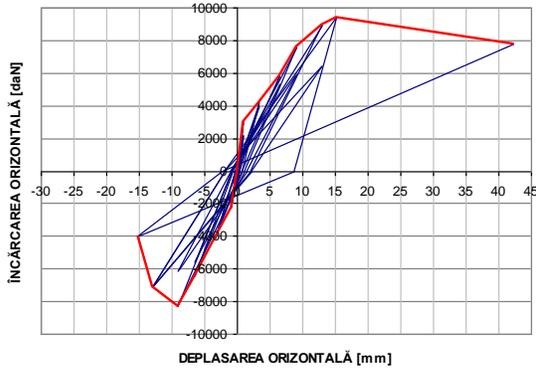
a) Force-displacement diagram of SW8
