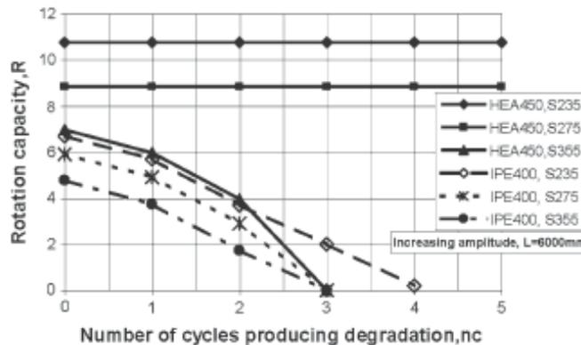
Fig. 3.37 Influence of the steel quality on the cyclic rotation capacity
