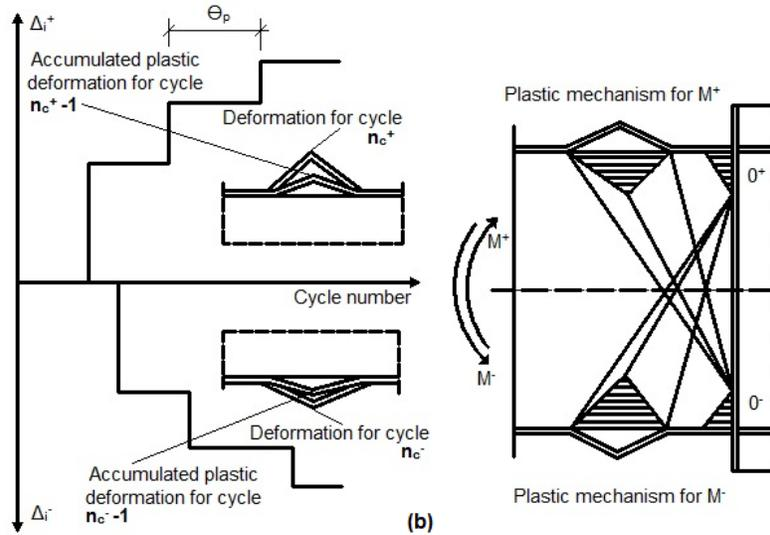
**Fig. 3.28** Plastic local mechanism for cyclic loading
