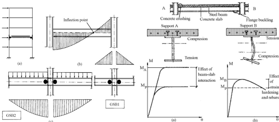
**Fig. 3.26** Behaviour of steel beams under real conditions and the use of the standard beam concept
