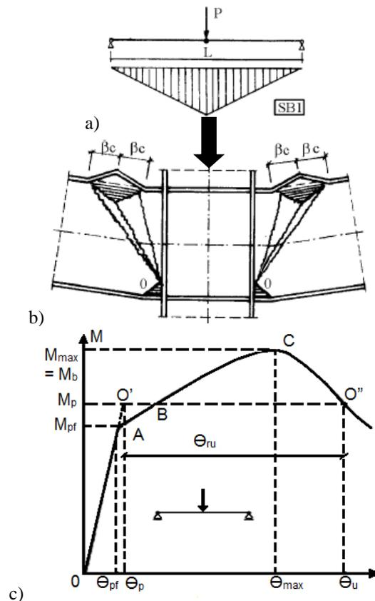
**Fig. 3.3** Local plastic mechanism for gradient moment: a) SB 1 standard beam, b) Local plastic mechanism, c) Actual moment-rotation curve
