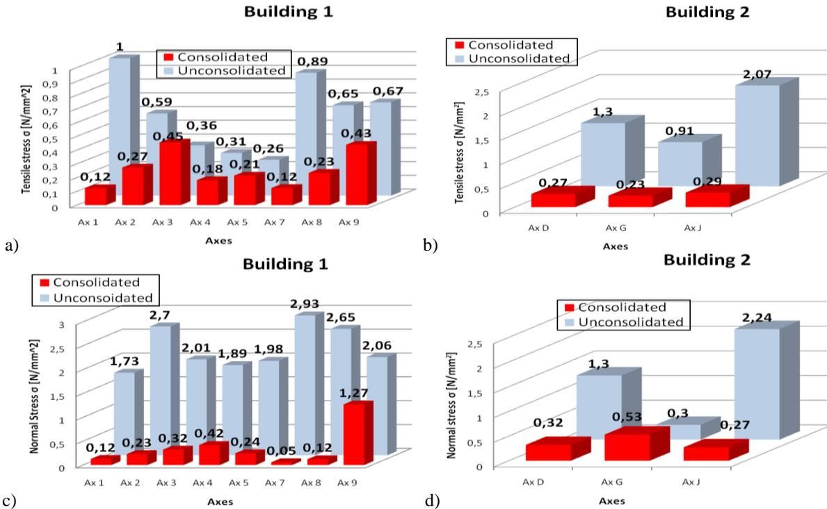
Fig. 5.27 Comparative values of maximum tensile and compressive stresses before and after strengthening of the buildings a, b) tensile stress, c-d) normal stress
