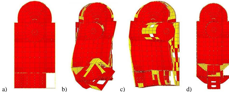
**Fig. 5.8** Modes of vibration a) undeformed; b) 1<sup>st</sup> shape mode; c) 2<sup>nd</sup> shape mode; d) 3<sup>rd</sup> shape mode
