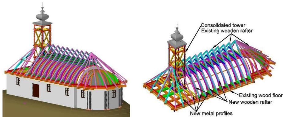
**Fig. 6.13** Consolidation solutions of the arches, rafters and wooden beams of the church
