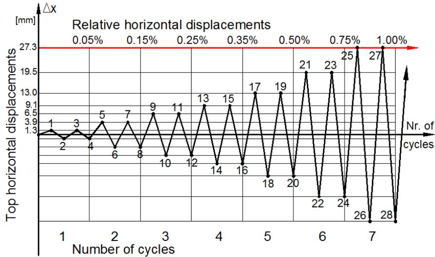
Fig. 2.6 Testing protocol
