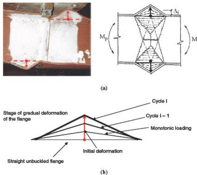
**Fig. 3.29** Accumulation of plastic deformation under cyclic loading
