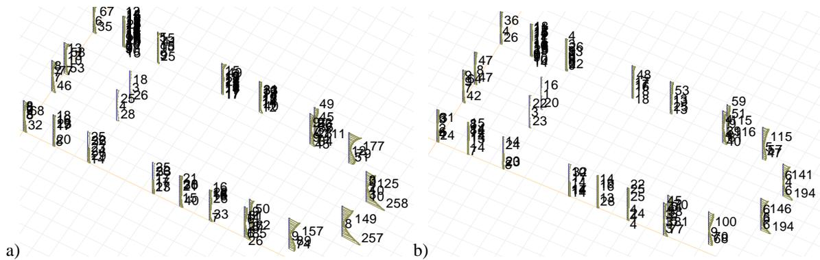
**Fig. 6.20** Maximum values of tensile stress in columns: a) before and b) after consolidation
