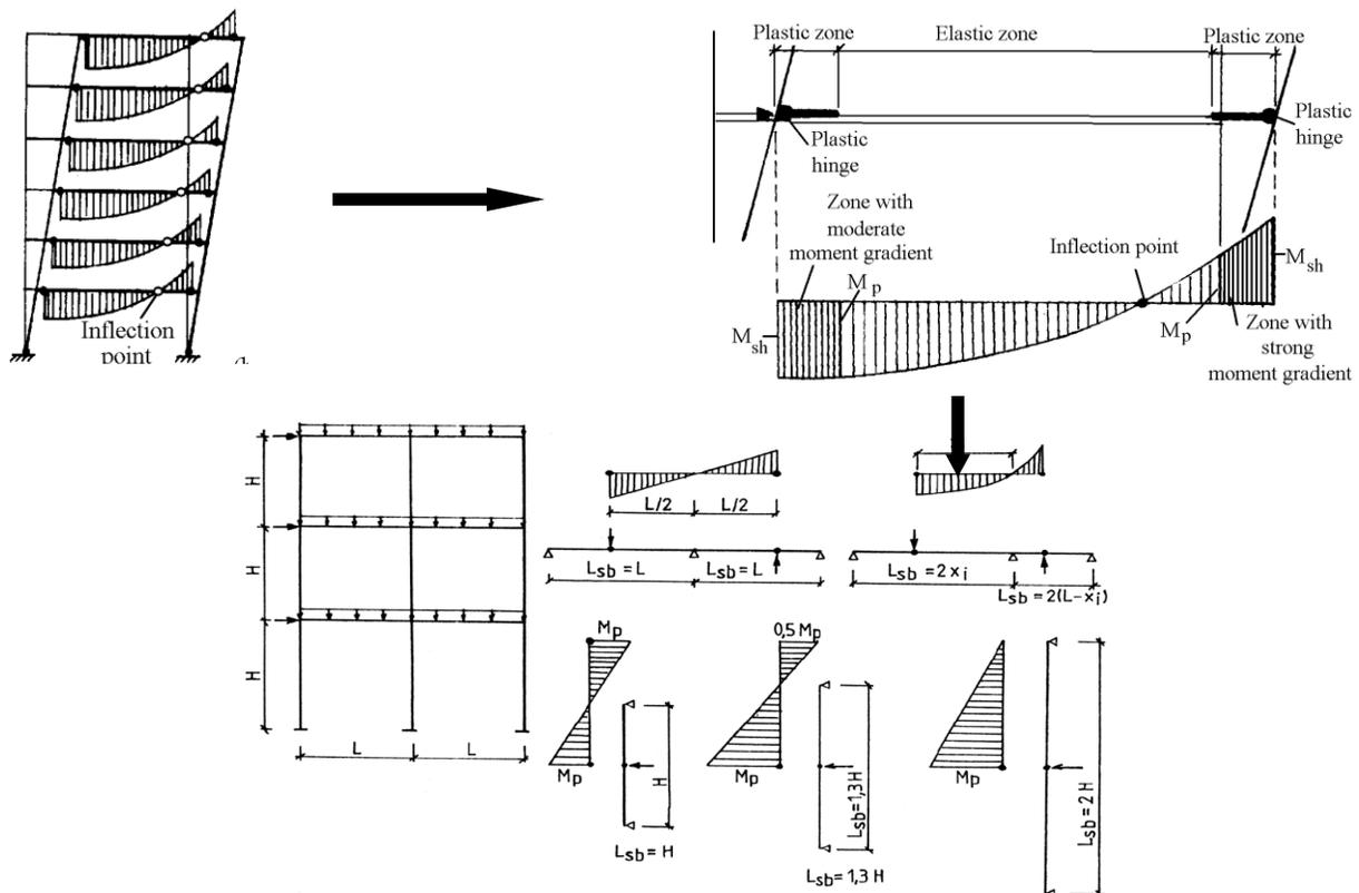
Fig. 3.2 The standard beam concept introducing the frame effect
