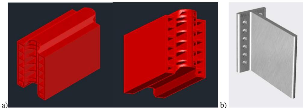
**Fig. 2.56** a) Prototype masonry block; b) T-shaped connector
