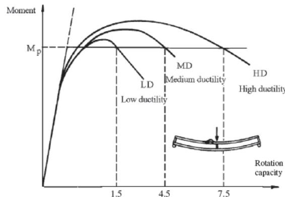
**Fig. 3.23** Member ductility classes based on moment-rotation curve
