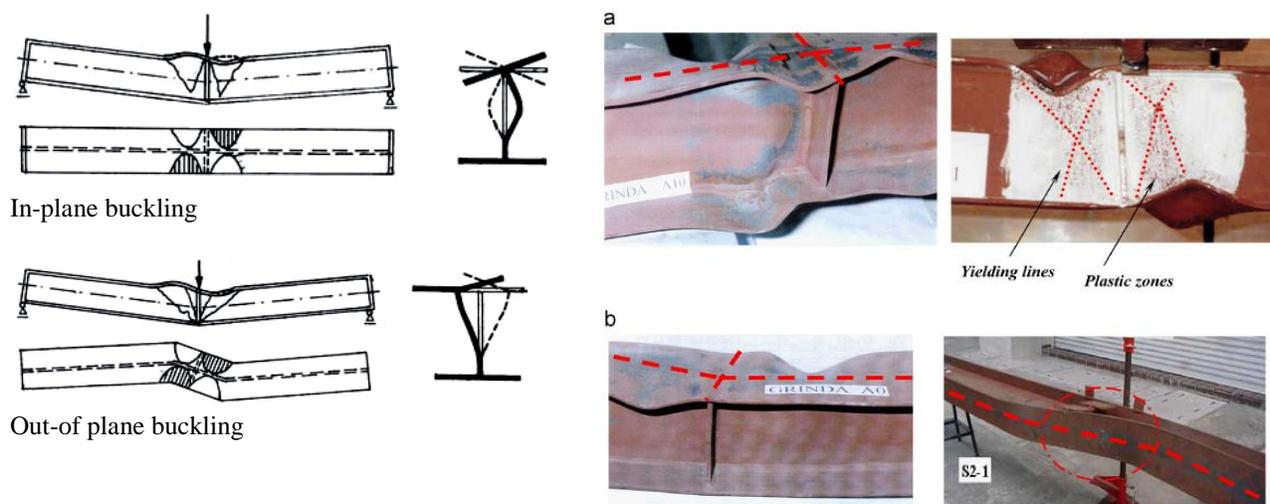
**Fig. 3.1** Plastic buckling types for standard beam SB 1: a) In-plane buckling, b) Out-of-plane buckling
