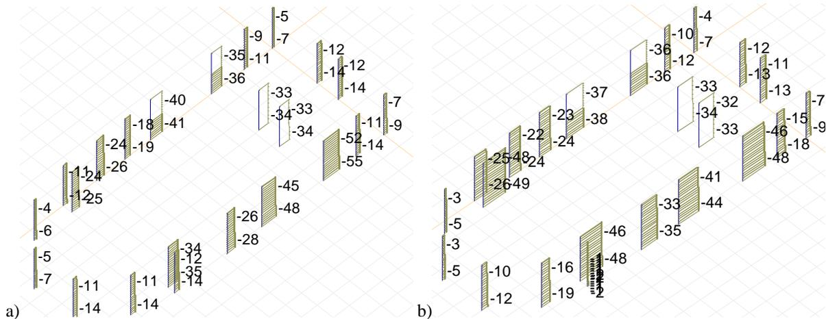
**Fig. 6.17** Maximum values of axial forces N in columns: a) before and b) after consolidation
