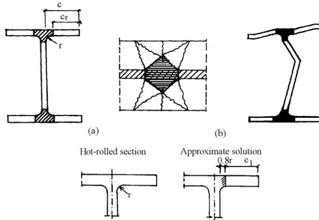
**Fig. 3.8** Plastic collapse mechanism for hot-rolled sections
