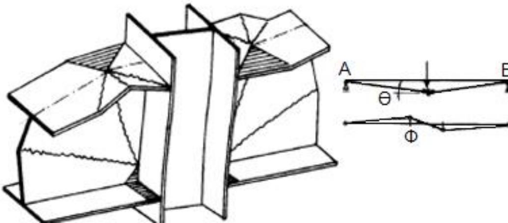
Fig. 3.4 Out of plane plastic mechanism
