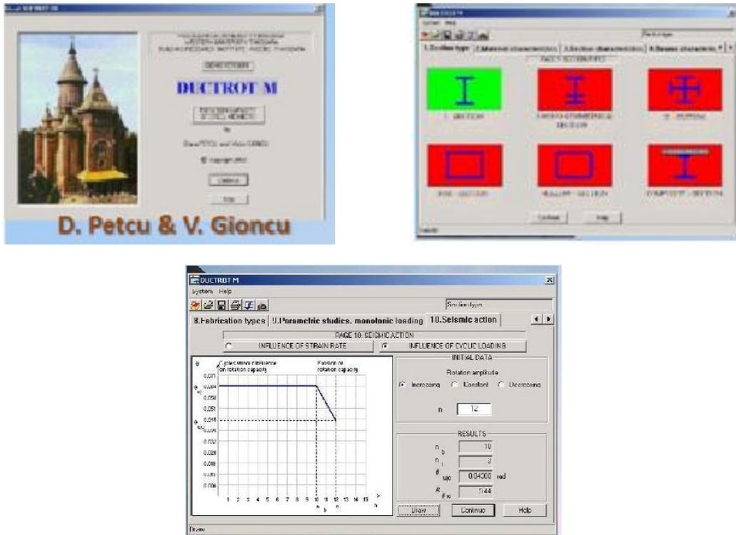
Fig. 3.30 DuctRot-M. Prediction of the local ductility under cyclic loading
