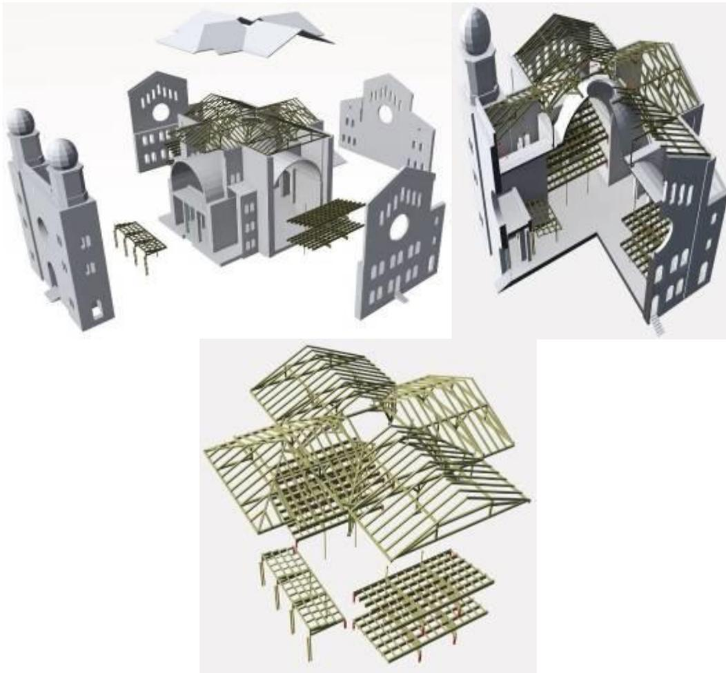
**Fig. 6.24** Arrangement of the load-bearing masonry walls and of the wooden elements at Timisoara Synagogue
