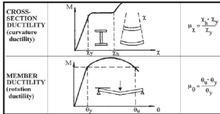
Fig. 3.21 Ductility types: cross-section ductility, member ductility
