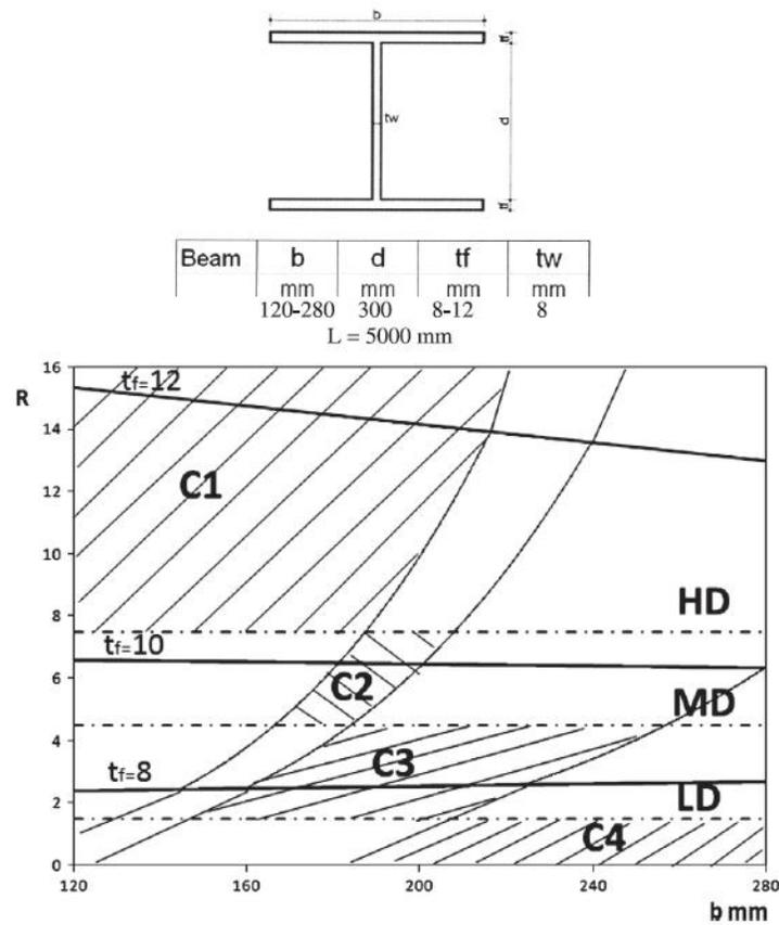
**Fig. 3.24** Member ductility vs. cross section ductility for a profile with C1 class for the web
