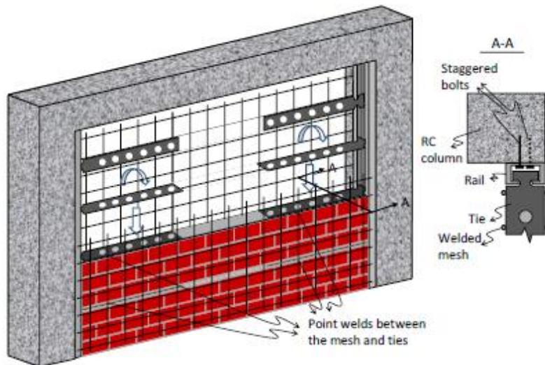
**Fig. 2.55** Solutions with special vertical joints and internal tie mesh system
