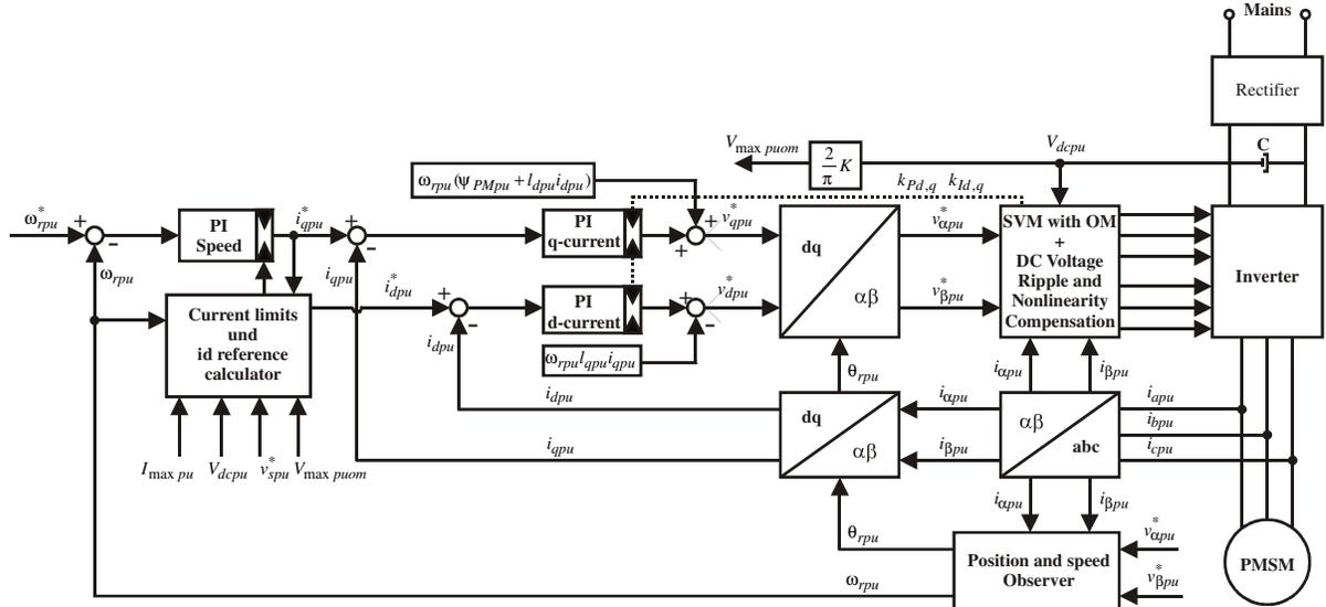
**Fig. 2.38.** Block diagram of the proposed rotor field oriented control.
