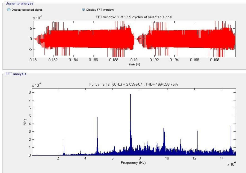
**Fig. 2.122.** FFT current between C and ground within 1 to 150kHz range for the Bridgeless IL topology.
