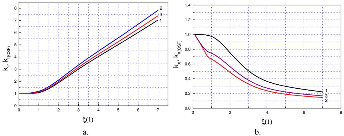
**Fig. 2.1.** Variation of the equivalent global changing factors of the rotoric parameters with the with the  $\xi_{(1)}$  for rectangular high slots: a.  $k_{r(CSF)}$  factor versus  $k_r$ ; b.  $k_{x(CSF)}$  factor versus  $k_x$ .
