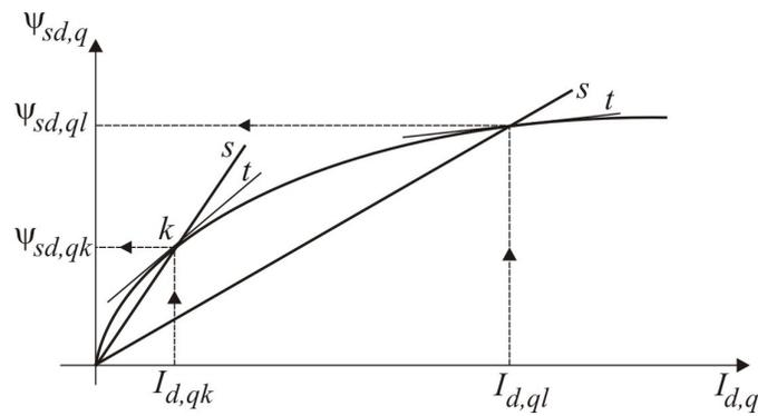
**Fig. 2.4.** Nonlinearity of  $d$ - and  $q$ -axis inductances.
