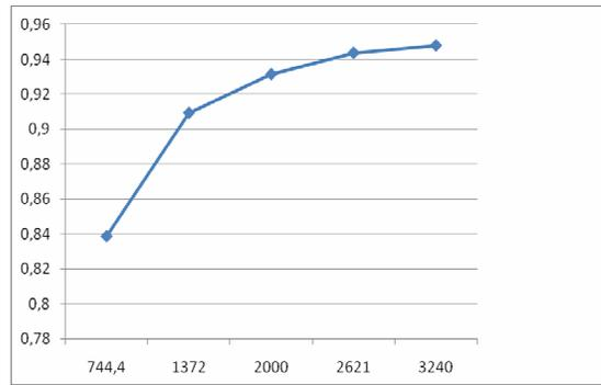
**Fig. 2.86.** Efficiency versus power curve for the Bridgeless topology.
