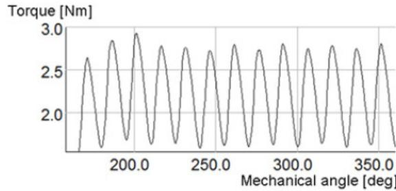
**Fig. 2.20.** Torque variation at 5.0 [A].
