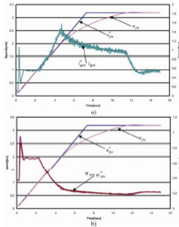
**Fig. 2. 58.** Acceleration performance showing, at 0.06 pu accelerating gradient: a) the speed ( $n_{pu}^*$ ,  $n_{pu}$ ),  $q$ -axis stator current ( $i_{apu}^*$ ,  $i_{apu}$ ); b) the speed ( $n_{pu}^*$ ,  $n_{pu}$ ), the stator flux ( $\Psi_{apu}^*$ ,  $\Psi_{apu}$ ).
