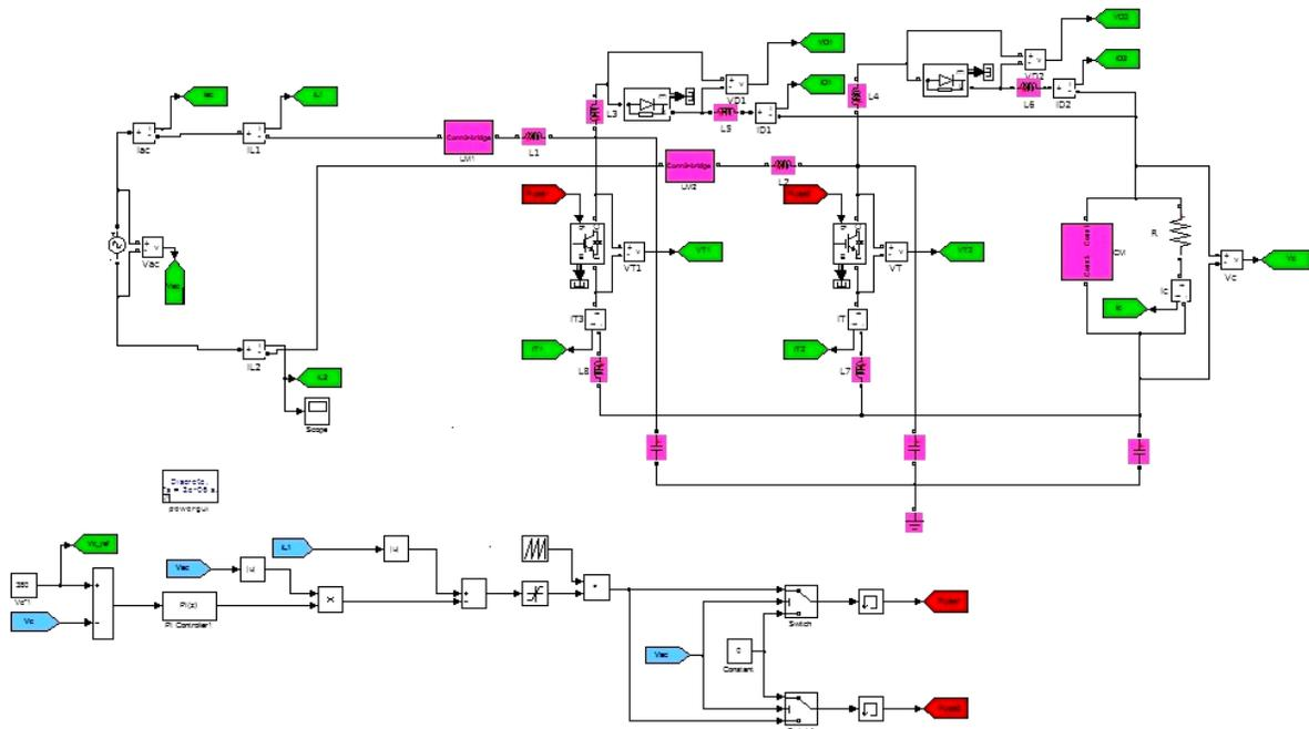
Fig. 2.65. Bridgeless PFC converter model implementation in Matlab/Simulink.
