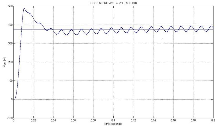
**Fig. 2.102.** Voltage output for the Boost IL topology.
