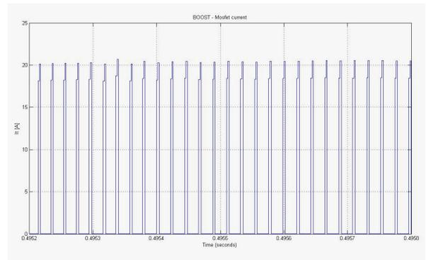
**Fig. 2.71.** Zoom on Mosfet current for the Boost topology.
