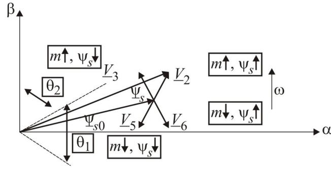
**Fig. 2.27.** Selection of the optimum voltage vector and the effects on the evolution of the electromagnetic torque and stator flux.
