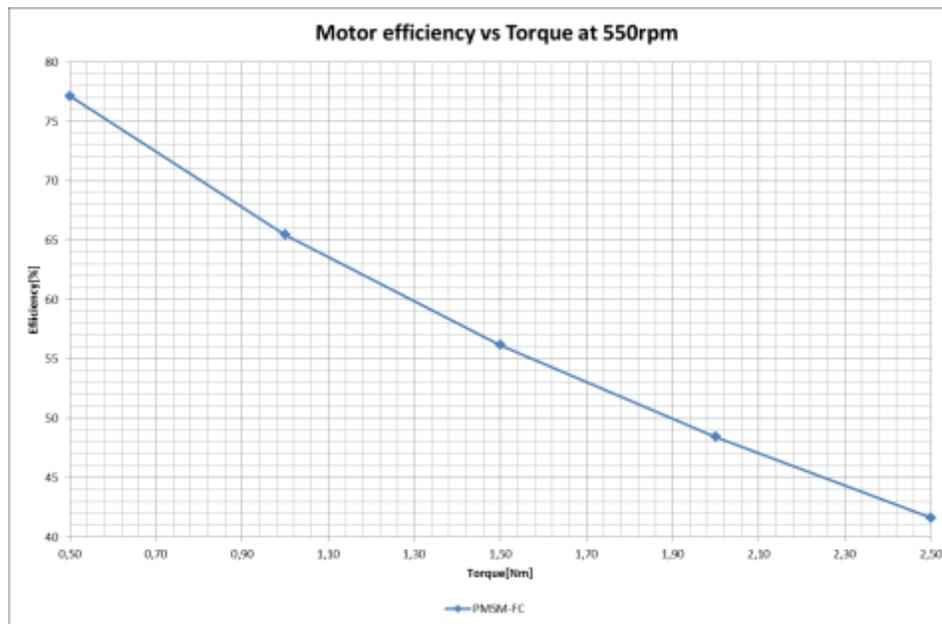
Fig. 2.23. Measured motor performance – Motor efficiency vs. torque.
