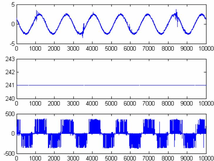
**Fig. 2.32.** The normal functioning regime at 20 % of the prescribed speed: phase current, speed, voltage.
