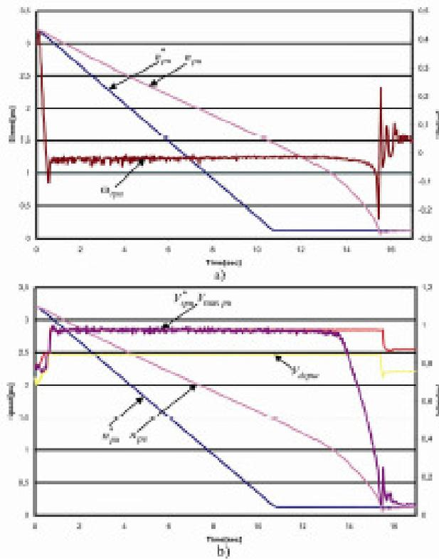
**Fig. 2.61.** Decelerating performance showing, at 0.04 pu accelerating gradient: a) the speed ( $n_{pu}^*$ ,  $n_{pu}$ ), rotor angular frequency ( $\omega_{rpu}$ ); b) the speed ( $n_{pu}^*$ ,  $n_{pu}$ ), the regulated stator voltage ( $V_{spu}^*$ ), the maximum terminal voltage ( $V_{max\ pu}$ ) and the dc link voltage ( $V_{dc\ pu}$ ).
