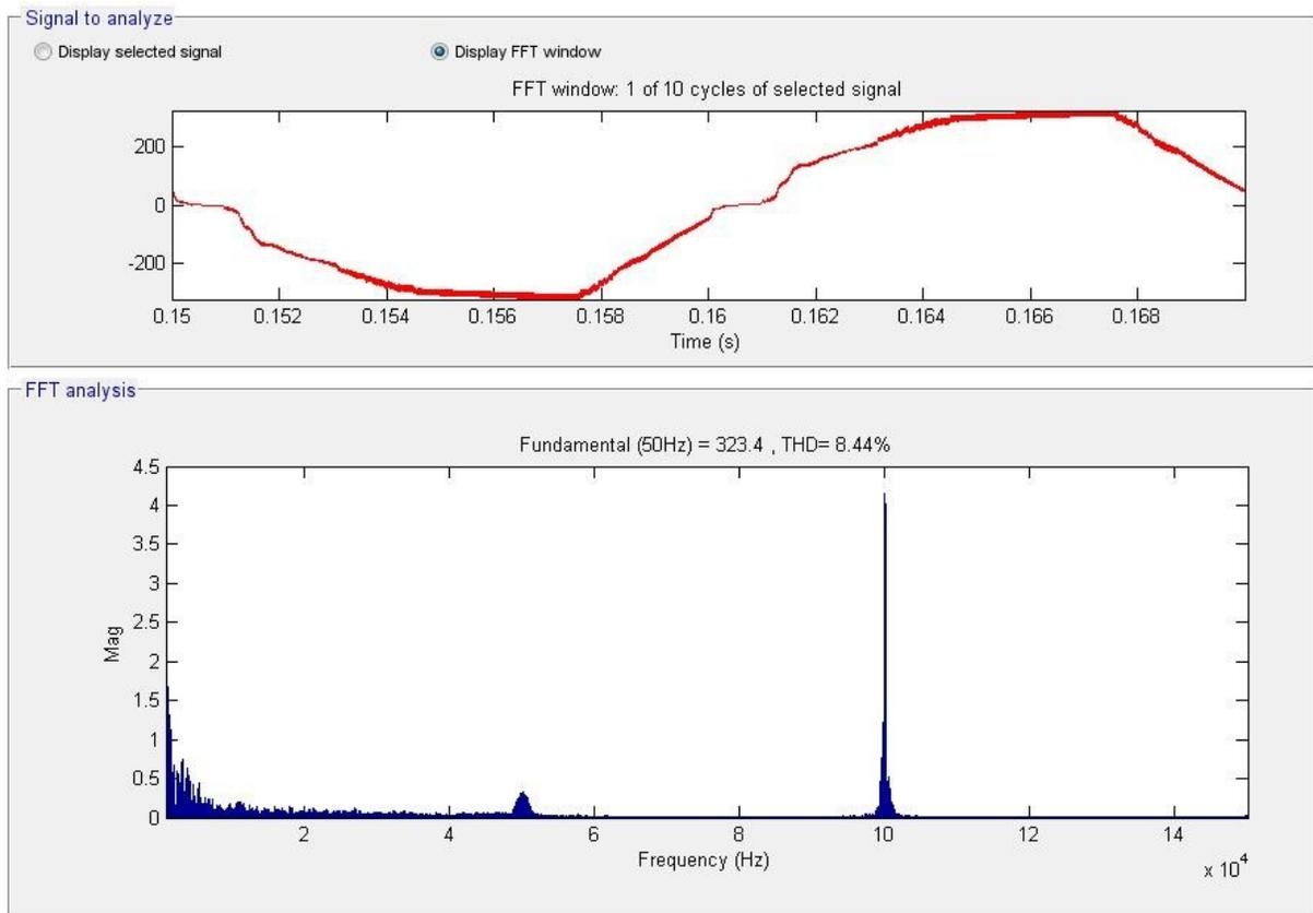
**Fig. 2.107.** FFT for voltage measured after EMI filter within 1 to 150kHz range for the Boost IL topology.
