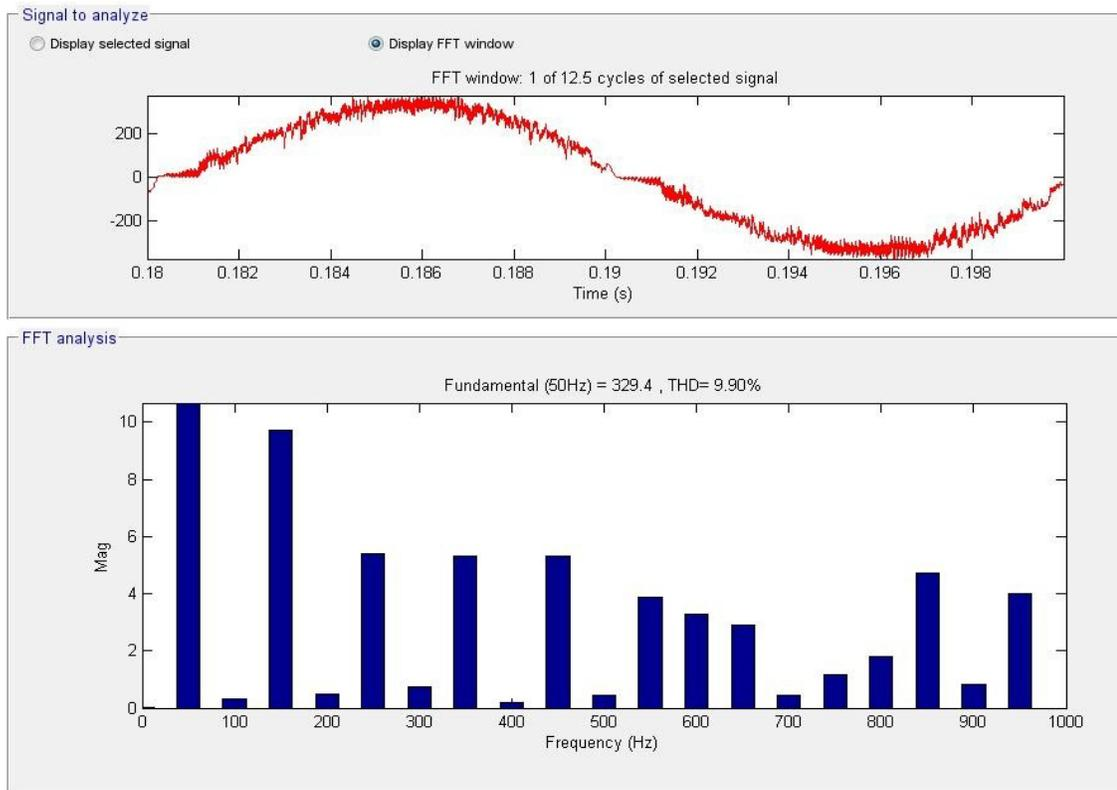
**Fig. 2.89.** FFT for voltage measured after EMI filter within 0 to 1kHz range for the Bridgeless topology.
