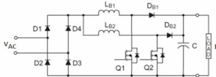
**Fig. 2.93.** Boost IL PFC converter topology.
