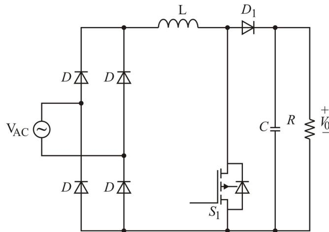
Fig. 2.62. Boost PFC converter topology.
