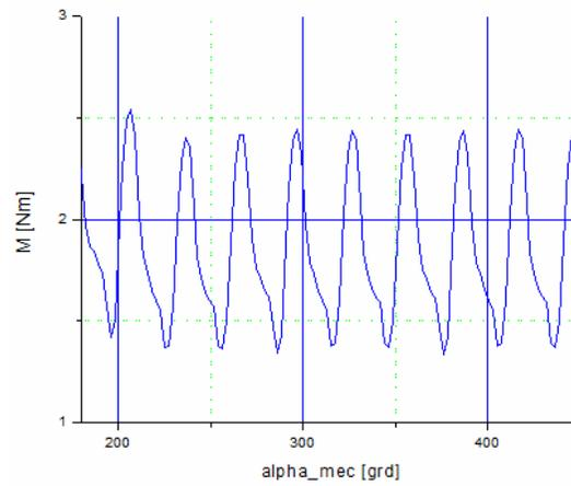
Fig. 2.15. Torque variation at 3.45 [A].
