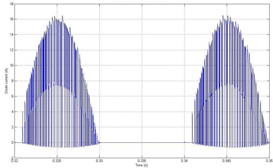
**Fig. 2.83.** Zoom on diode current for the Bridgeless topology.
