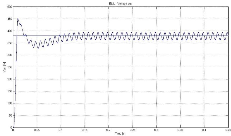
**Fig. 2.115.** Voltage output for the Bridgeless IL topology.
