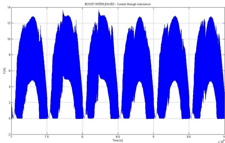
**Fig. 2.98.** Zoom on inductance current for the Boost IL topology.
