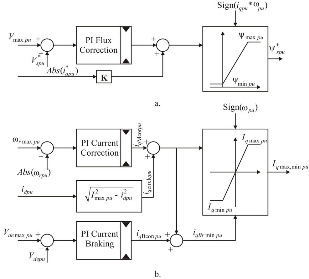
**Fig. 2. 57.** a) Block diagram of proposed “Flux reference calculator”;
