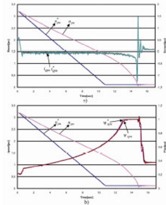
**Fig. 2.60.** Decelerating performance showing, at 0.06pu accelerating gradient: a) the speed ( $n_{pu}^*$ ,  $n_{pu}$ ),  $q$ -axis stator current ( $i_{apu}^*$ ,  $i_{apu}$ ); b) the speed ( $n_{pu}^*$ ,  $n_{pu}$ ), the stator flux ( $\Psi_{spu}^*$ ,  $\Psi_{spu}$ ).
