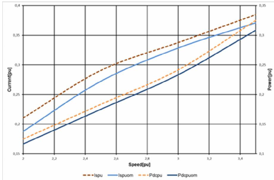
**Fig. 2.44.** Overmodulation benefits in steady-state showing motor current ( $i_{spuom}$ ,  $i_{spu}$ ), and dc link power ( $P_{dcpuom}$ ,  $P_{dcpu}$ ) with or without overmodulation versus motor speed.
