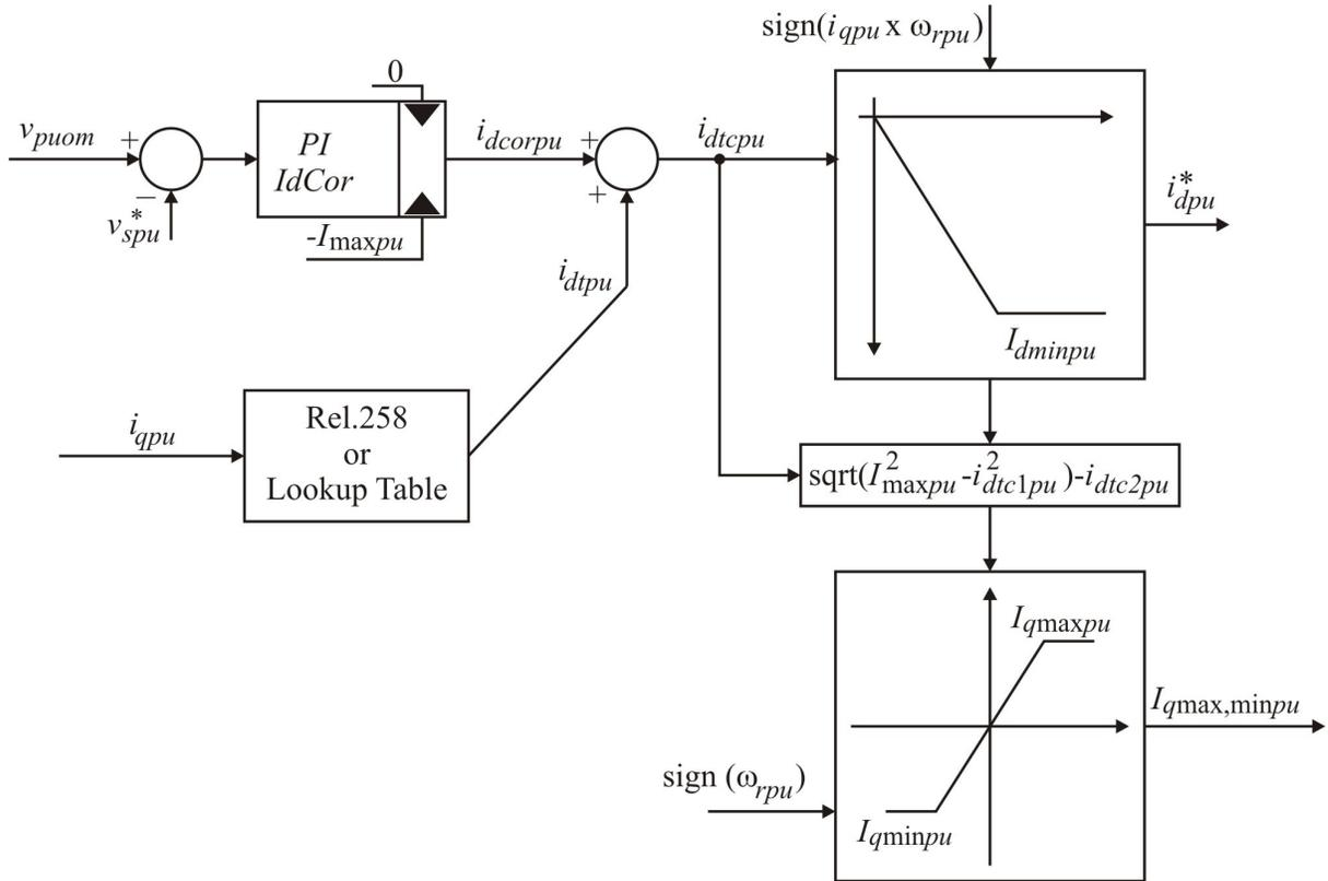
**Fig. 2.39.** Block diagram of the proposed algorithm.
