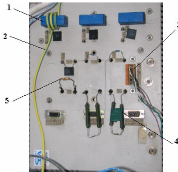
**Fig. 2.29.** The signal conversion plate received from inverter 1, MEL, current transducer; 2-phase used for current acquisition at the inverter output; 3 - the output used for voltage acquisition; 4- resistance of 44 [kΩ] corresponding to the motor voltage; 5-resistance of 1.8 [kΩ] corresponding to speed signal.
