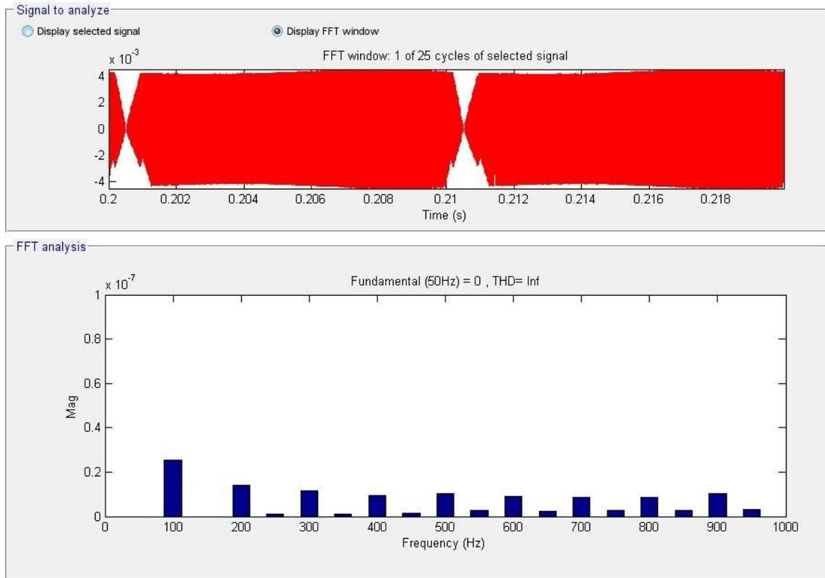
**Fig. 2.91.** FFT current between C and ground within 0 to 1kHz range for the Bridgeless topology.
