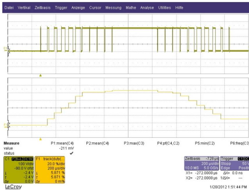
Fig. 2.45. Carrier-based pulse width-modulated voltage with overmodulation.
