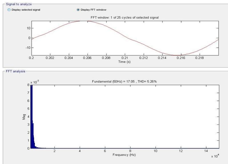
**Fig. 2.88.** FFT for input current range from 1 to 150kHz for Bridgeless topology.
