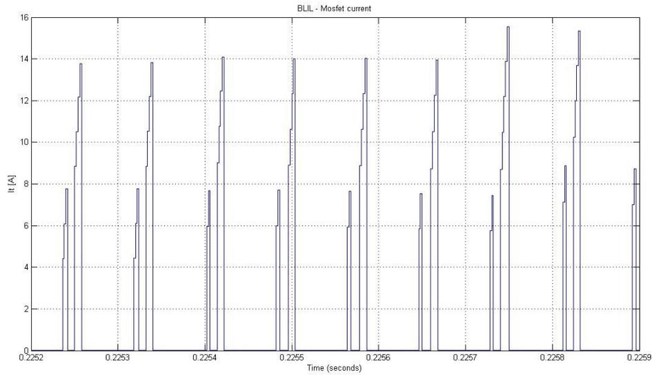
**Fig. 2.114.** Zoom on Mosfet current for the Bridgeless IL topology.
