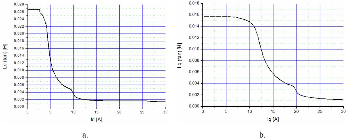
**Fig. 2.14.** The a.  $L_d$  and b.  $L_q$  inductivities curves vs. current for version 2V.
