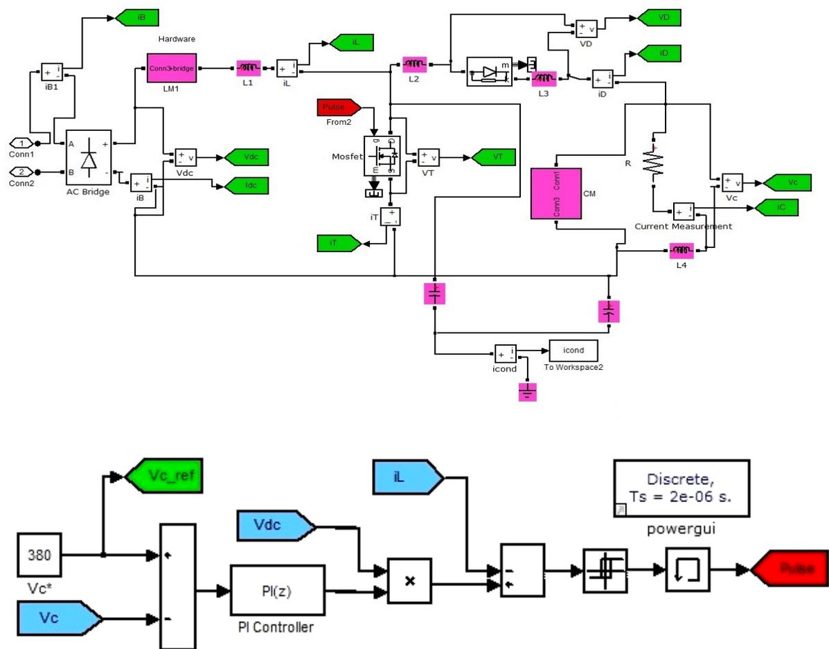
Fig. 2.63. Boost PFC converter model implementation in Matlab/Simulink.
