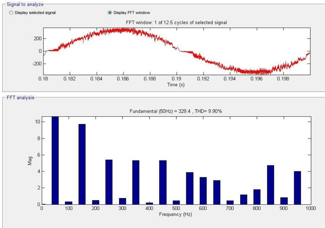
**Fig. 2.119.** FFT for voltage measured after EMI filter within 0 to 1kHz range for the Bridgeless IL topology.
