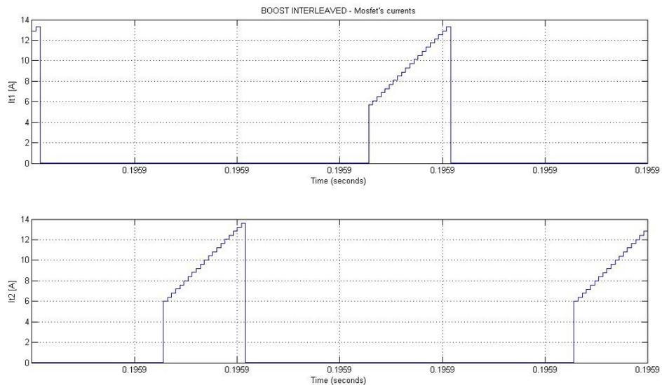
Fig. 2.101. Zoom on Mosfet currents for the Boost IL topology.
