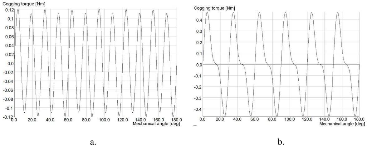
**Fig. 2.13.** Cogging torque 2V; b. 2VU.
