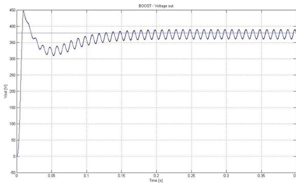
**Fig. 2.72.** Voltage output for the Boost topology
