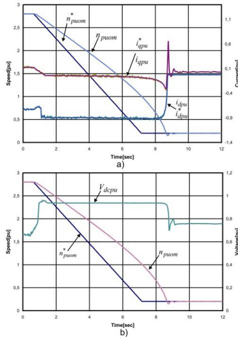
**Fig. 2.42.** Braking performances showing the speed ( $n_{puom}^*$ ,  $n_{puom}$ ),  $d$ -axis current ( $i_{dpu}^*$ ,  $i_{dpu}$ ) and  $q$ -axis current ( $i_{qpu}^*$ ,  $i_{qpu}$ ) gradient 0.2 pu a), b) the speed ( $n_{puom}^*$ ,  $n_{puom}$ ), regulated dc link voltage ( $V_{dc\ pu}$ ) braking gradient 0.02 pu.
