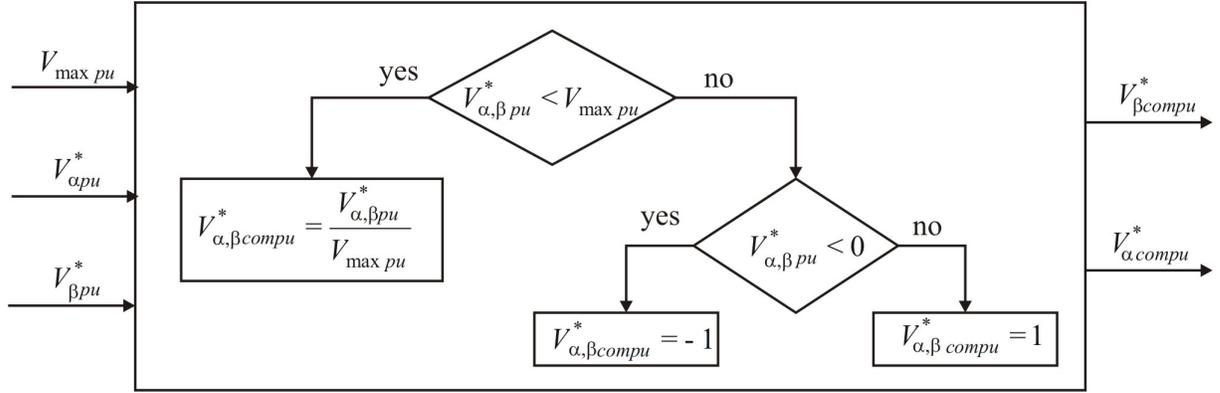
**Fig. 2.49.** DC-link voltage ripple compensation.
