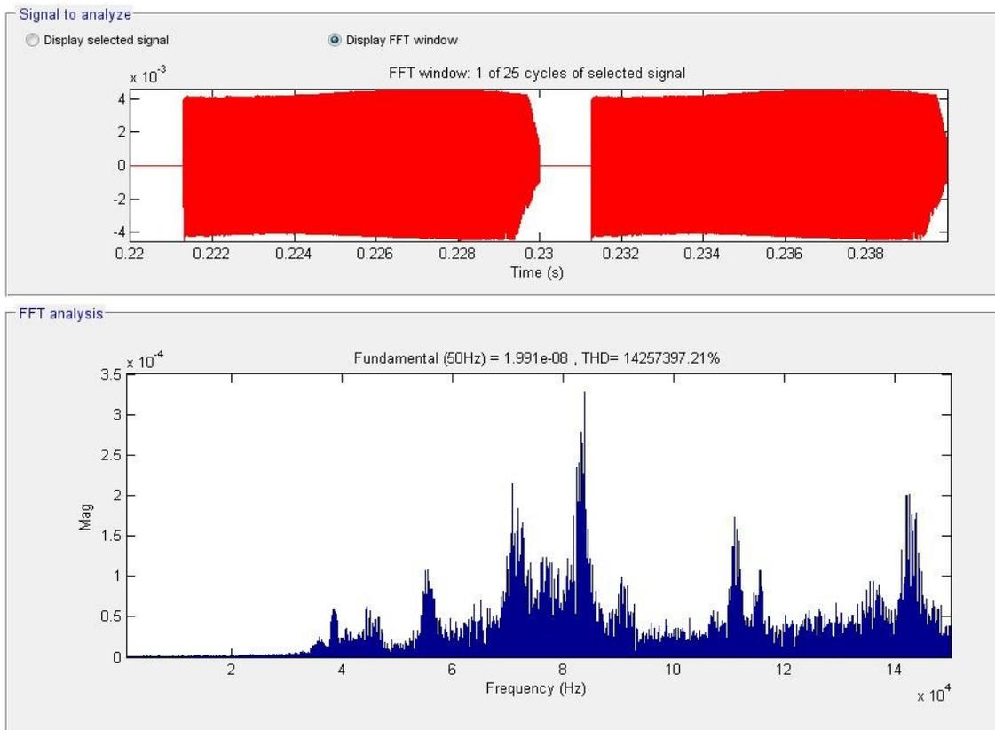
Fig. 2.79. FFT current between C and ground within 1 to 150kHz range for the Boost topology.
