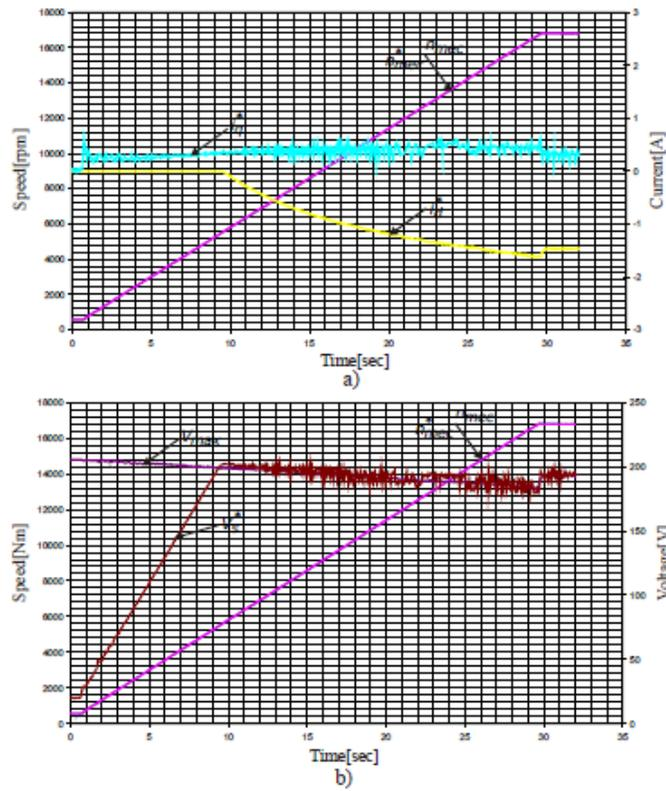
Fig. 2.53. Accelerating performance of the proposed speed regulation drive system of MSMPS.
