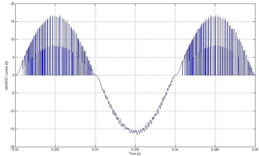
**Fig. 2.84.** Zoom on Mosfet current for the Bridgeless topology.
