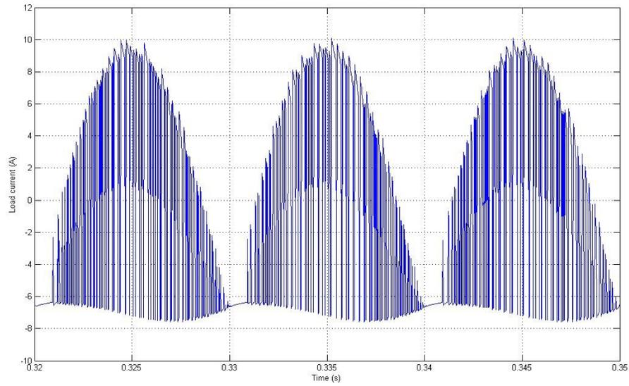
**Fig. 2.82.** Zoom on capacitor current for the Bridgeless topology.
