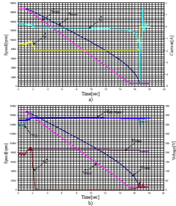
**Fig. 2.55.** Decelerating performance of the proposed speed regulation drive system of MSMPS.
