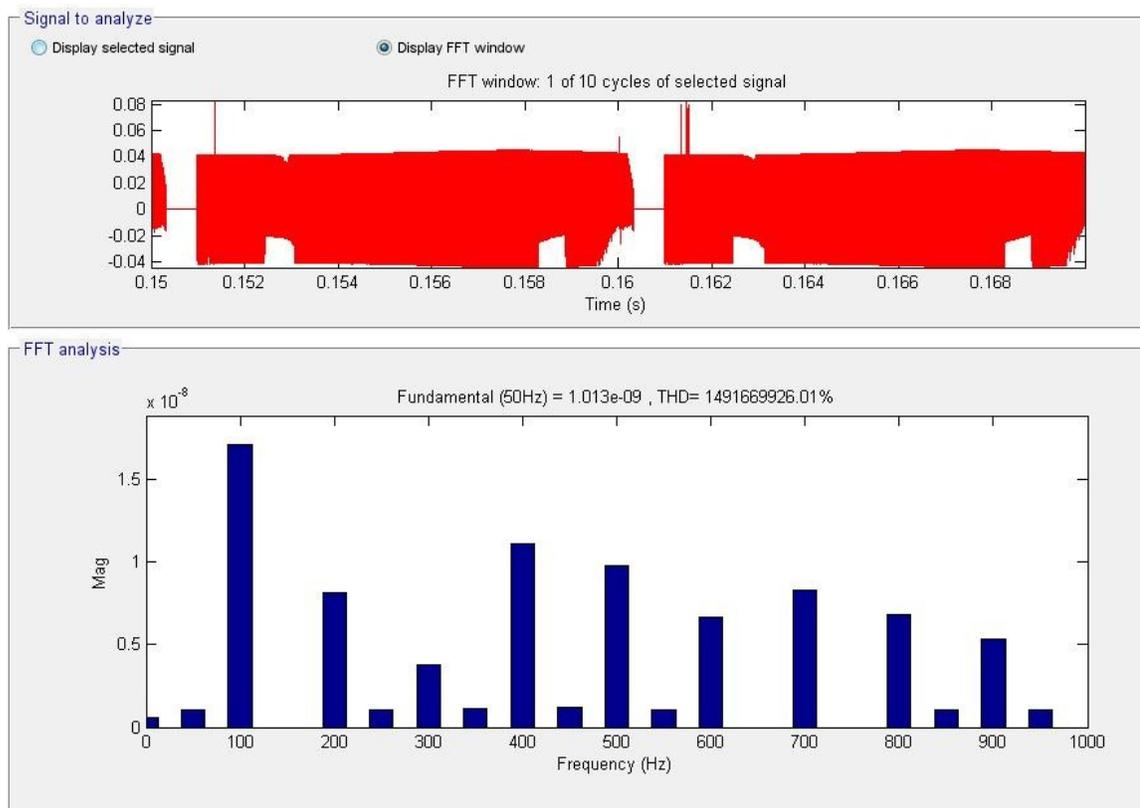
**Fig. 2.108.** FFT current between C and ground within 0 to 1kHz range for the Boost IL topology.
