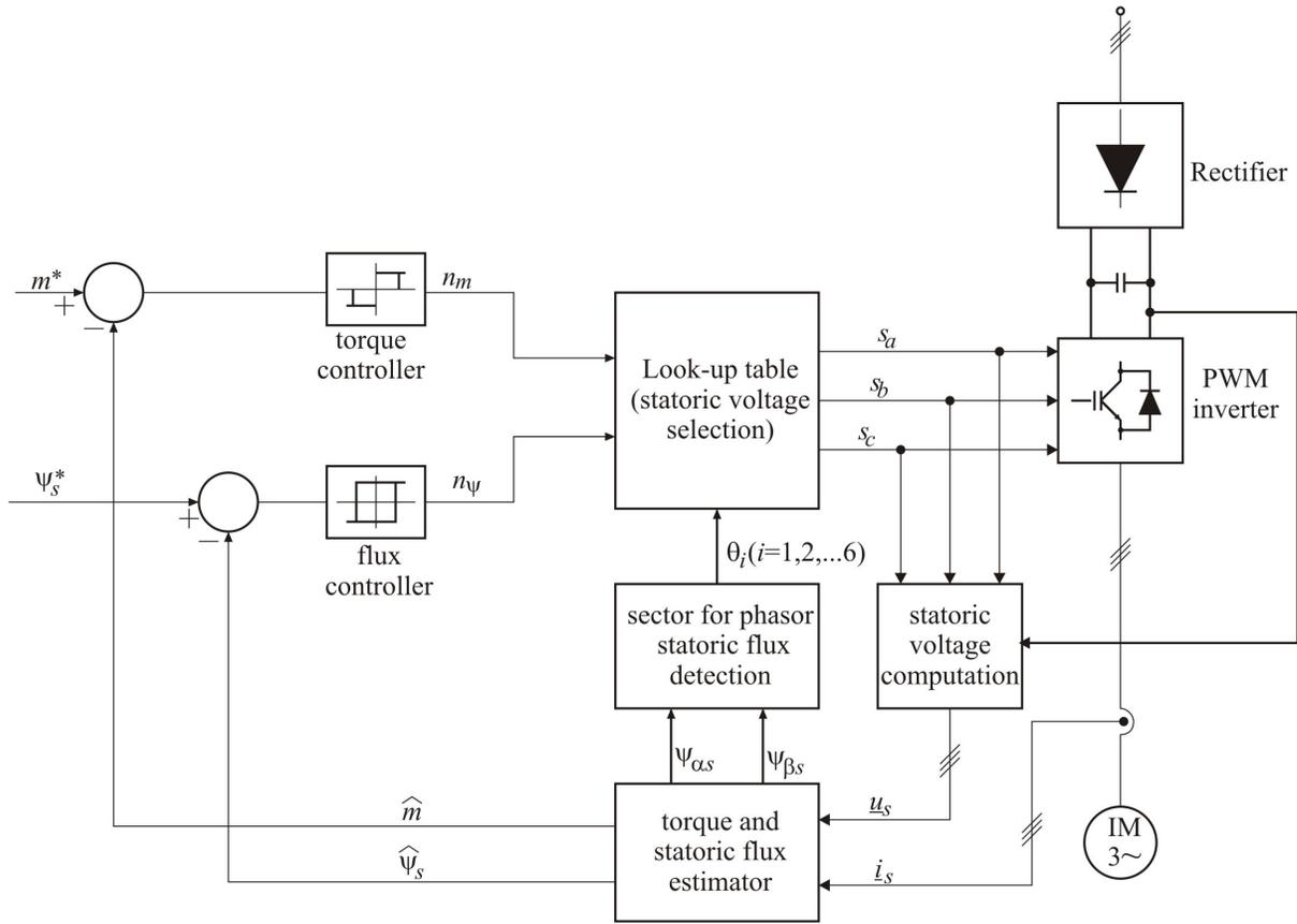
**Fig. 2.24.** Classic DTC stator-flux-oriented induction motor fed by a PWM voltage inverter
