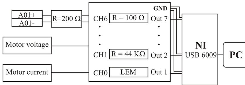
**Fig. 2.28.** The block diagram of the data acquisition system.
