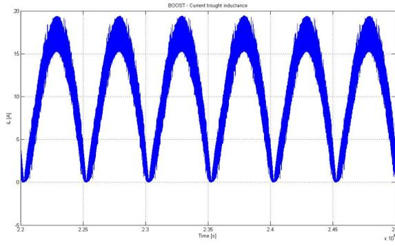
**Fig. 2.68.** Zoom on inductance current for the Boost topology.
