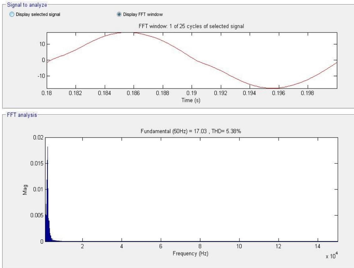
**Fig. 2.118.** FFT for input current range from 1 to 150kHz for Bridgeless IL topology.
