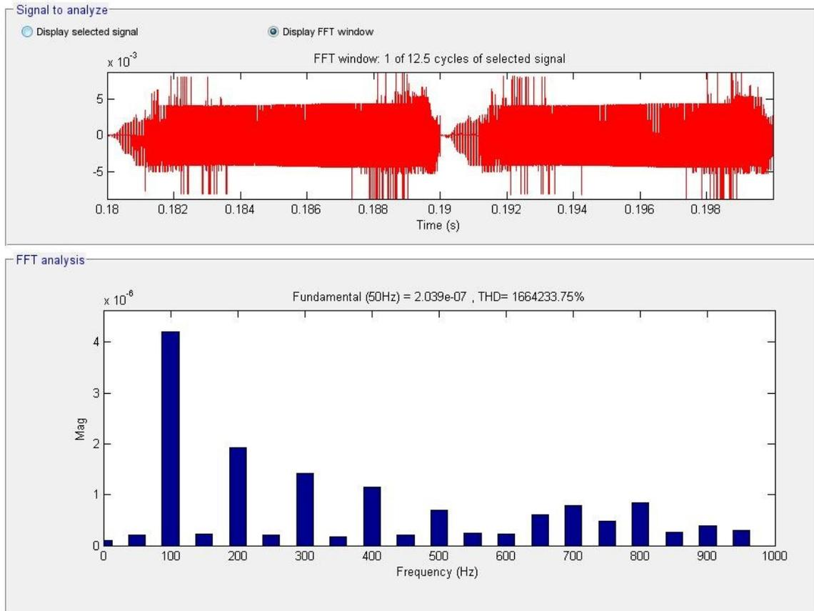
**Fig. 2.121.** FFT current between C and ground within 0 to 1kHz range for the Bridgeless IL topology.
