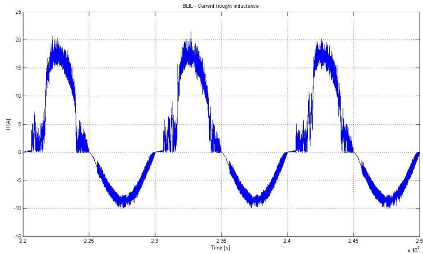
**Fig. 2.111.** Zoom on inductance current for the Bridgeless IL topology.
