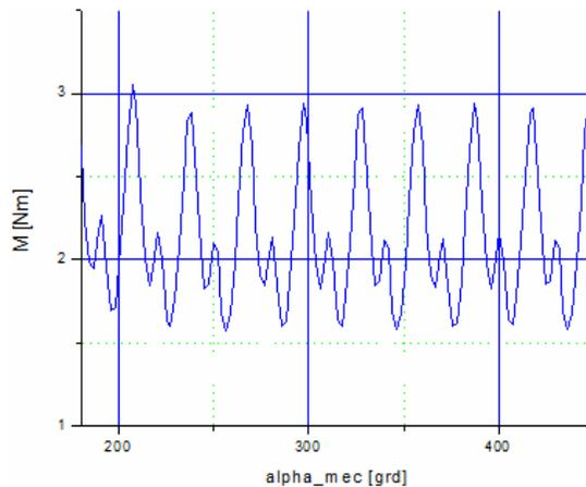
Fig. 2.10. Torque variation at 5 [A].
