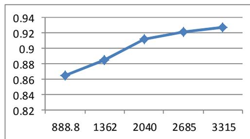
**Fig. 2.103.** Efficiency versus power curve for the Boost IL topology.
