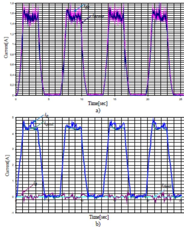
Fig. 2.52. Current estimation performance in the constant-torque region.
