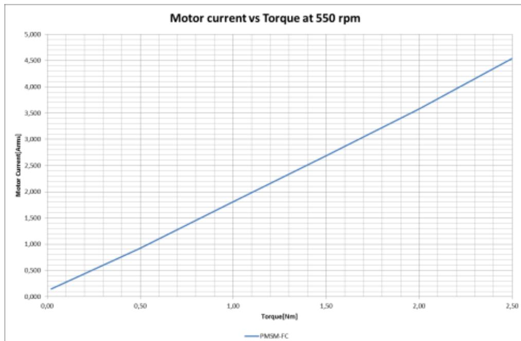
**Fig. 2.22.** Measured motor performance – Motor current vs. torque.
