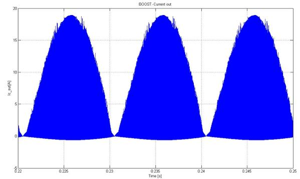
**Fig. 2.69.** Zoom on capacitor current for the Boost topology.
