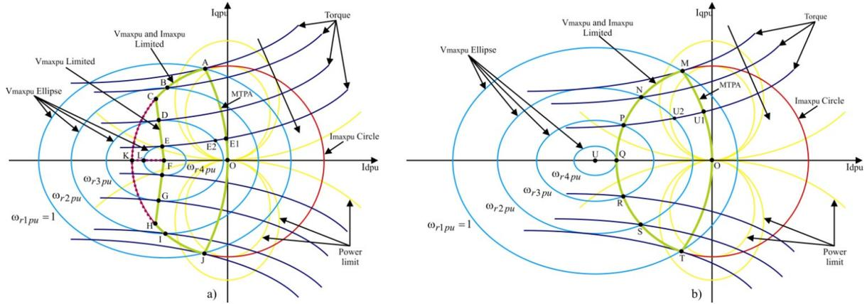
**Fig. 2.37.** Cycle diagrams of PMSM drive.
