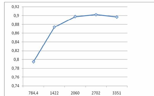
**Fig. 2.73.** Efficiency versus power curve for the Boost topology.
