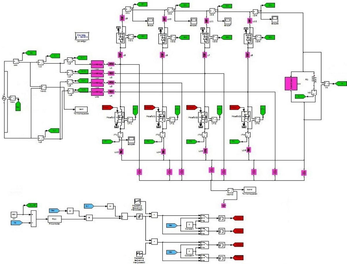
Fig. 2.96. Bridgeless IL PFC converter model implementation in Matlab/Simulink
