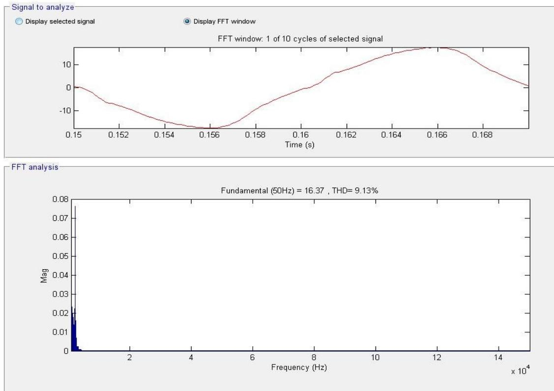
**Fig. 2.105.** FFT for input current range from 1 to 150 [kHz] for Boost IL topology.
