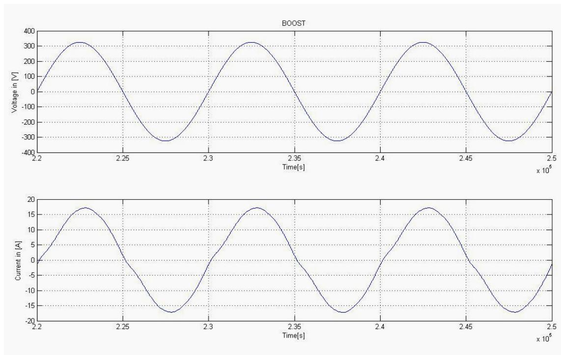
**Fig. 2.67.** Zoom on input voltage & input current for the Boost topology.
