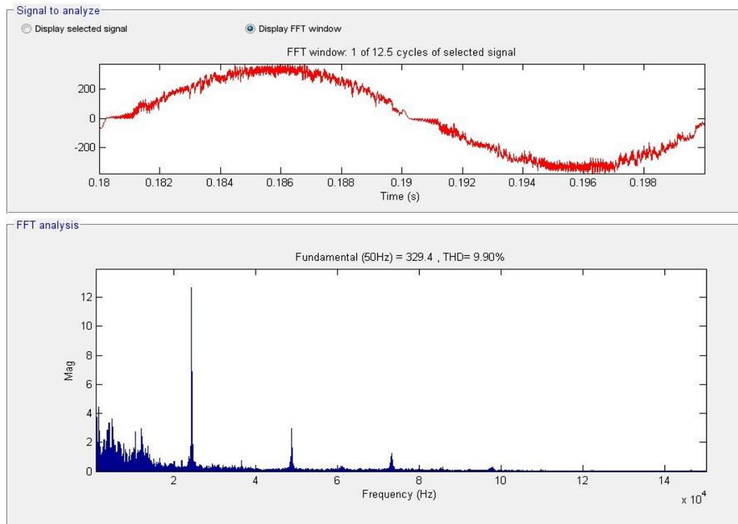
**Fig. 2.120.** FFT for voltage measured after EMI filter within 1 to 150kHz range for the Bridgeless IL topology.
