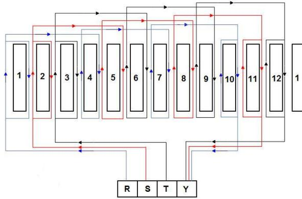
**Fig. 2.3.** The machine stator winding scheme.
