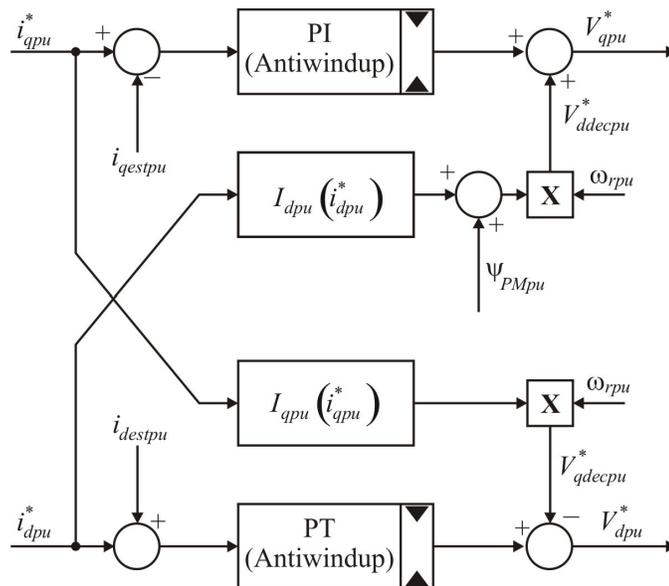
Fig. 2.48. Voltage reference calculator block in the rotor reference frame
