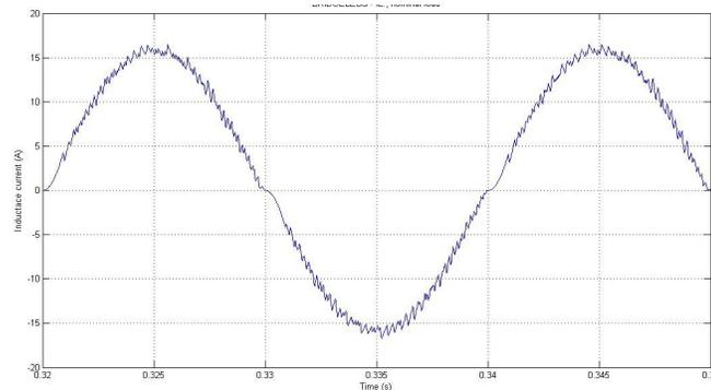
**Fig. 2.81.** Zoom on inductance current for the Bridgeless topology.
