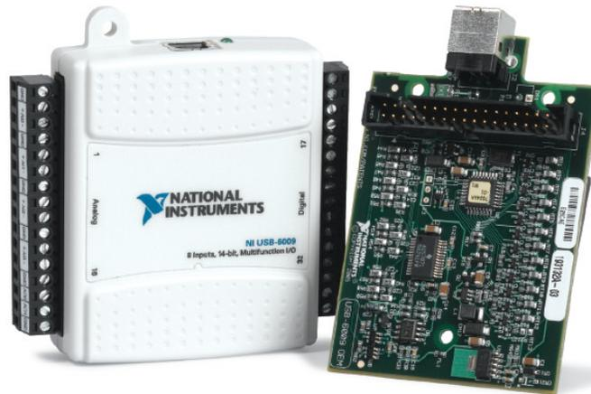
**Fig. 2.31.** National Instruments 6009 acquisition board.
