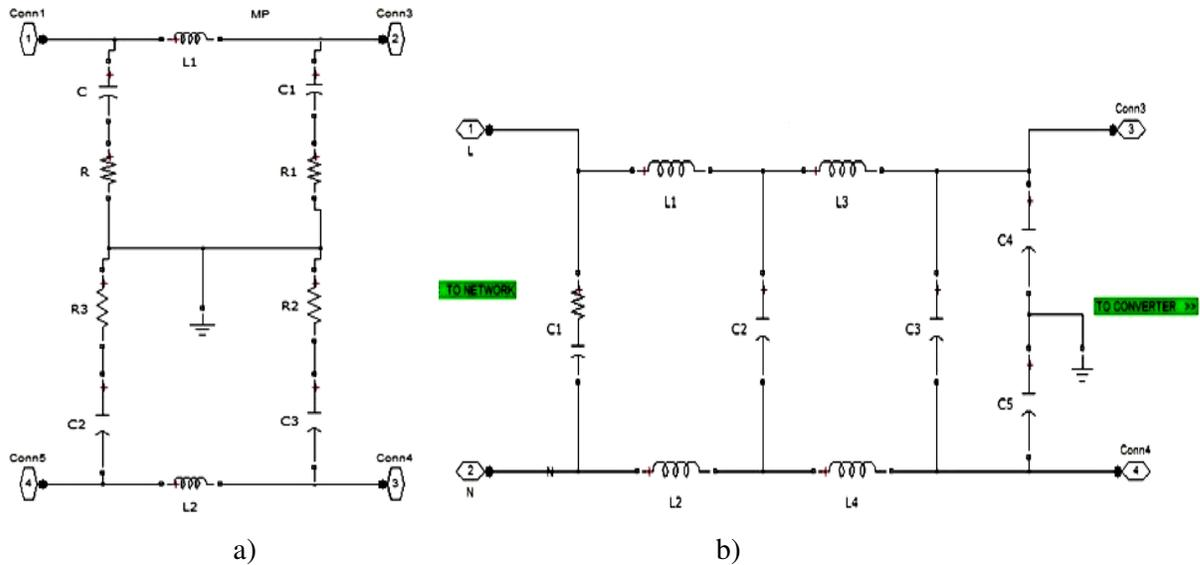
**Fig. 2.66.** Matlab/Simulink Implementation of the Common Mode (a) and EMI filters (b).
