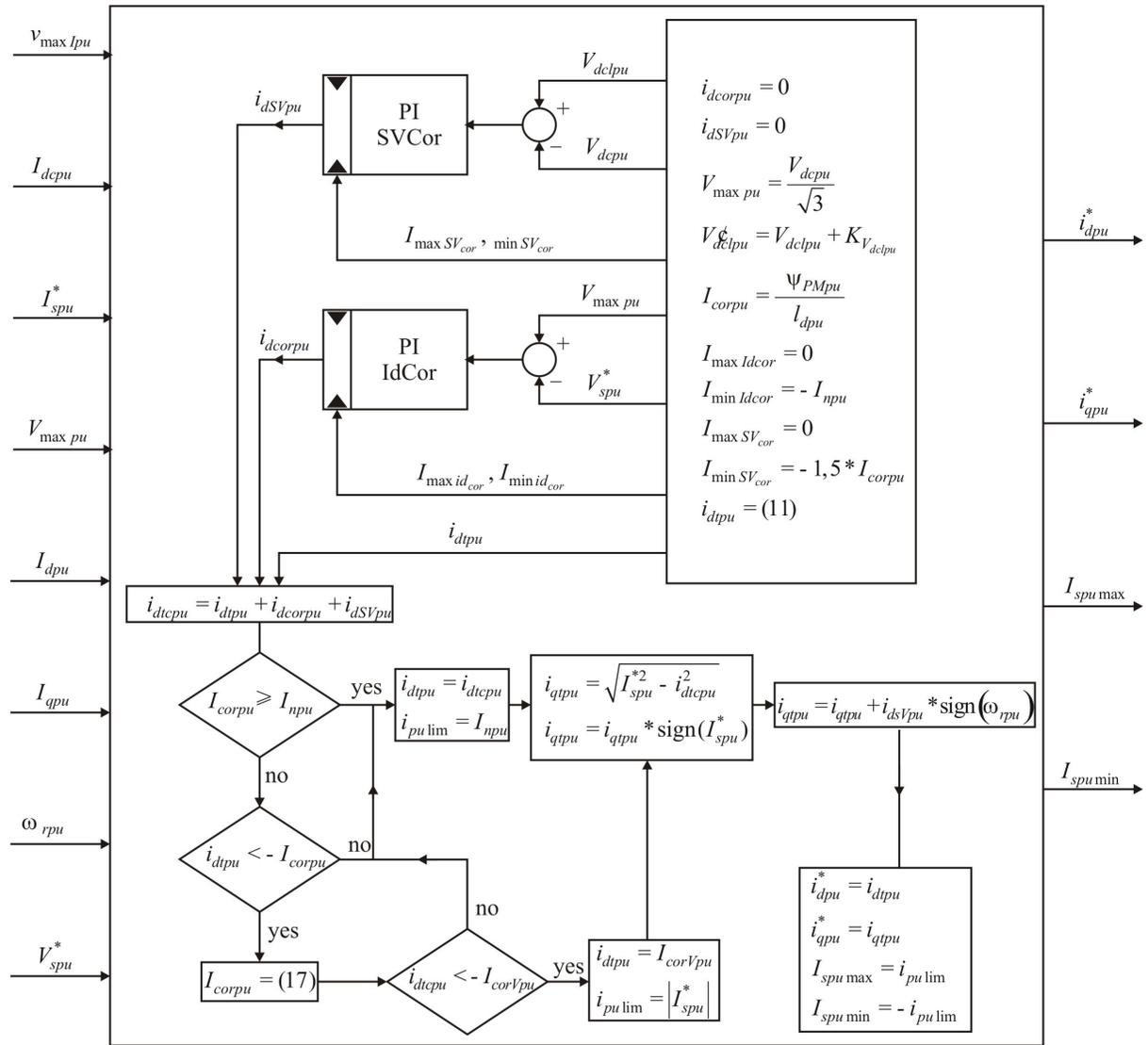
Fig. 2.47. Block diagram of the proposed current reference calculator.
