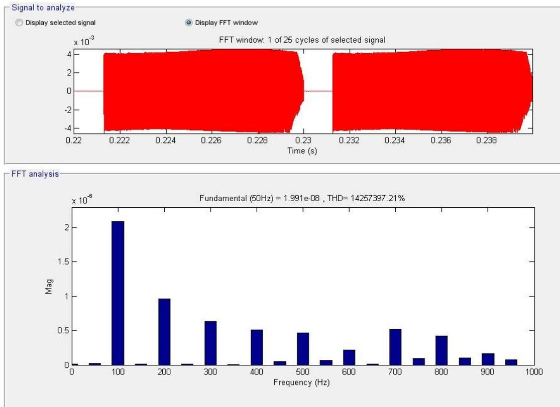
Fig. 2.78. FFT current between C and ground within 0 to 1kHz range for the Boost topology.
