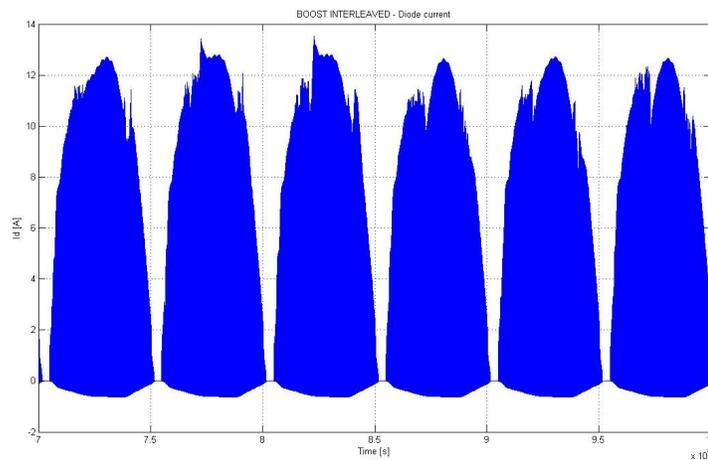
Fig. 2.100. Zoom on diode current for the Boost IL topology.
