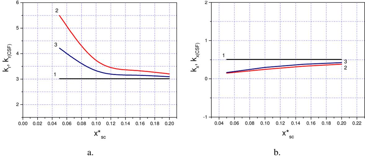
**Fig. 2.2.** Variation of the equivalent global changing factors of the rotoric parameters with the reported short-circuit reactance of the machine: a.  $k_{r(CSF)}$  factor versus  $k_r$ ; b.  $k_{x(CSF)}$  factor versus  $k_x$ .
