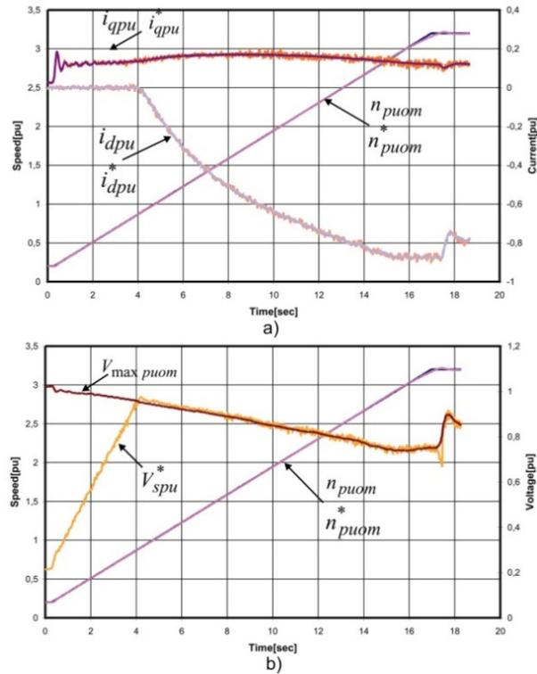
**Fig. 2.41.** Accelerating performance showing, at 0.03 pu accelerating gradient: a) the speed ( $n_{puom}^*$ ,  $n_{puom}$ ),  $d$ -axis current ( $i_{dpu}^*$ ,  $i_{dpu}$ ) and  $q$ -axis current ( $i_{qpu}^*$ ,  $i_{qpu}$ ), b) the speed ( $n_{puom}^*$ ,  $n_{puom}$ ), the regulated stator voltage ( $V_{spu}^*$ ) and the maximum terminal voltage ( $V_{max\ pu}$ ).
