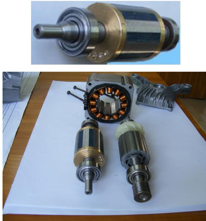
**Fig. 2.21.** PMSM with flux concentrator rotor PMSM-FC.
