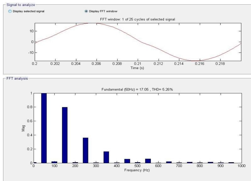
**Fig. 2.87.** FFT for input current range from 0 to 1kHz for Bridgeless topology
