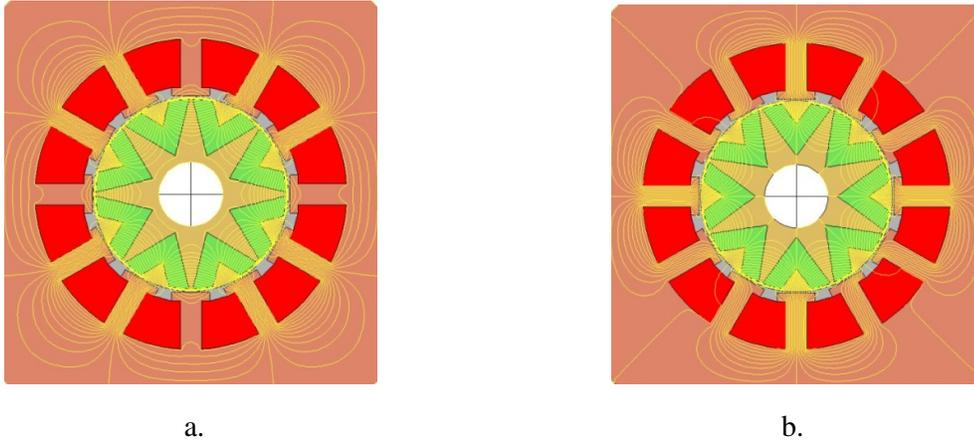
**Fig. 2.6.** One V flux barrier rotor geometry:  $d$ -axis PM flux plots,  $b$ .  $q$ -axis PM flux plots.
