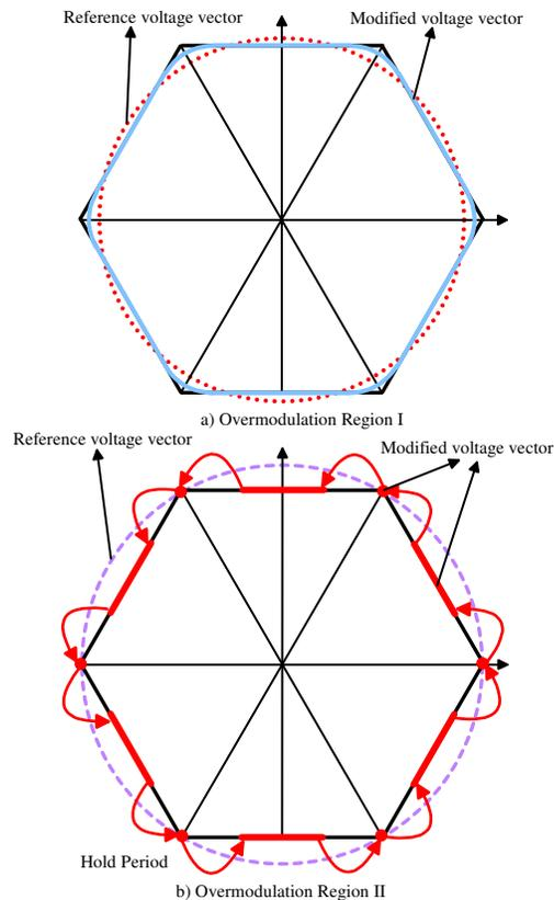
**Fig. 2.40.** Trajectory of voltage vector in:
