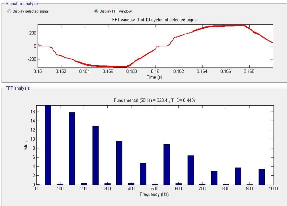
**Fig. 2.106.** FFT for voltage measured after EMI filter within 0 to 1 [kHz] range for the Boost IL topology.
