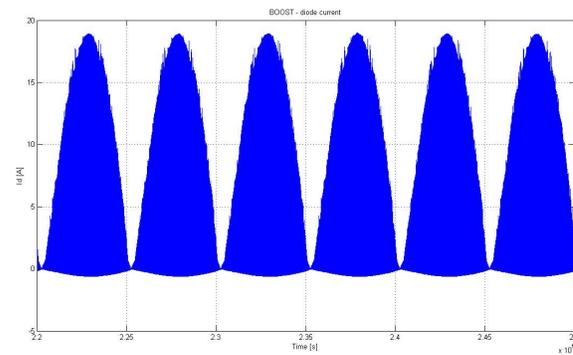
**Fig. 2.70.** Zoom on diode current for the Boost topology.
