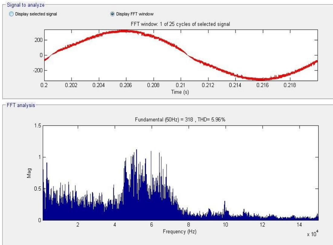
**Fig. 2.90.** FFT for voltage measured after EMI filter within 1 to 150kHz range for the Bridgeless topology.
