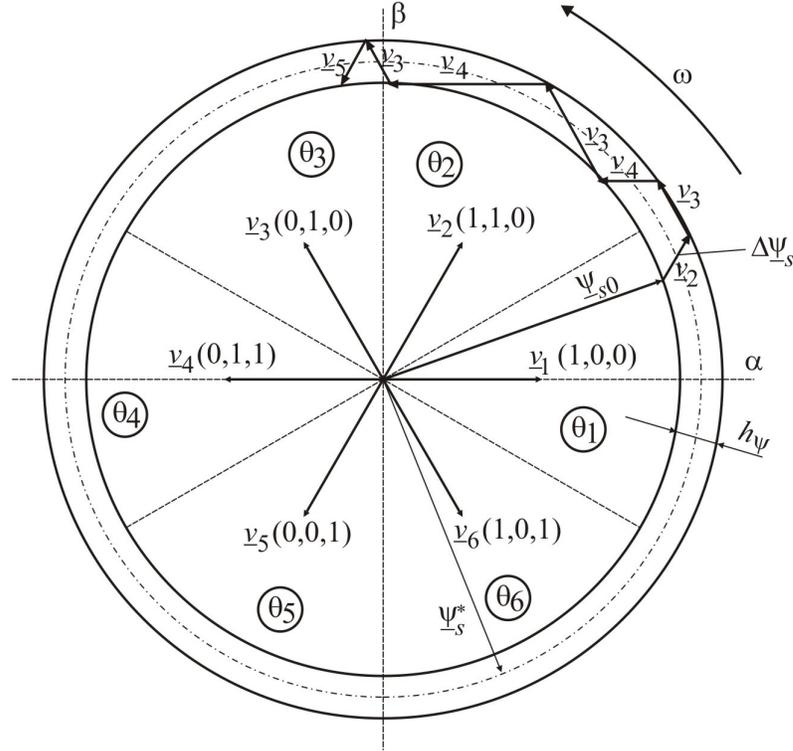
**Fig. 2.26.** Discrete stator voltage vectors  $\underline{V}_i(S_A, S_B, S_C)$  and the evolution of the stator flux trajectory within the hysteresis band  $h_\psi$ .
