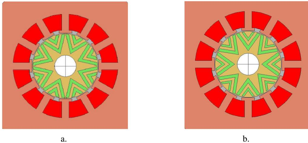
**Fig. 2.11.** Two V flux barriers rotor geometry: a. with same width of flux barriers 2V; b. with different widths of the flux barriers 2VU.
