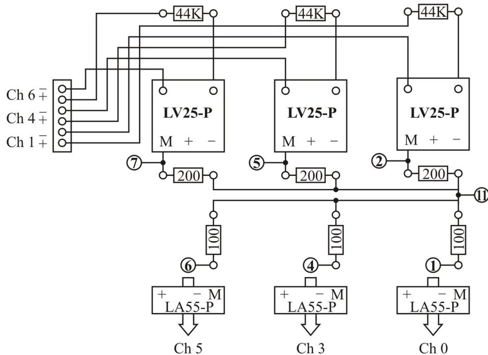
**Fig. 2.30.** The acquisition board scheme.
