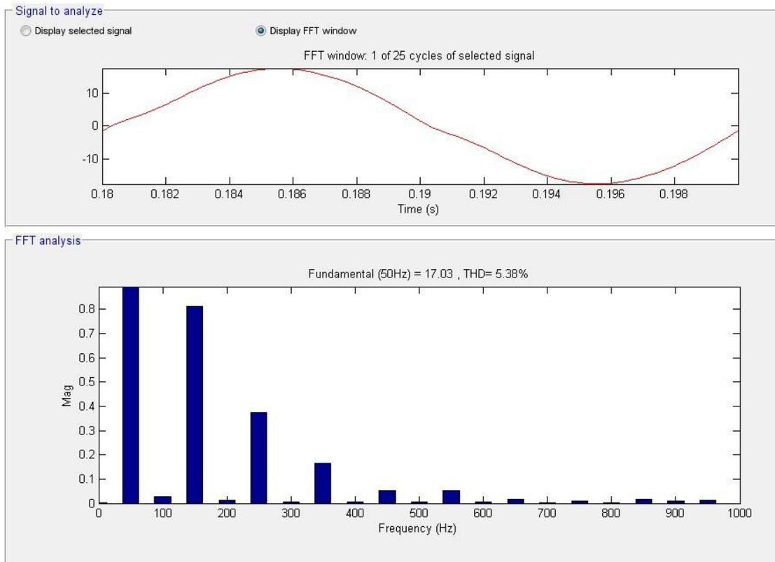
**Fig. 2.117.** FFT for input current range from 0 to 1kHz for Bridgeless IL topology.
