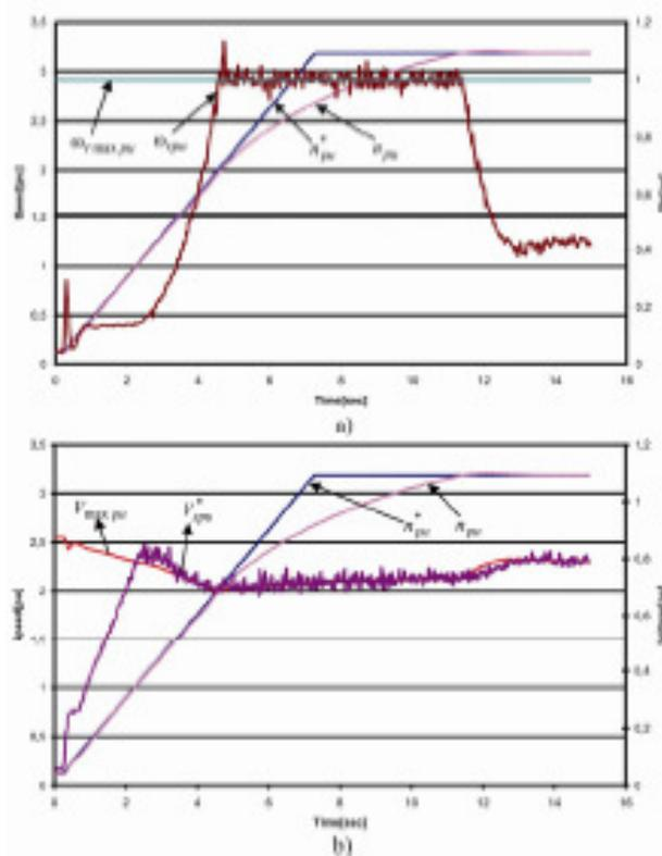
**Fig. 2.59.** Acceleration performance showing, at 0.06pu accelerating gradient: a) the speed ( $n_{pu}^*$ ,  $n_{pu}$ ), rotor angular frequency ( $\omega_{rmax pu}$ ,  $\omega_{rpu}$ ); b) the speed ( $n_{pu}^*$ ,  $n_{pu}$ ), the regulated stator voltage ( $V_{apu}^*$ ,  $V_{apu}$ ) and the maximum terminal voltage ( $V_{max pu}$ ).
