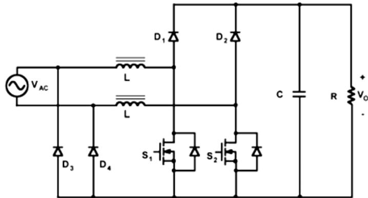
Fig. 2.64. Bridgeless PFC converter topology.
