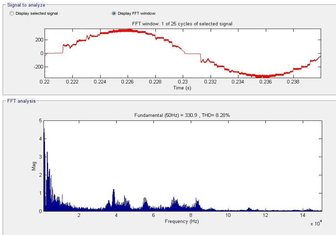
**Fig. 2.77.** FFT for voltage measured after EMI filter within 1 to 150kHz range for the Boost topology.
