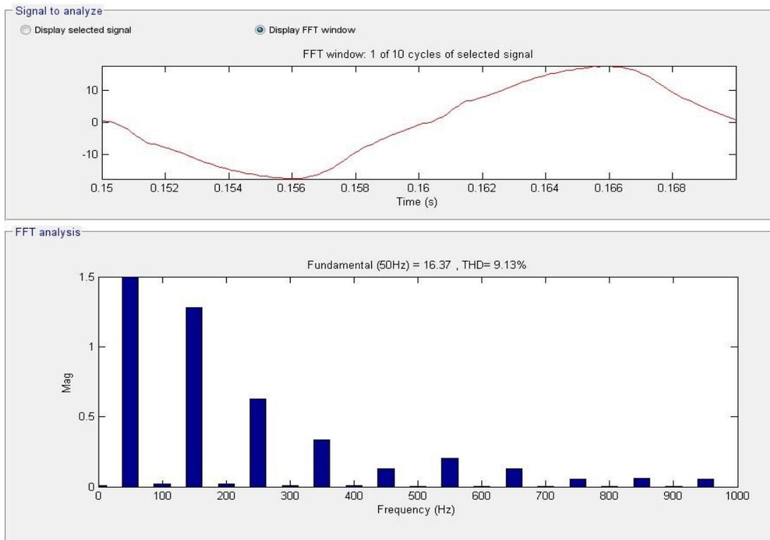
**Fig. 2.104.** FFT for input current range from 0 to 1 [kHz] for Boost IL topology.
