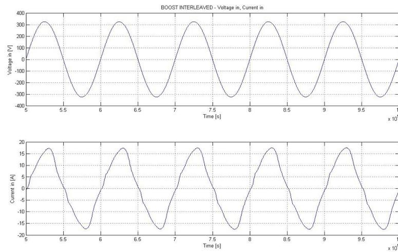
**Fig. 2.97.** Zoom on input voltage & input current for the Boost IL topology.
