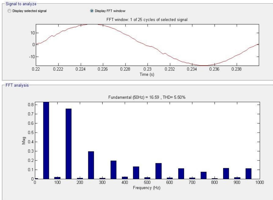
**Fig. 2.74.** FFT for input current range from 0 to 1kHz for Boost topology.
