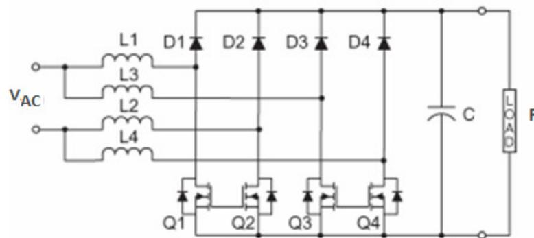
**Fig. 2.95.** Bridgeless IL PFC converter topology.
