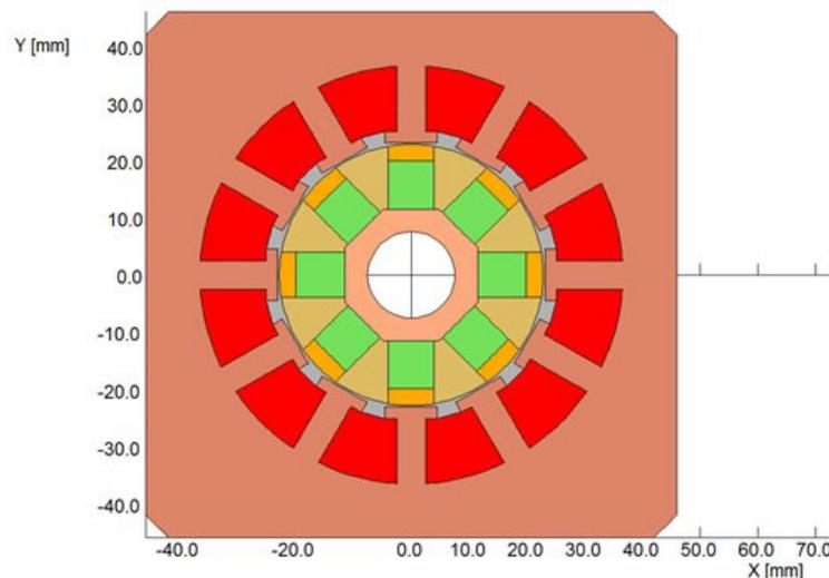
Fig. 2.16. PMSM wit flux concentrator (PMSM-FC).
