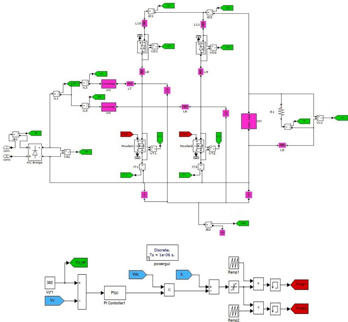
**Fig. 2.94.** Boost IL PFC converter model implementation in Matlab/Simulink.
