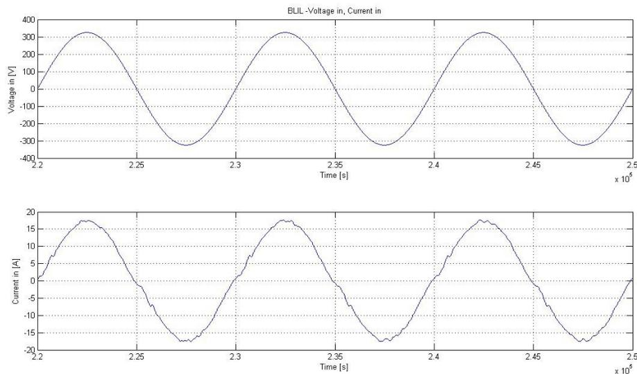
**Fig. 2.110.** Zoom on input voltage & input current for the Bridgeless IL topology.
