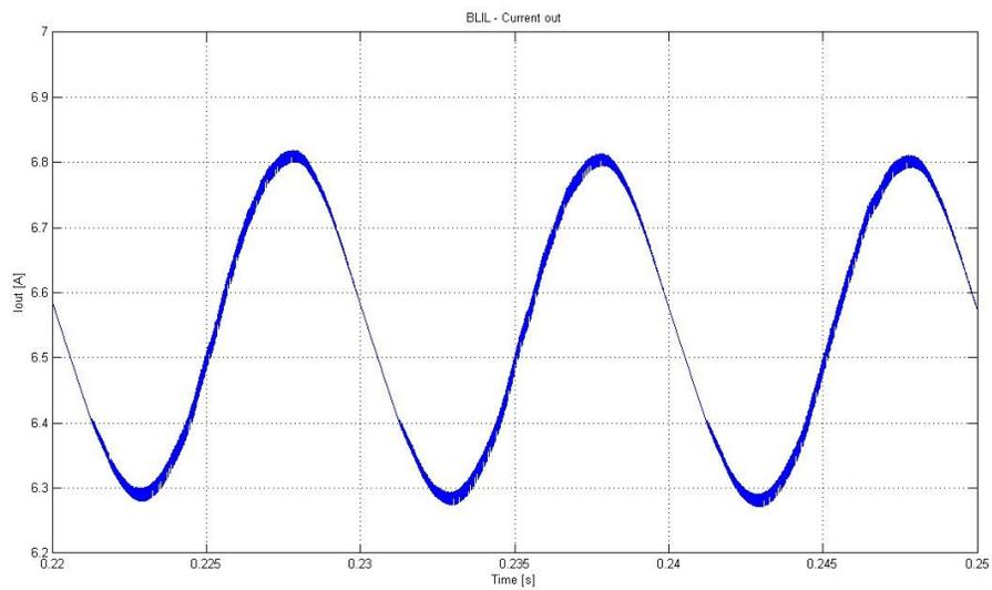
**Fig. 2.112.** Zoom on capacitor current for the Bridgeless IL topology.
