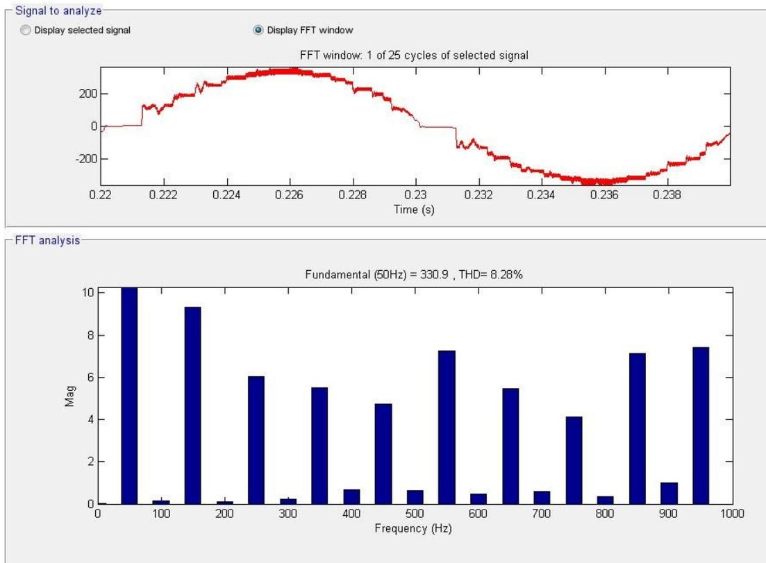
**Fig. 2.76.** FFT for voltage measured after EMI filter within 0 to 1kHz range for the Boost topology.
