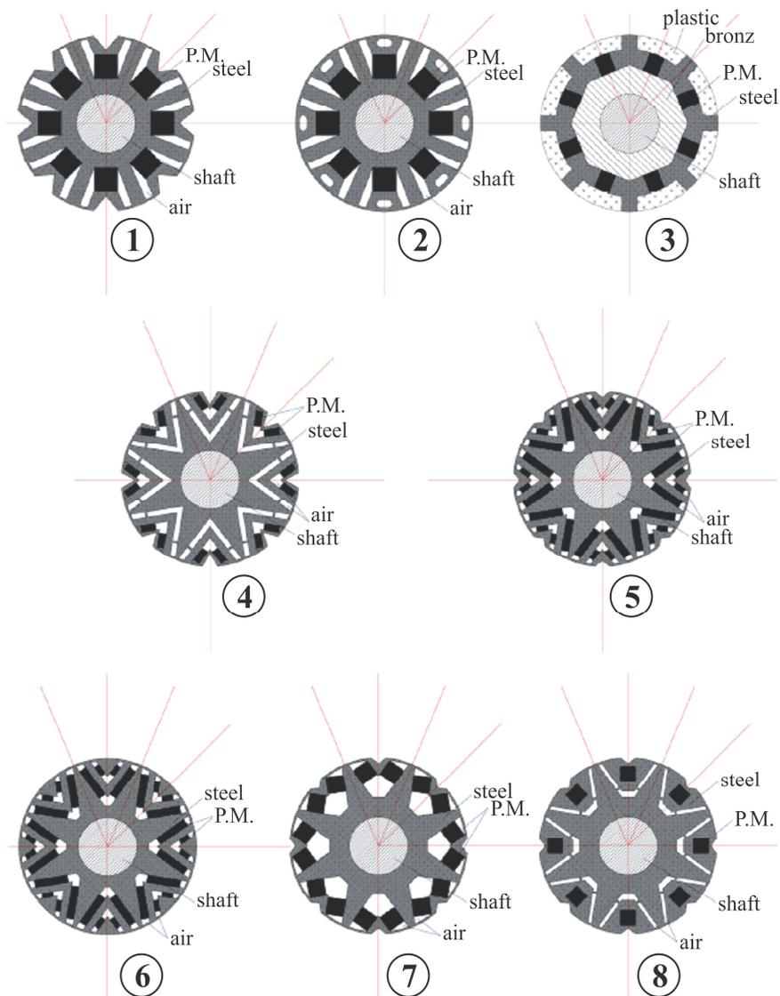
**Fig. 2.5.** The proposed rotor type variants for PMSynRM .
