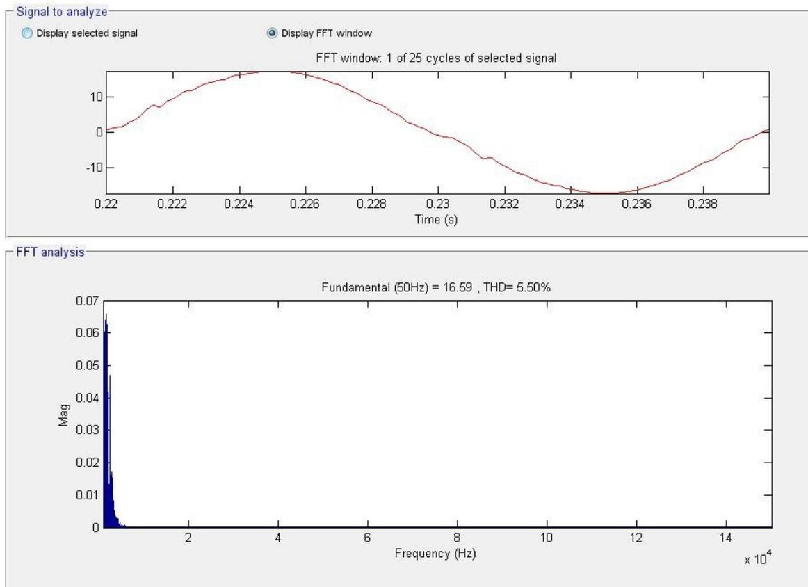
**Fig. 2.75.** FFT for input current range from 1 to 150kHz for Boost topology.
