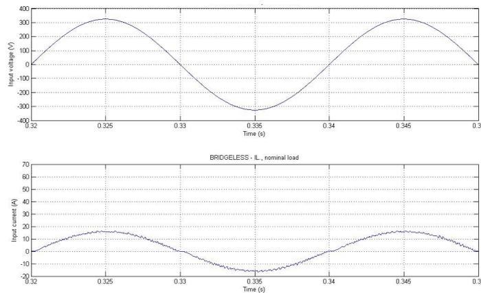
**Fig. 2.80.** Zoom on input voltage & input current for the Bridgeless topology.
