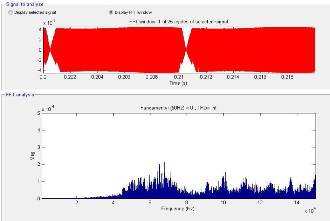
**Fig. 2.92.** FFT current between C and ground within 1 to 150kHz range for the Bridgeless topology.
