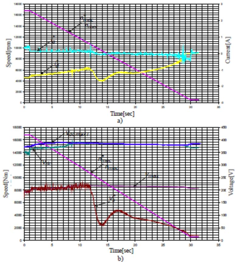
Fig. 2.54. Decelerating performance of the proposed speed regulation drive system of MSMPS.
