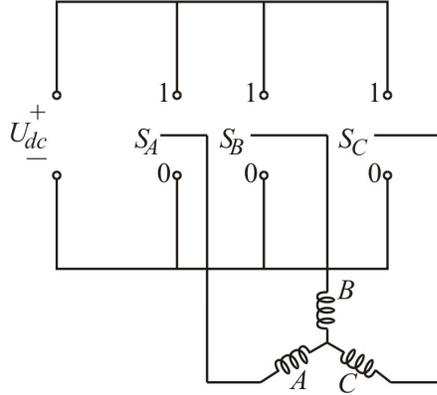
**Fig. 2.25.** Model of voltage inverter
