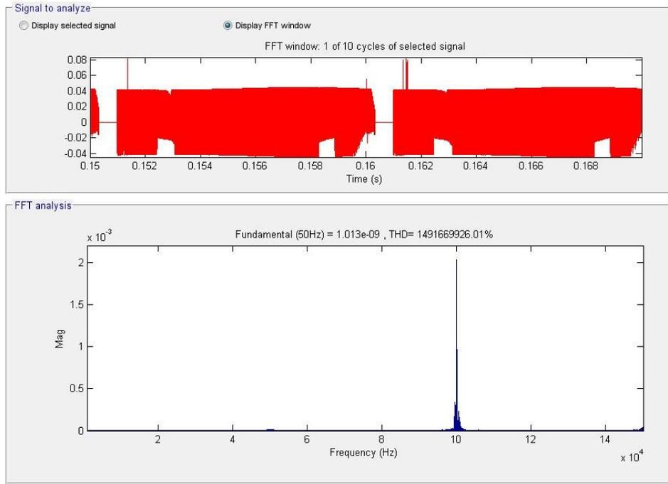
**Fig. 2.109.** FFT current between C and ground within 1 to 150kHz range for the Boost IL topology.
