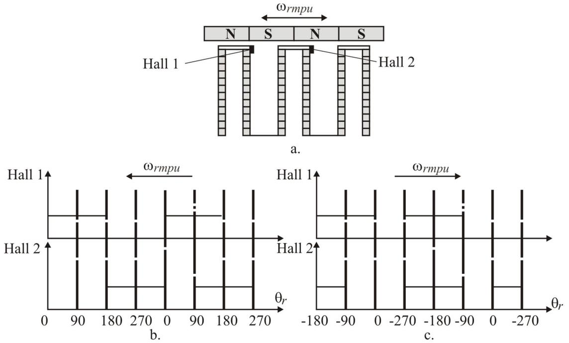
**Fig. 2.50.** Hall-effect position sensor signals.
