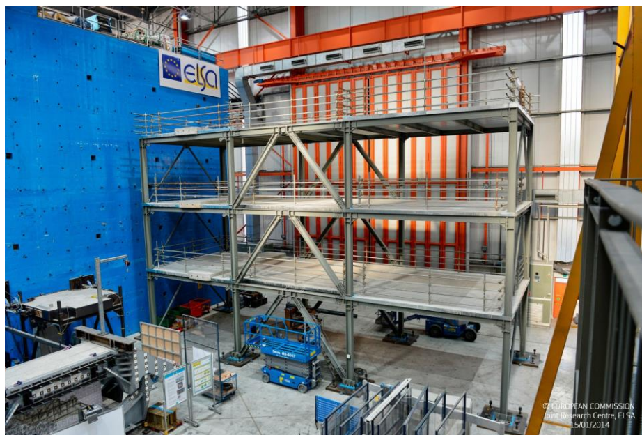
Figure 6. Experimental mock-up in front of the reaction wall.
