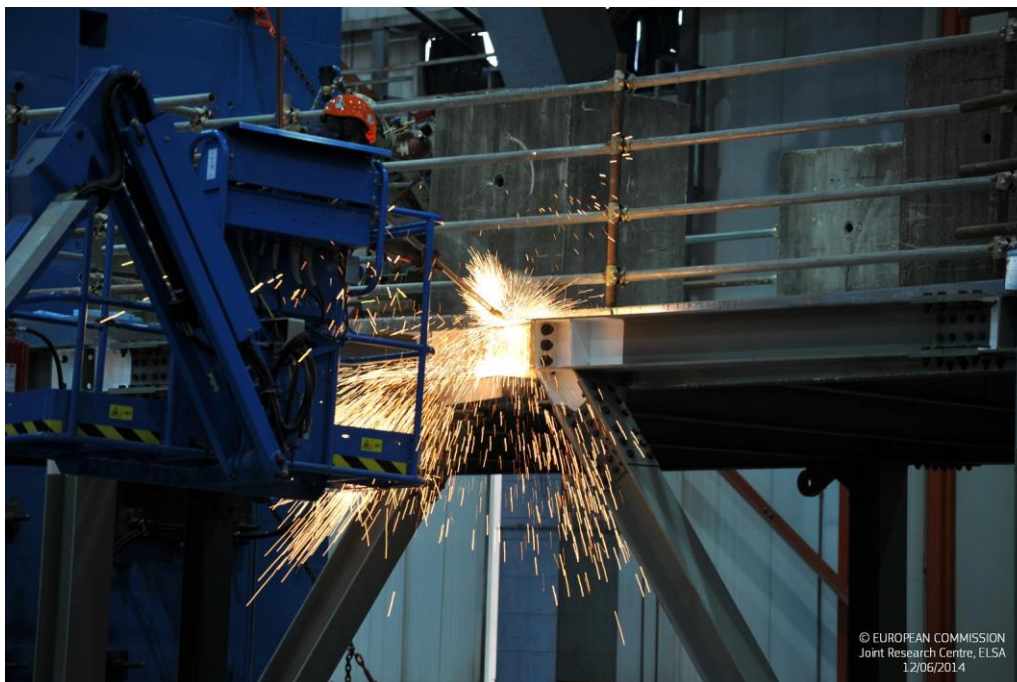
Figure 70. Cutting process of the links
