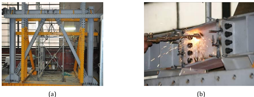
Figure 27. One story frame: (a) experimental setup and (b) flame cutting of the link.
