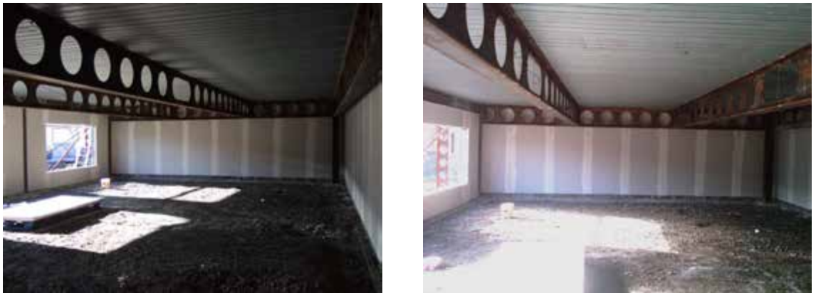
Figure 7.44 : Test compartment with long unprotected cellular beams
