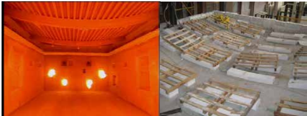
Figure 7.38 Tested floor during and after the fire
