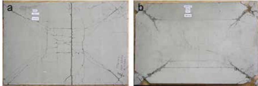
Tensile failure of reinforcement
