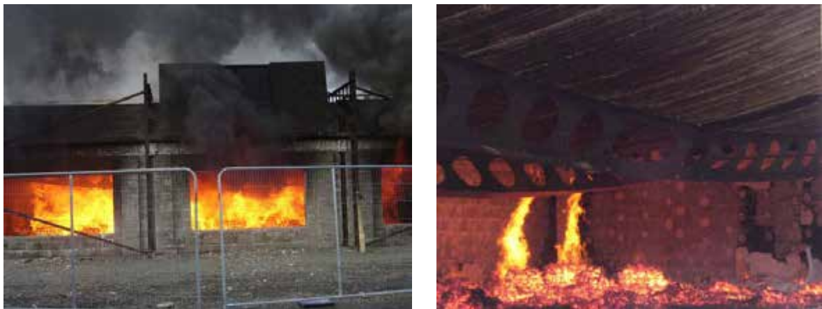
Figure IV : Fire test and structural elements after the fire
