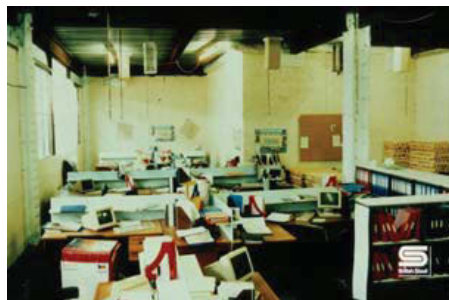
Fire load with real office furniture
