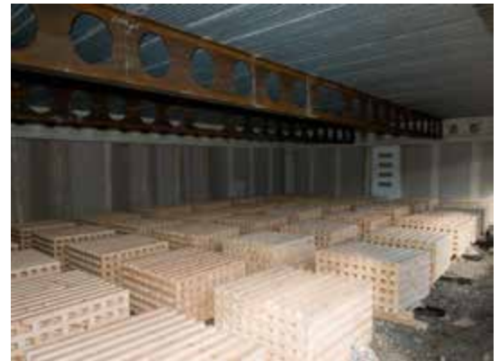
Figure 7.49 : (a) Vertical static load , (b) Wooden cribs used for the fire load
