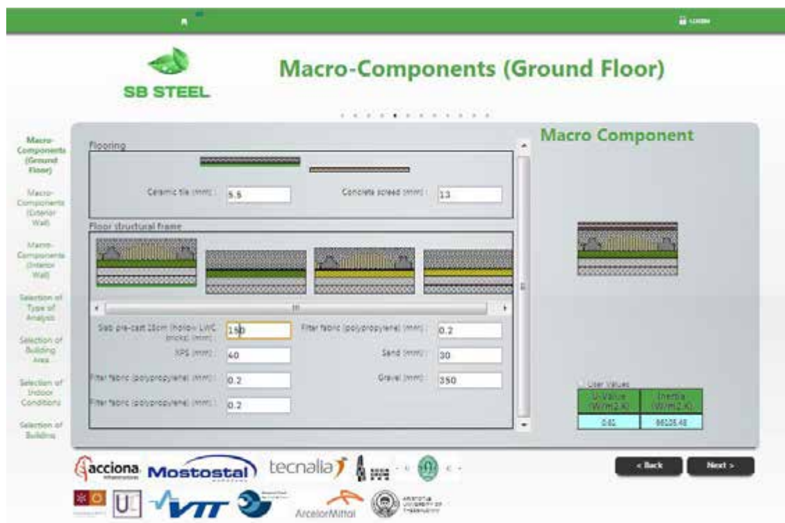
Figure 40. Building's ground floor macro-component identification.
