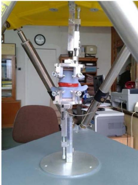
Figure 3.52. The device's clamping mode on the Stewart platform.
