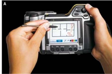
Fig. 2.26. – The FLIR B200 device used in thermographic studying. A - the back of the device with the display and its setting. B - the underside of the device with the connecting hubs. C - normal photographic image in the display. D - Thermographic image of the same object in detail C. [112]
