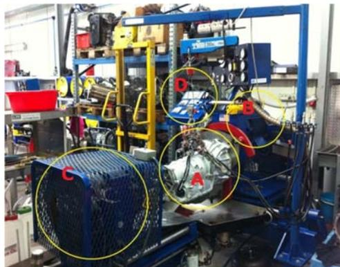
Fig. 2.23. Dynamic test rig for automatic gearbox at variable speeds.
