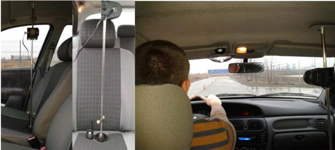
Figure 3.30. The sensor in the first position for determining the C1 vertebra movements.
