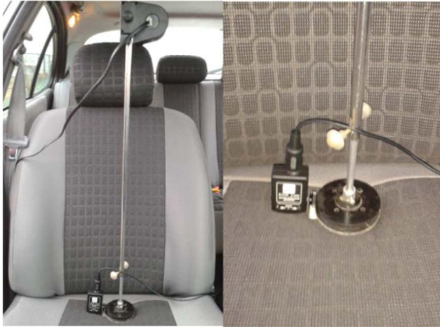
Figure 3.59. Layout accelerometer for acceleration registration in lateral plan.
