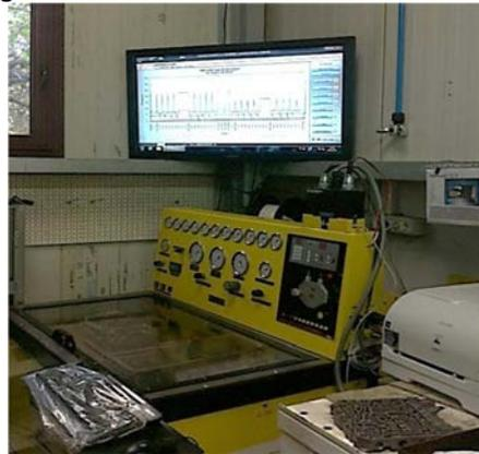
Fig. 2.20. The test rig of the control block for determining the functional parameters of the clutches and brakes with the visualization of the register data.
