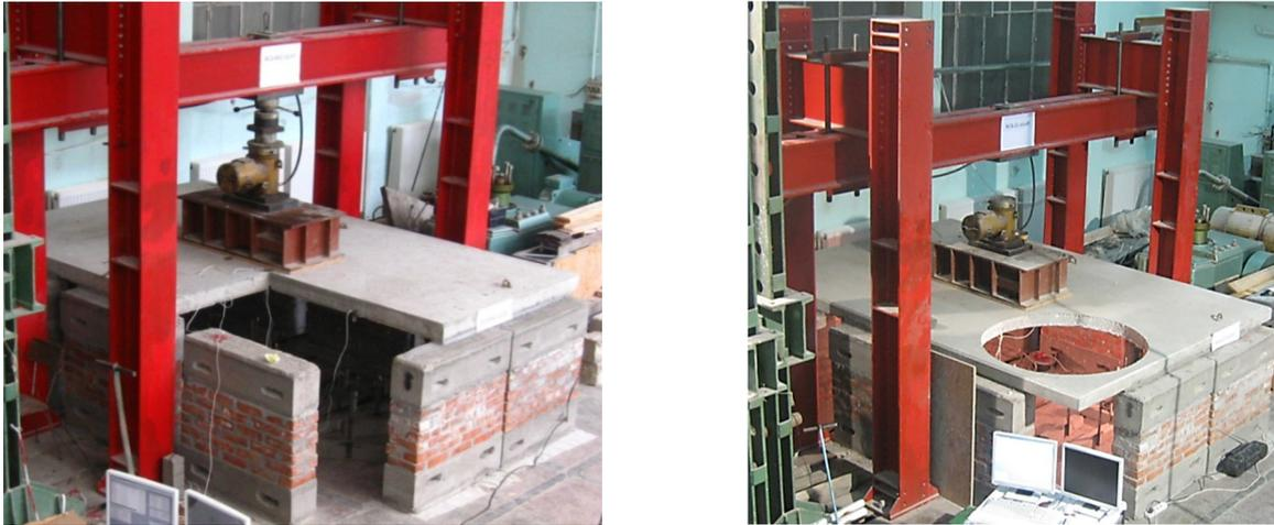
Figure 43. Test setup for RSC-01 and CC-01 slabs
