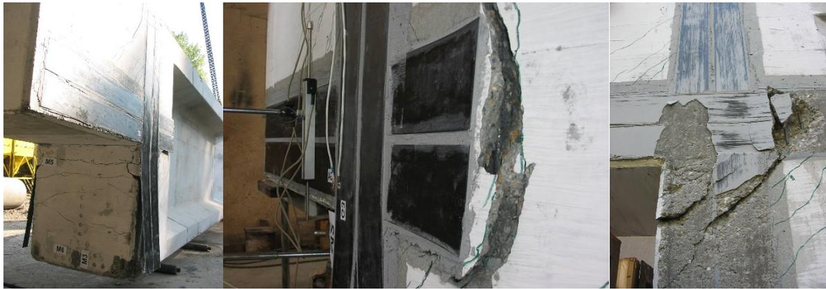
Figure 69. Vertical and horizontal CFRP plates peeling-off from the RC4 element
