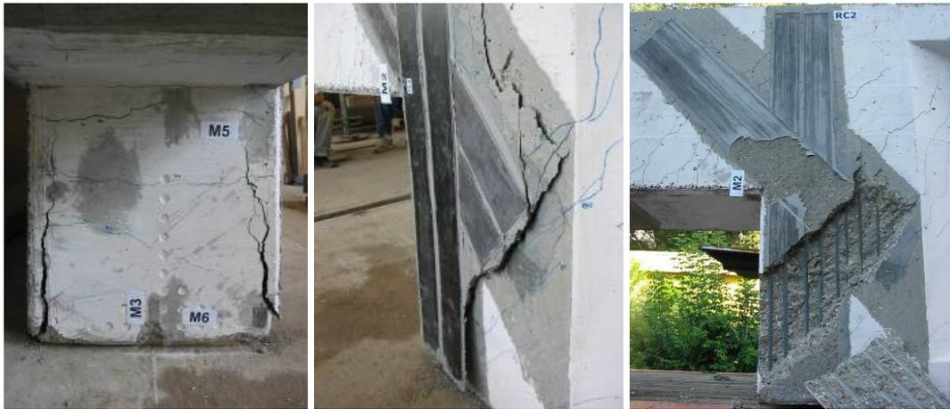
Figure 62. Photographs showing the vertical and inclined CFRP plates peeling-off from element RC2.
