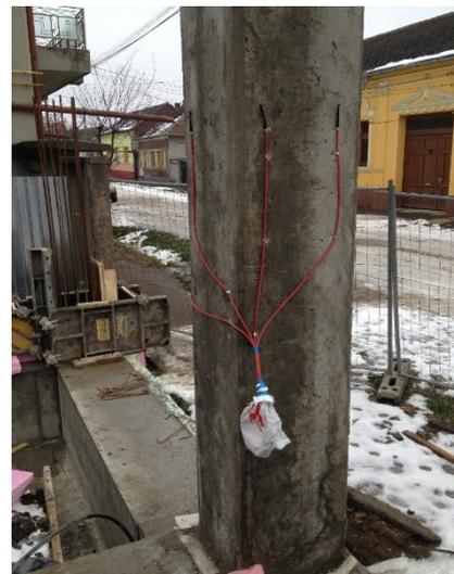
Figure 96. Detail of the ground floor column with the mounted sensors
