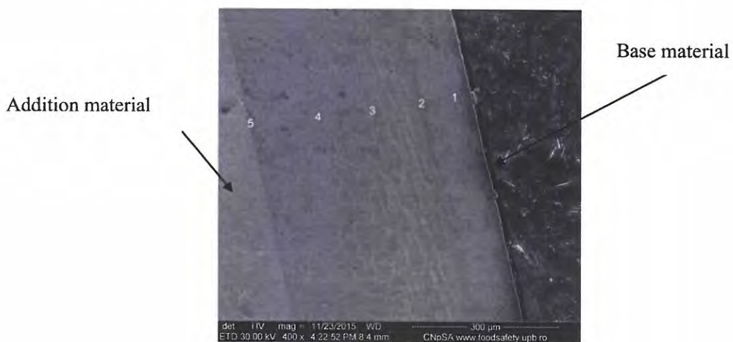
Figure 5.34. Detection points of local chemical composition, Zone A (400x). 1) MB; 2-4) ZIT; 5) interfaces with melted addition material.
