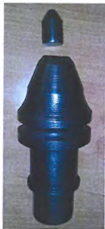
Figure 5.10. mill knife for asphalt stripping machines: 1) reinforcement-cutting body equipped with self-protection system to wear; 2) knife support from low alloyed steel with chromium; 3) spin self-blocking system.
