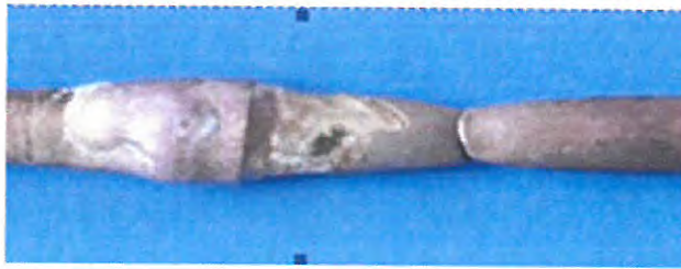
Figure 5.8. Sample broke by applying traction.
