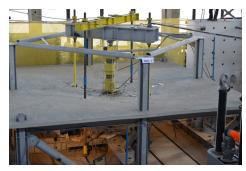
Fig. 5. Experimental test on 3D composite frame system
