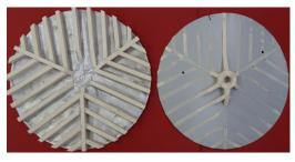
Fig. 4d. core shear (MEC 2)
