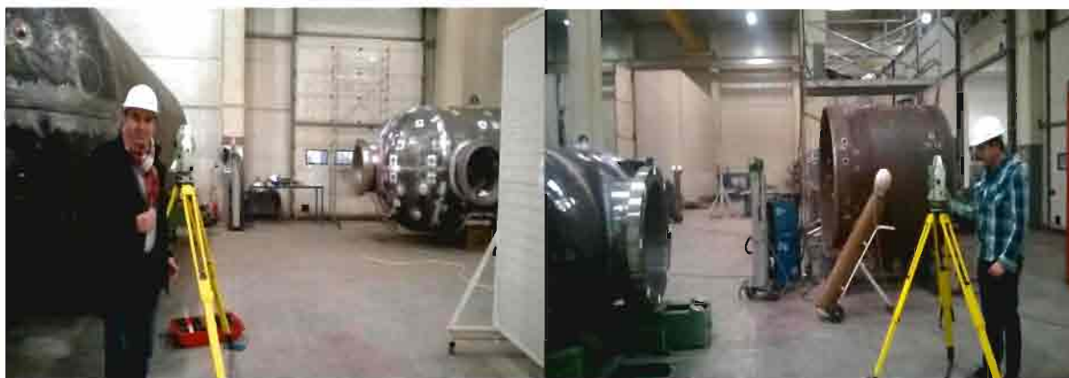
Figure 2.58. Procces of data colectiong inside of powerplant using Leica 1200 Series
