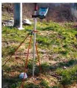
Figure 2.29. Marking of the FENO reference mark and the sketch of the geodetic support network
