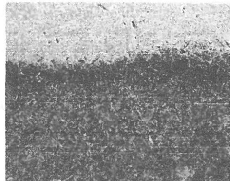
Fig.5.8. Microstructure of the gaseous nitrided layer – x500
