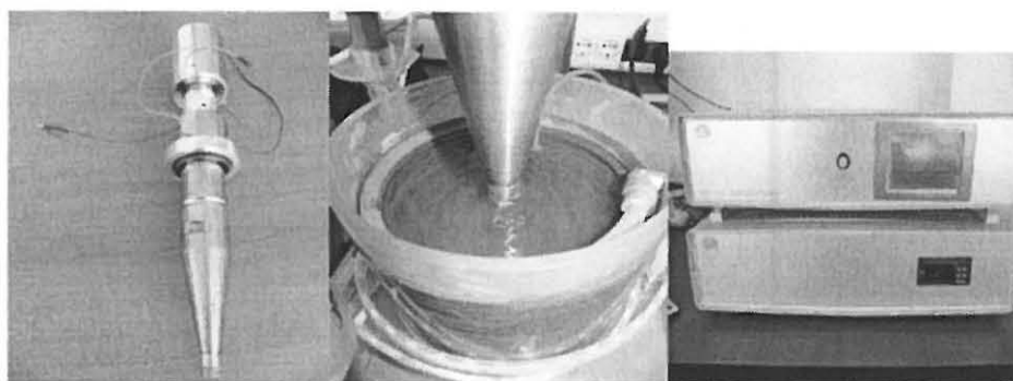
Fig. 2.3 The specimen during the cavitation erosion procedure
