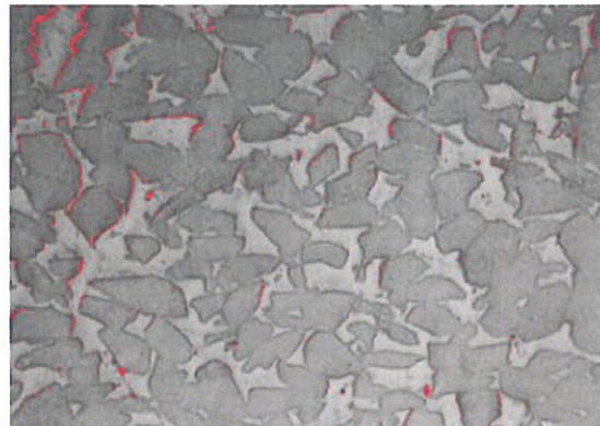
Figure 9 Processed micrograph illustrating the porosity degree
