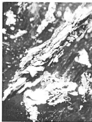
Fig.6. Silver with dendritic aspect (x20)
