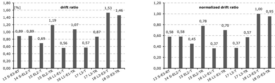
Figure 4-9 Drift ratio for all tested specimens
