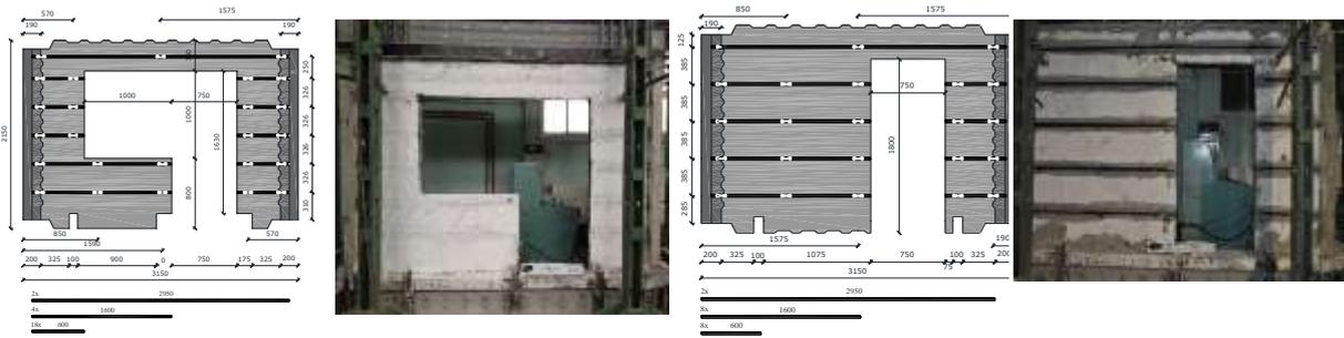
Figure 3-4 The position of the EBR CFRP laminates
