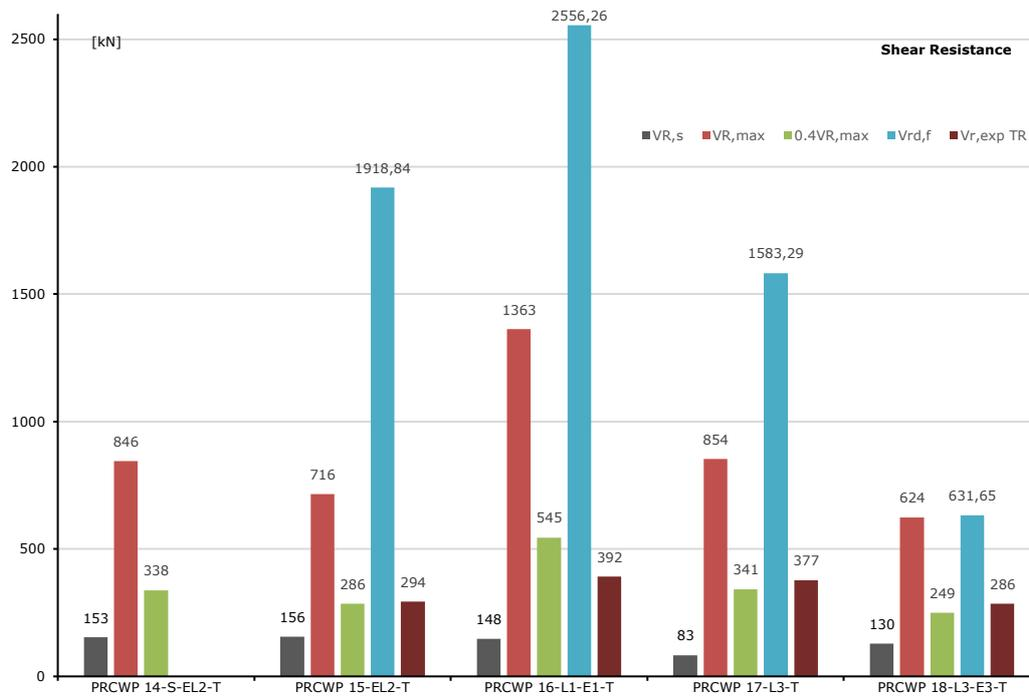
Figure 4-12 Shear resistance retrofitted specimens comparison
