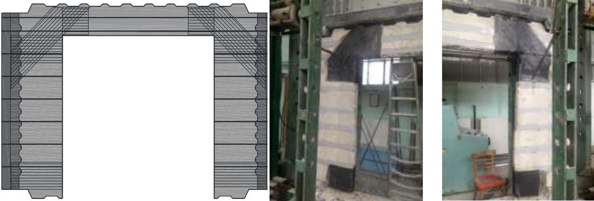
Figure 3-3 Strengthening strategy using NSM-CFRP combined with ERB CFRP
