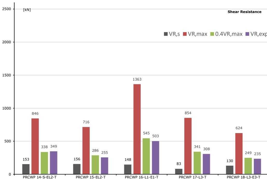
Figure 4-11 Shear resistance of reference specimens comparison
