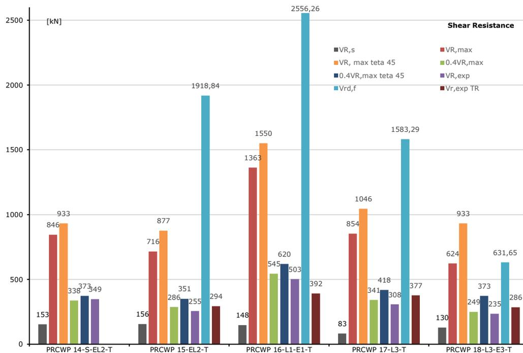
Figure 4-13 Shear resistance comparison between computed elements
