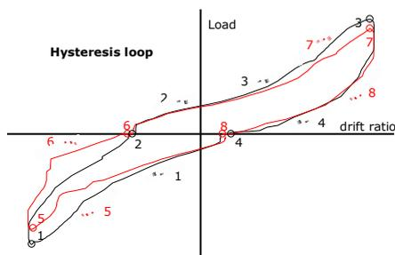
Figure 4-1 Cycles' loading points and subsections
