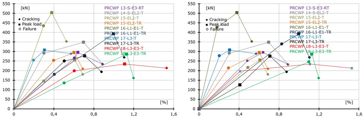
Figure 4-5 Backbone Envelope comparison: (left) Type 1; (right) Type 2
