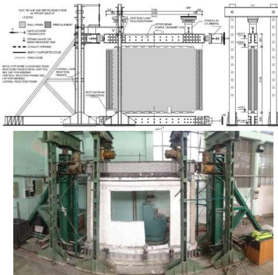
Figure 3-5 Experimental test set-up
