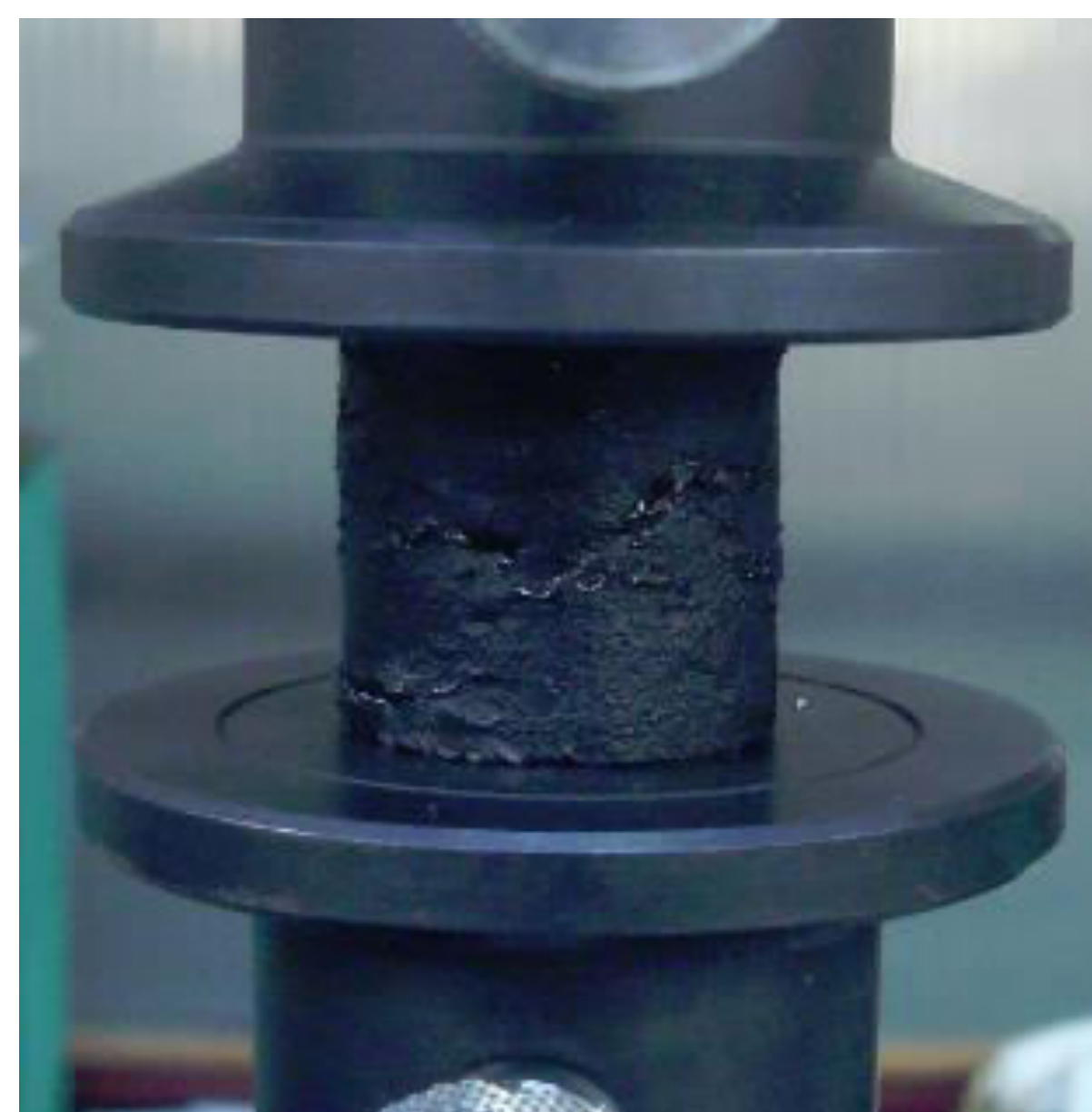
Fig. 5. A 10 kN Walter+Bay fatigue testing machine
