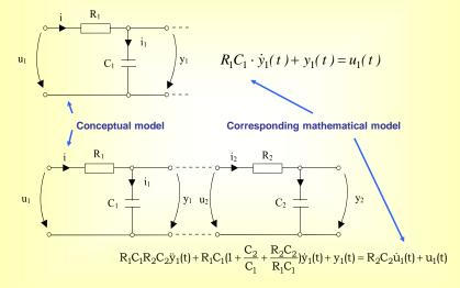
**Black-box** — general term for a system/process, viewed only from the point of view of inputs, outputs and function performed, considered, be the case, as a transfer feature from the input to the output, irrespective of the actual structure and phenomena within the system/process;
