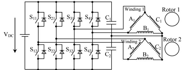
Fig. 1 Proposed single stator dual rotor PMSM drive-system with two distinct stator windings and four leg inverter
