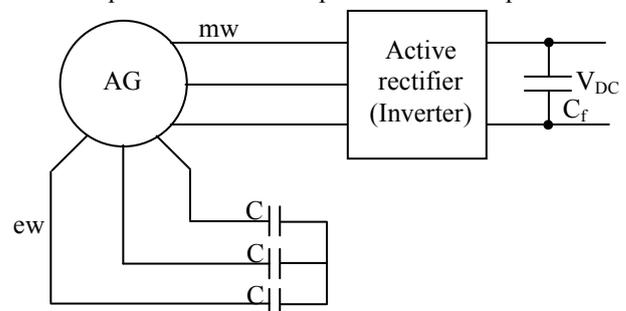
Fig.1. Dual stator winding induction generator with a rectifier (proposed scheme).
