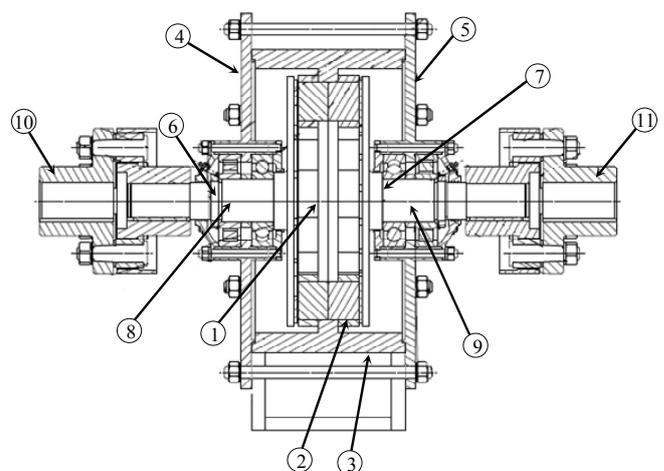
Fig.1. Longitudinal section through the dual PM rotors machine.
