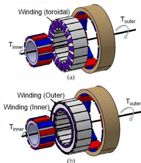
Fig. 1. Exploded view of (a) toroidally and (b) radially wound dual-rotor machines with 12 rotor poles and 18 stator slots.
