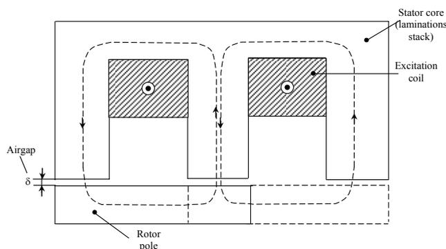
Fig. 1. Longitudinal magnetic circuit section.
