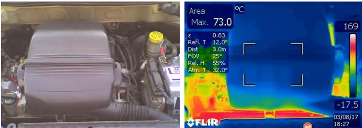
Figure 11. Thermal field on the shell of the air filter
