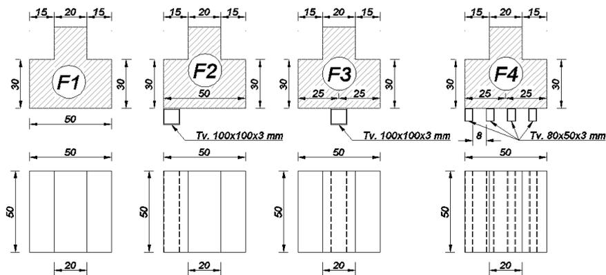
Figure 22. Concrete scaled foundations
