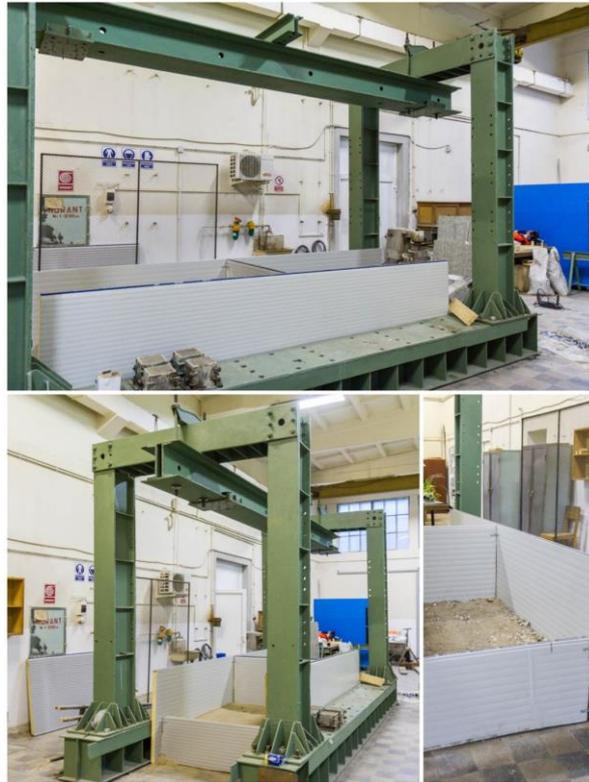
The test stand was constructed as two box shaped areas, one for each soil type. The foundations were laid on each of the soil surface and pushed horizontally, while horizontal and vertical displacements were measured along with the pushing force. For this particular study four foundation types and two types of soil were analyzed (figure 22).
