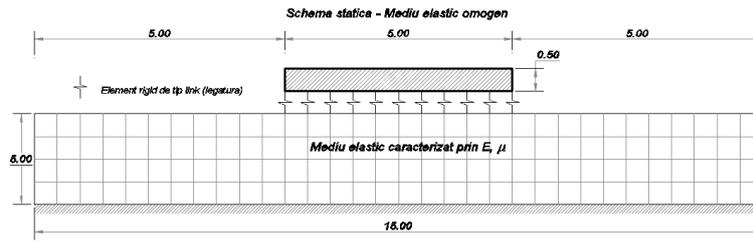
Figure 18. Beam on continuous elastic media (solid)
