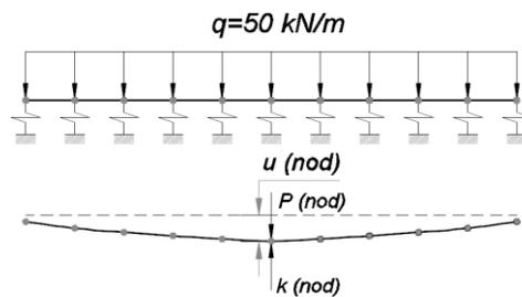
Figure 20. Static model for calculating P load
