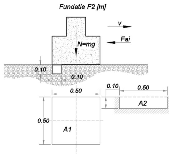
Figure 21. Prismatic rugosity on a concrete foundation
