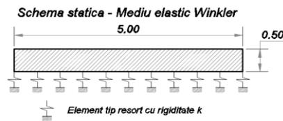
Figure 19. Beam on Winkler type elastic support
