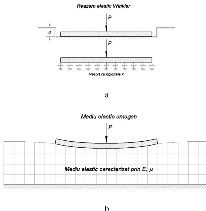
Figure 18. Rigid body on Winkler foundation (a) and flexible body on solid elements (b)
