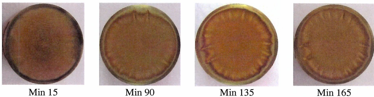
Fig.4.56 Images of specimen surface at different cavitation exposure time ( Sample 2 )
