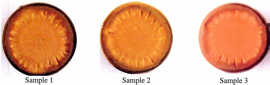
Fig.4.15 Macroscopic images (taken with a Canon A480 camera) of the surfaces eroded by vibratory cavitation, after 165 minutes of cavitation exposure
