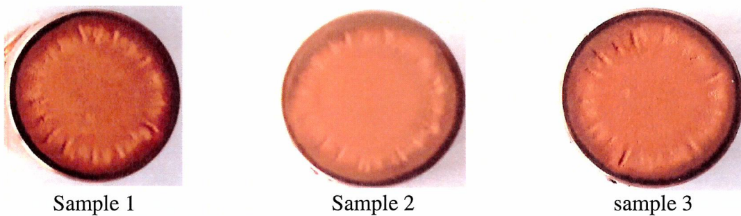
Fig.4.33 Macroscopic images (taken with a Canon A480 camera) of the surfaces eroded by vibratory cavitation, after 165 minutes of cavitation exposure
