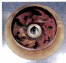
Destroyed by cavitation
