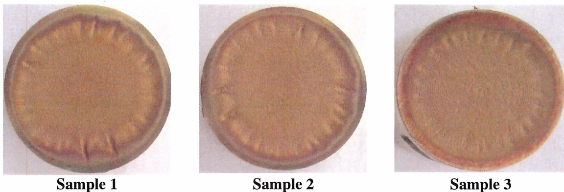
Fig.4.57 Macroscopic images (taken with a Canon A480 camera) of the surfaces eroded by vibratory cavitation, after 165 minutes of cavitation exposure
