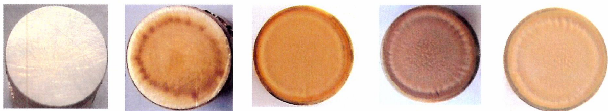
Min 0 Min 15 Min 90 Min 135 Min 165 Fig.3. Images of specimen surface at different cavitation exposure time (Sample 2)
