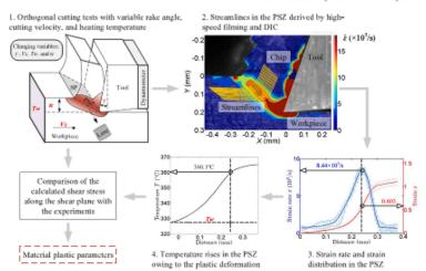
Fig. 2. Flowchart of material testing based on metal cutting process.
