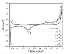
Fig. 4. Cyclic voltammograms on Pt electrode in 0.5 M CH<sub>3</sub>COOH/0.25 M in the absence/presence of u-histidine, scan rate 50 mV s<sup>-1</sup>.
