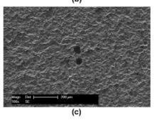
Fig. 8. SEM images obtained for carbon steel samples: abraded without immersion in test solutions (a); after 240 h immersion in the blank solution (b); and after 240 h immersion in the test solution with 10°2 M L-histidine (c).
