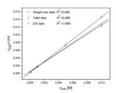
Fig. 6. Langmuir adsorption isotherm for ι-histidine obtained by weight loss, EIS and Tafel data.
