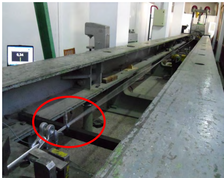
Fig. 2.47. The accelerometer mounted on the conductor for the displacement amplitude recording
