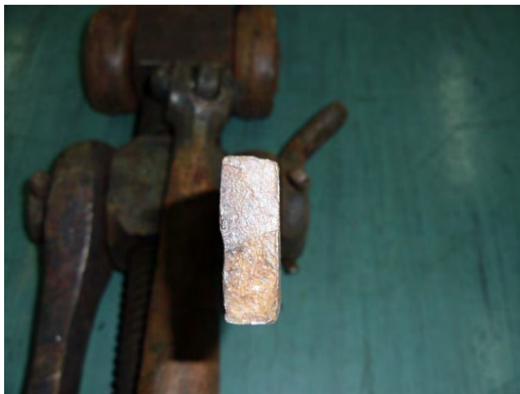
Fig. 2.53. The fracture surface of the connection shoe lining, due to the initiation and propagation of a fatigue crack
