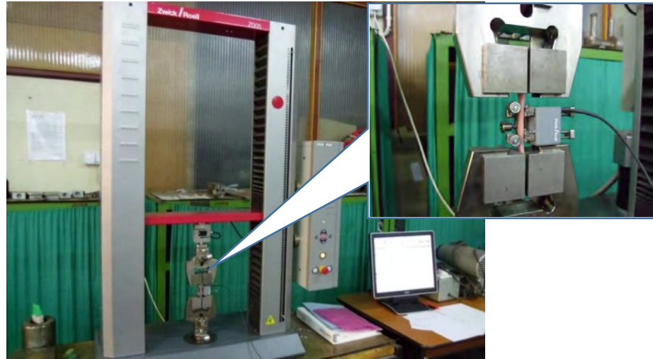
Fig. 1.2. Tensile testing of acrylic resins
