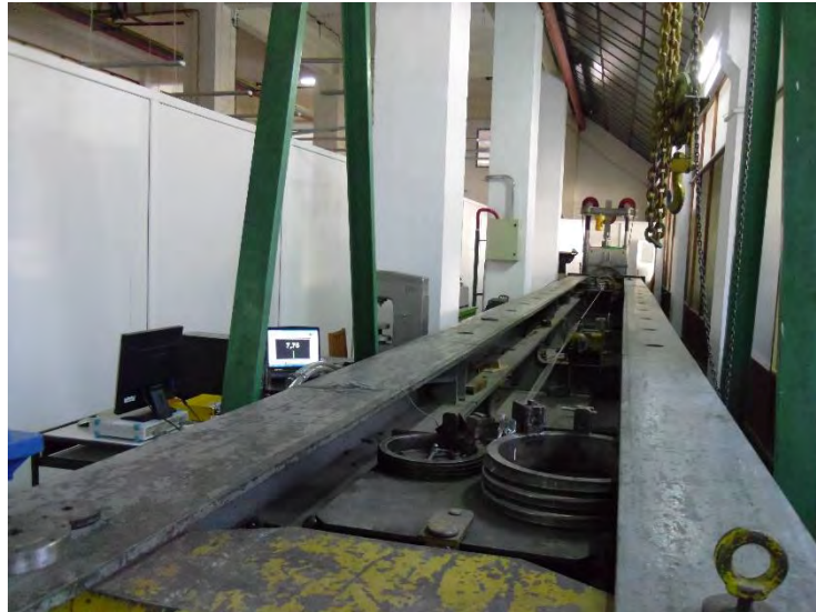
Fig. 2.46. The configuration of the fatigue test of 122-AL1/20-ST1A ACSR conductor
