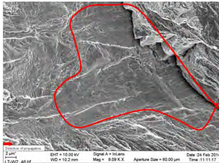
Fig. 2.33. The fracture surface of CT specimen at 9000x magnification for crack propagation in weld.
