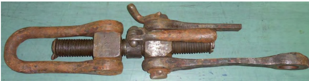
Fig. 2.52. The failure of a wagon coupling from a passenger train
