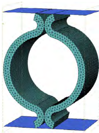
Fig. 2.7. The analysis model for compression in longitudinal direction of the cell, [49]
