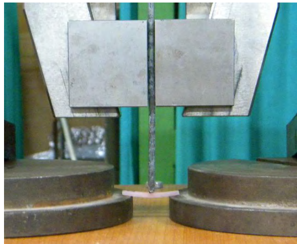
Fig. 1.3. Three-point bending testing of acrylic resins
