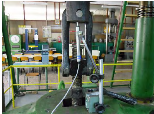
Fig. 2.63. The tensile tests on the screw – nuts – shackle assembly.
