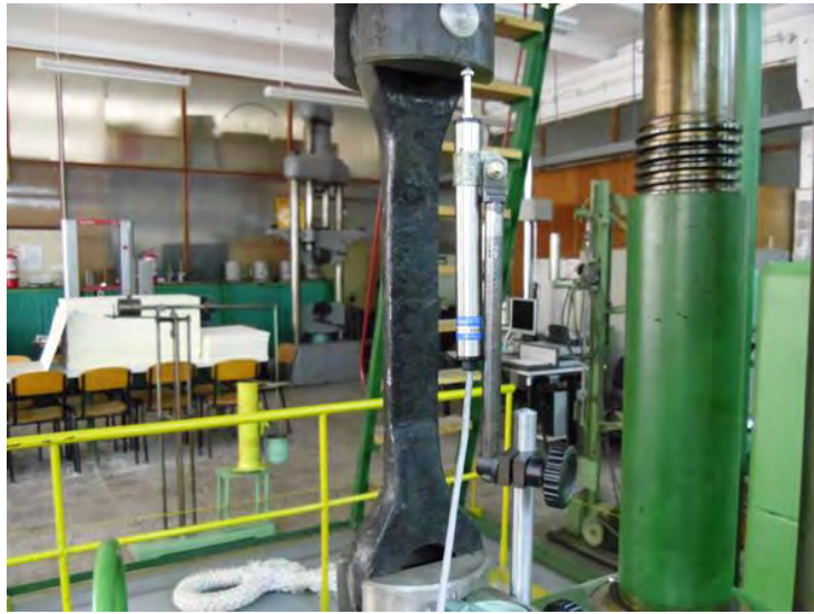
Fig. 2.62. The tensile test on a link of the coupling.
