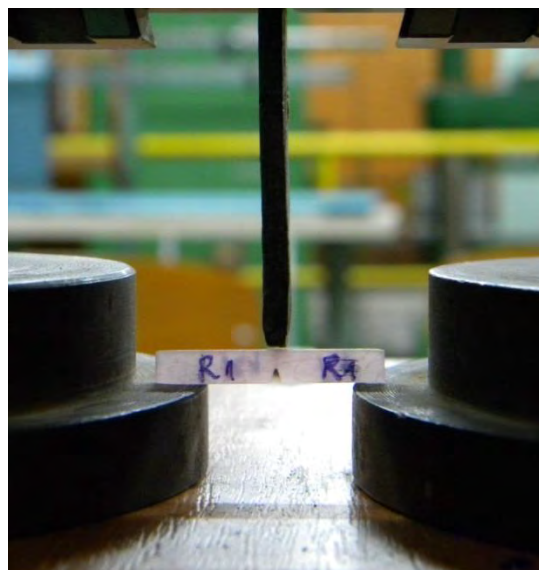
Fig. 1.8. The SENB specimen from acrylic resin
