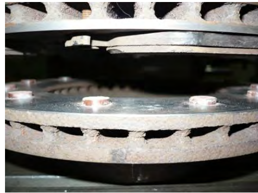
Fig. 3.3.1.34 Mounting with 2 pads
