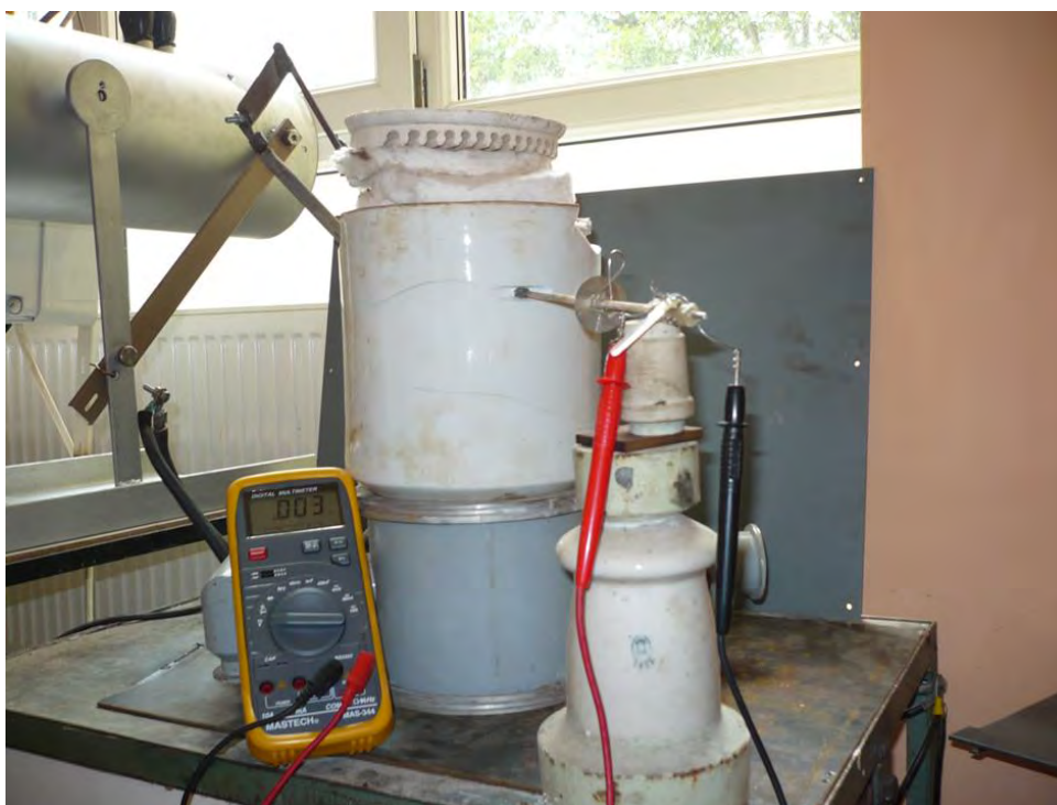
Fig. 3.1.1.5 Basalt powder melting furnace
