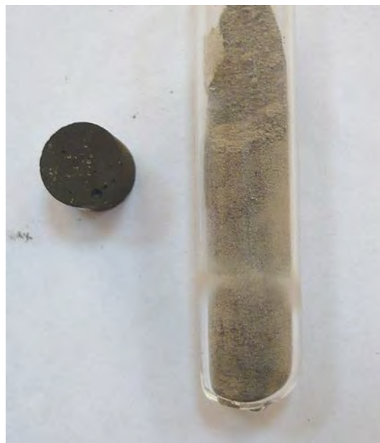
Fig. 3.1.1.6 Basalt powder inside the quartz capsule
