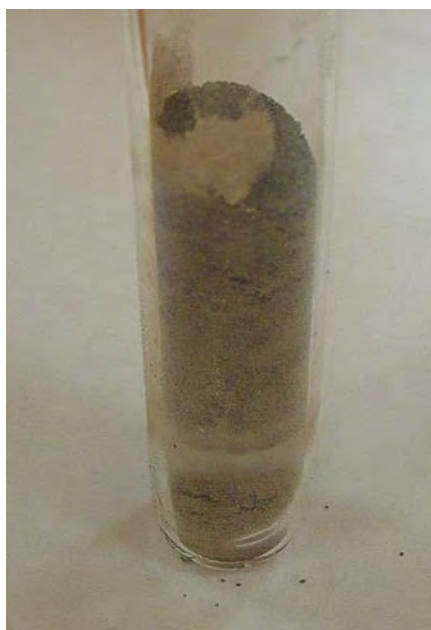
Fig. 3.1.1.6 Basalt powder inside the quartz capsule
