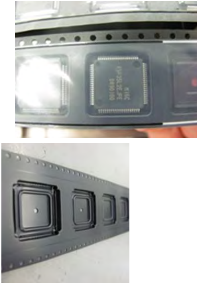
Fig. 2.2.3.19 Rolls with sprocket holes on one side (a) and both sides (b)
