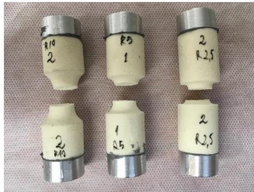
Figure 4.14 PUR specimens used in the triaxial state of stress-critical plastic strain study
