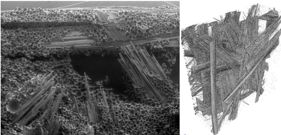
Figure 4.11 SEM image of the fracture area and CT scan showcasing the glass fibre distribution [36]
