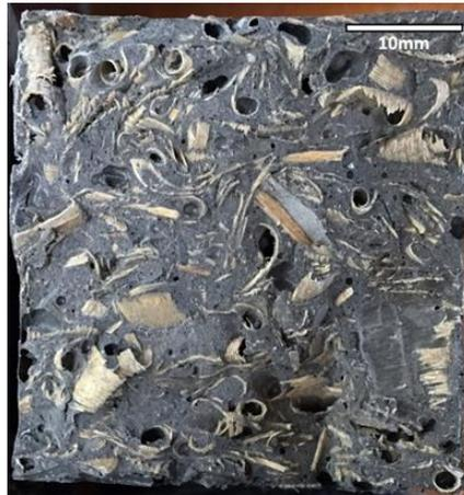
Figure 4.22 Geopolymer – wood fibre composite cross section
