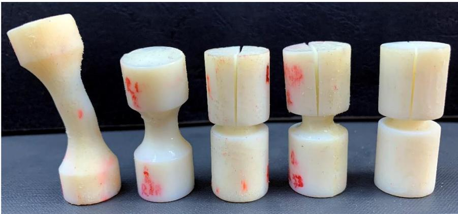
Figure 3.15 Specimen condition after the compressive tests
