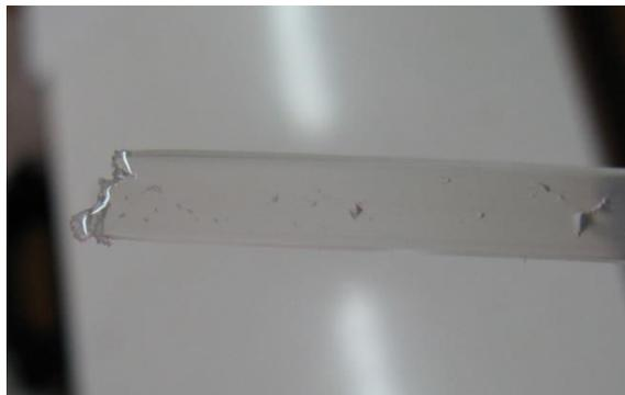
Figure 3.4 Void nucleation in a polyamid compound
