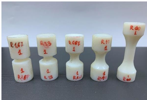
Figure 3.13 Notched cylindrical compressive specimens
