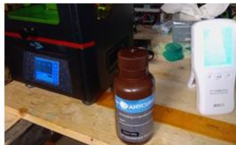
Fig. 2. Printer, resin and apparatus for made probes in the 3D printed process
