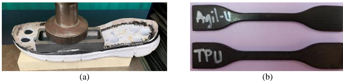
Fig. 1. Dogbone specimens (a) taken from sports shoes (b) realized through rapid prototyping
