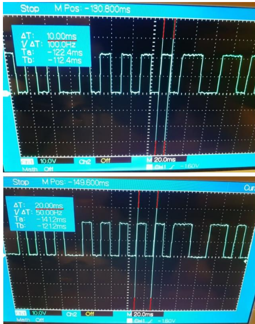
Figure 20. Generated Digital Signal based on payload delivered by the Gateway Application at 10 ms recurrence
