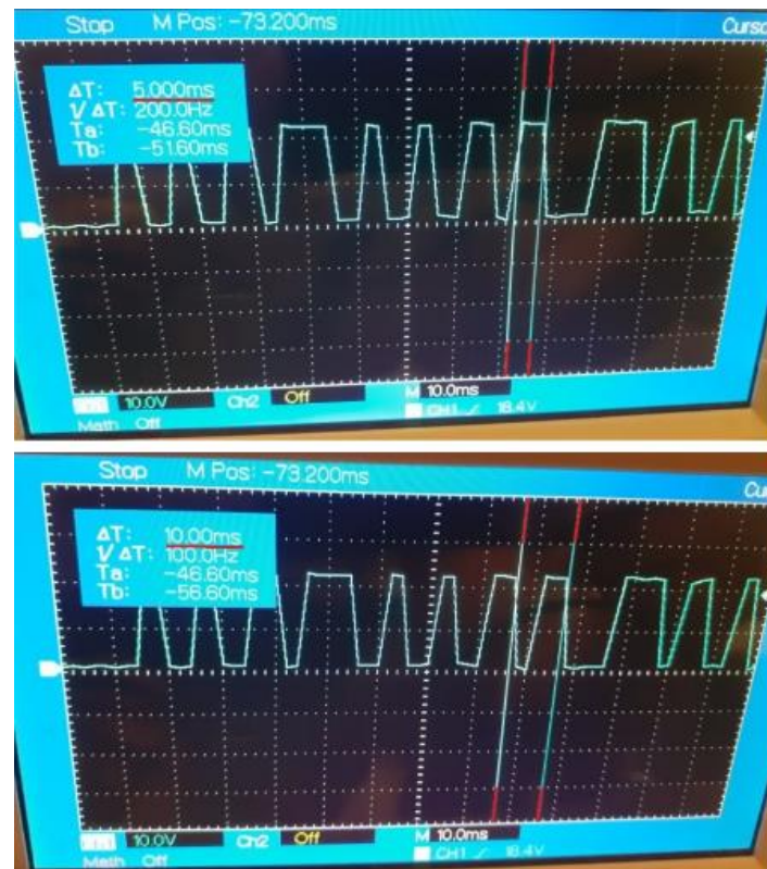
Figure 21. Generated Digital Signal based on payload delivered by the Gateway Application at 5 ms recurrence.
