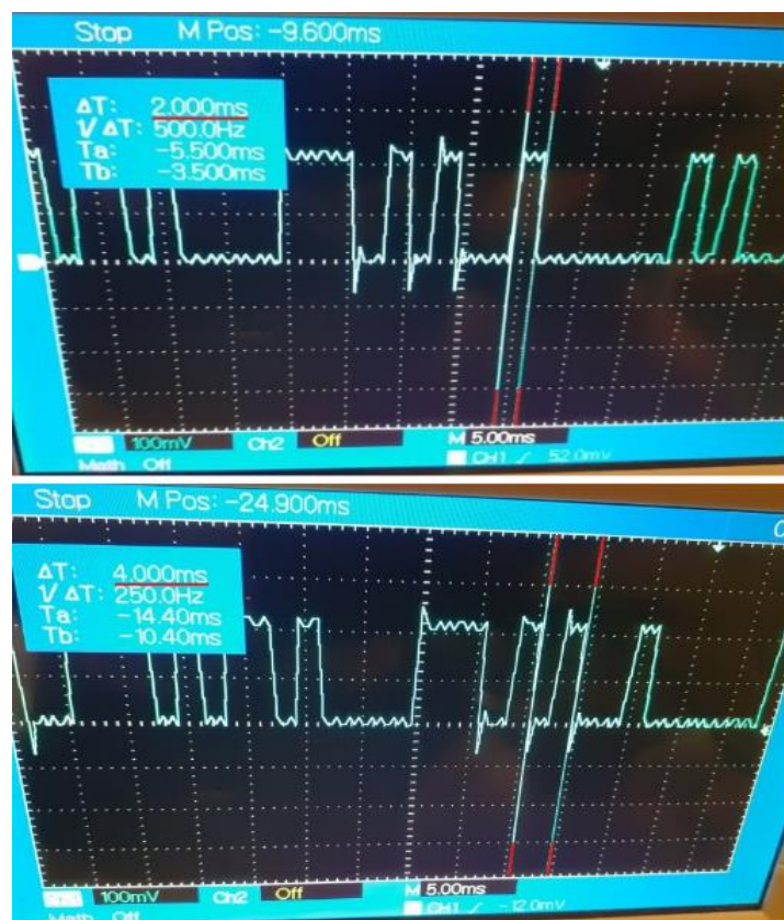
Figure 22. Generated Digital Signal based on payload delivered by the Gateway Application at 2 ms recurrence
