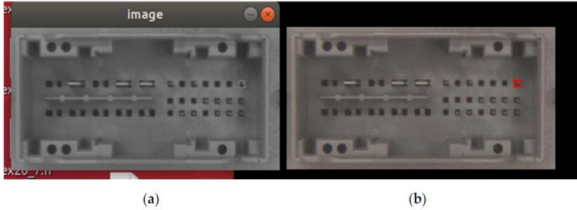
Figure 15. OPC UA publish-subscribe, 20-channel image transmission for ECU automatic optical inspection process in the automotive manufacturing: (a) the received image and (b) the target image
