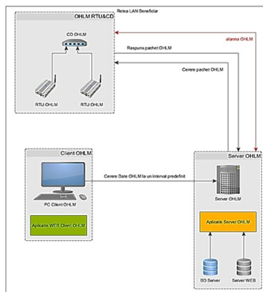
Fig. 6.5.1. NOVA OHLM software architecture
