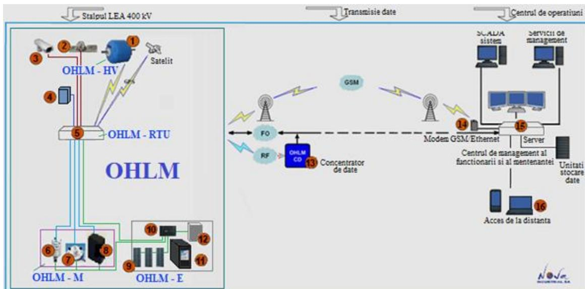
Fig. 6.2.1. Nova OHLM system architecture
