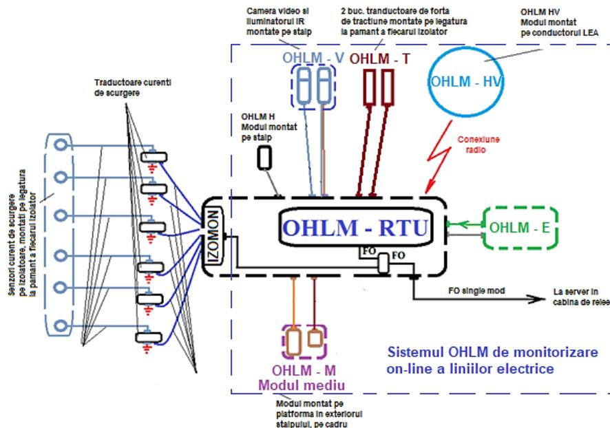
Fig. 6.6.2. The architecture of the measurement system used in the pilot project on-line monitoring of the 400 kV OHL Bucharest South - Pelicanu
