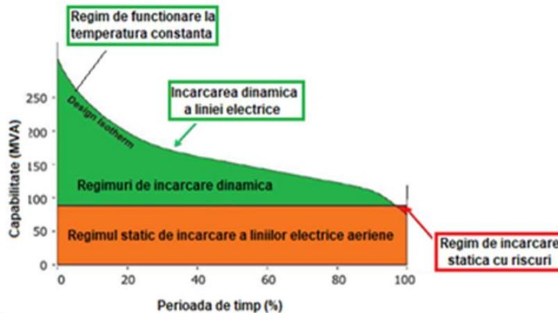
Fig. 4.4.1. Static and dynamic loading regimes of an OHL
