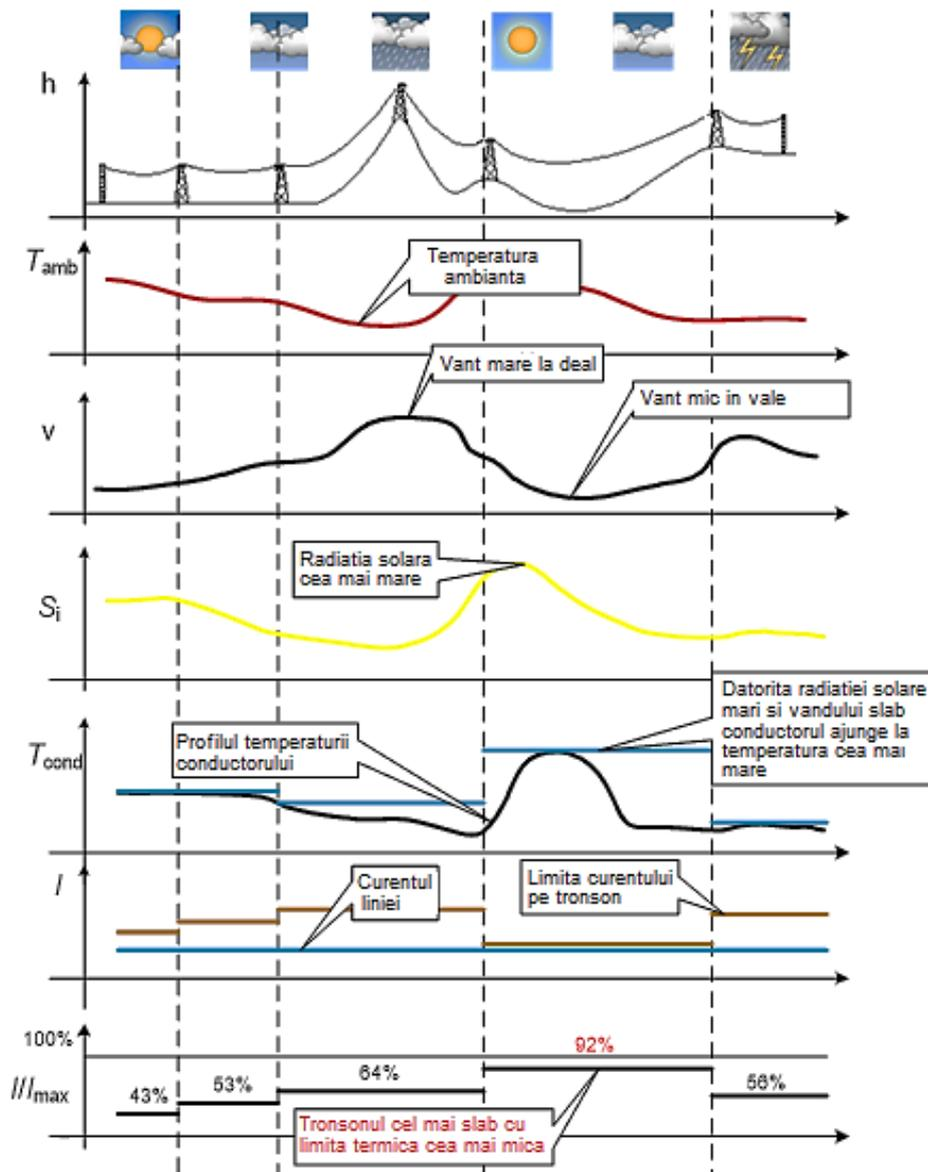
Fig. 4.2.1. The variety of factors that influence the carrying capacity of a transport OHL
