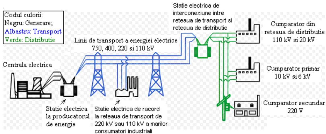
Fig. 3.1.1. Schematic diagram of the transfer of electricity from producers to consumers
