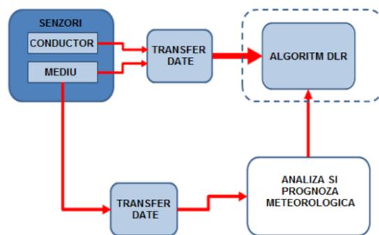
Fig. 4.4.4. Technological scheme for the application of the dynamic loading regime of the OHL
