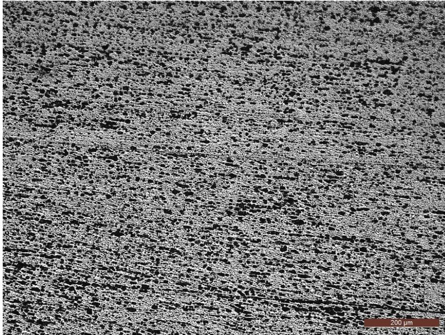
**Fig.2.11 x100** Base metal microstructure
