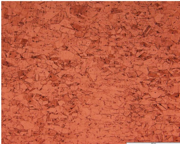
**Fig. 4.14** Microstructure of base metal stainless steel
