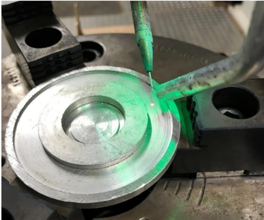
**Fig. 3.8** Sample positioning and fixing device for braze-welding
