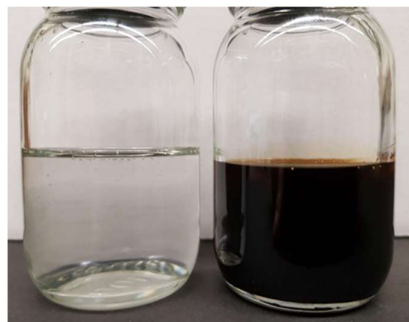
Figure 1 Glycolysis product obtained from flexible PU foam waste and diethylene glycol in a 1:1 (w/w) ratio, in autoclave (image on right), compared to virgin polyol (image on left)
