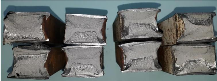
**Fig.3.38** Macrographic specimens with notch, API 5L X65M, 42 "(1066.8mm) x31.75mm after testing
