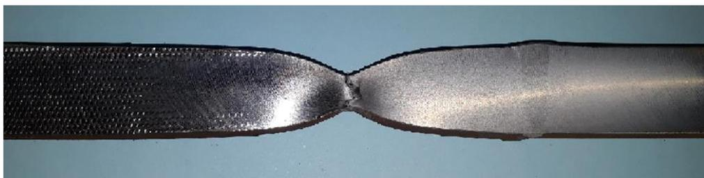
**Fig.3.28** Fracture location of the tensile strength test specimen
