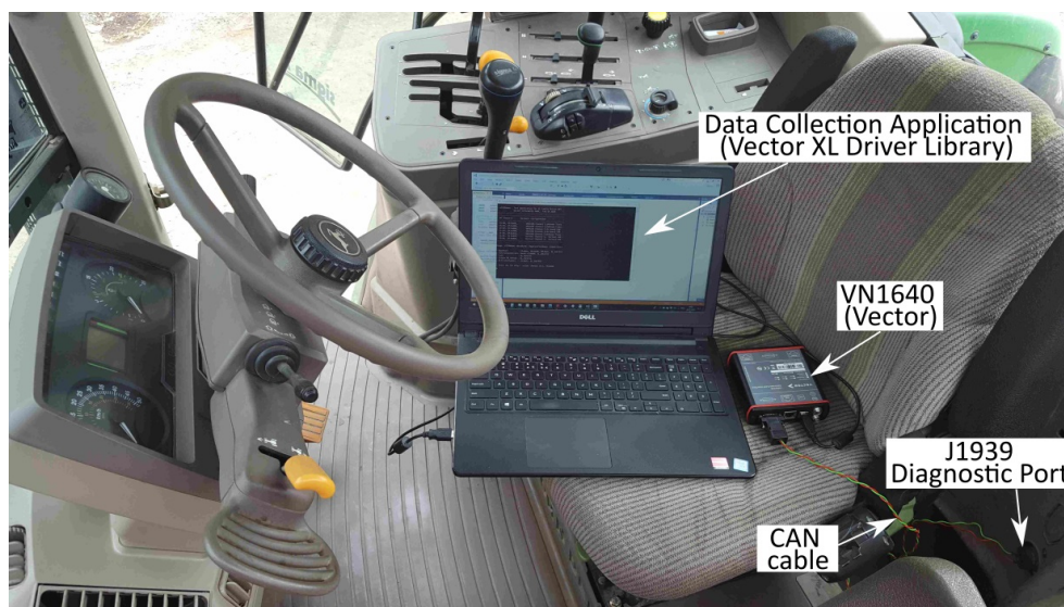
Fig. 1. A typical heavy-duty vehicle implementing the SAE J1939 standard and tools for data collection of the CAN traffic
