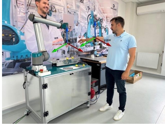
Fig. 13- Myo Armband application on Universal Robots UR10e
