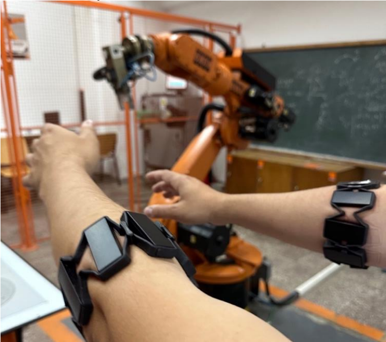
Fig. 12- Dual Myo application on KUKA KR15
