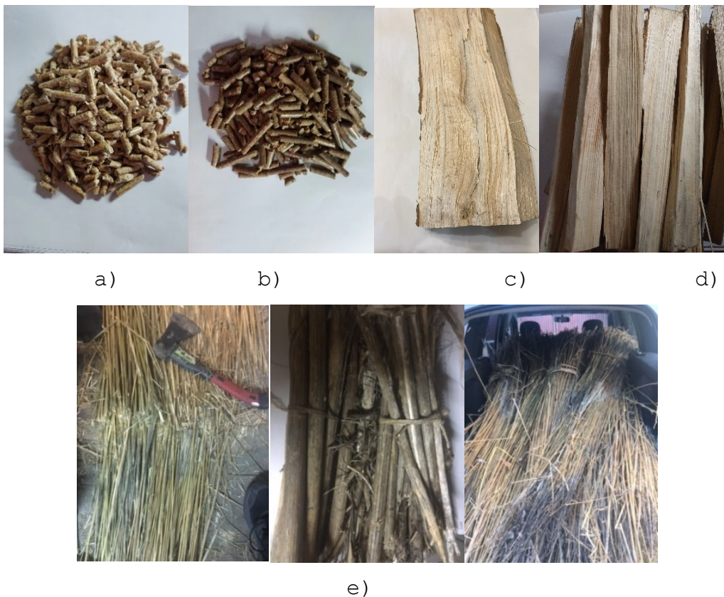
Figure 5. 2. Materials chosen for the combustion process: a)resinous pellets, b)beech pellets with fir, c)hornbeam, d)resinous, e)hemp
