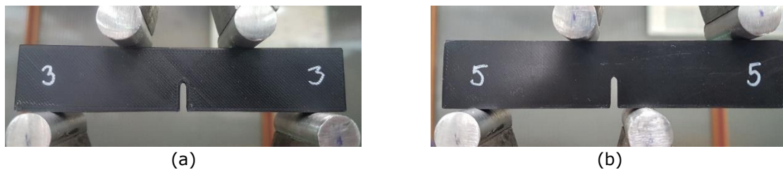
Fig. 6. Positioning of the SENB specimen on the Walter+bay 10 kN machine clamp: mode I (a) and mode II (b) of loading
