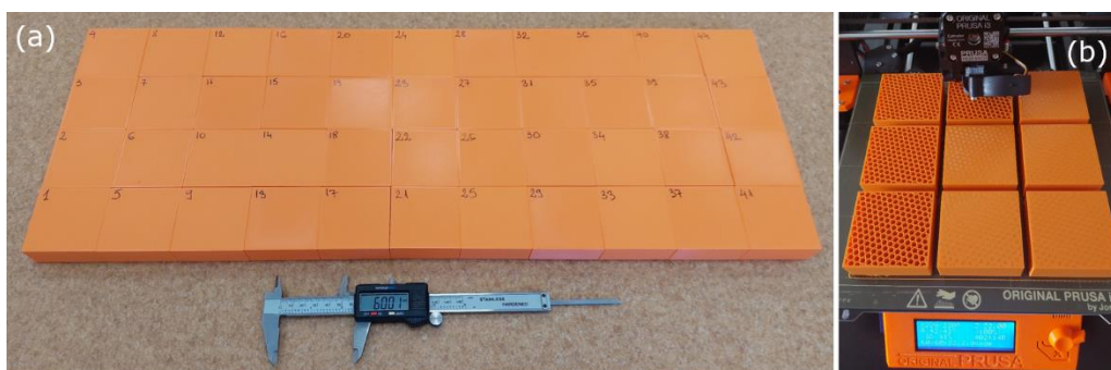
Fig. 7. 3D printed specimens used for impact testing: overview (a) and manufacturing process (b)
