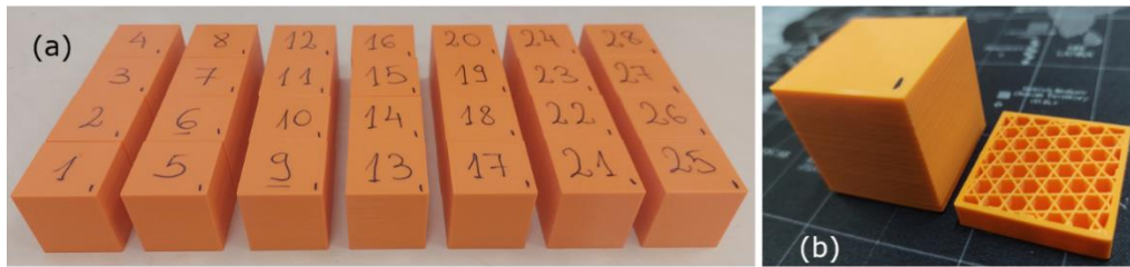
Fig. 9. 3D printed specimens for fatigue tests: overview (a) and internal structure (b)
