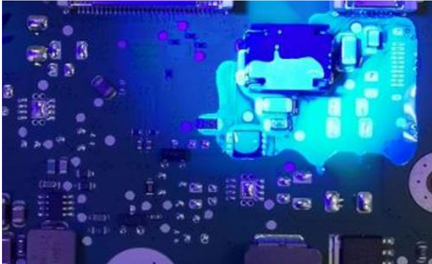
Fig.6.5. Varnish applied on the PCB, visible only when exposed to UV light
