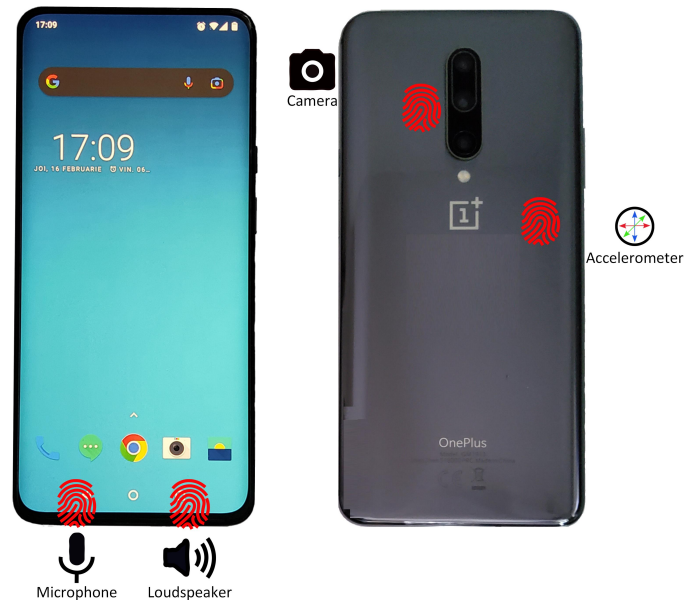
Fig. 1. A generic smartphone with sensors and transducers subject to fingerprinting
