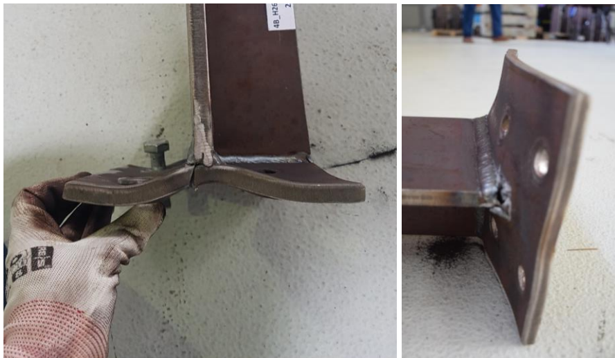
Fig. 5-10 End-plate deformed shape for HEA260 (left) and IPE360 (right)
