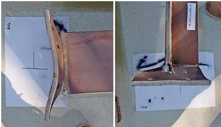
Fig. 4-5 End-plate deformation and weld failure from 4B_I360_t12_M16_P3
