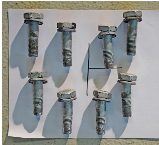
Fig. 4-4 Tested bolts from 4B_I360_t12_M16_P3
