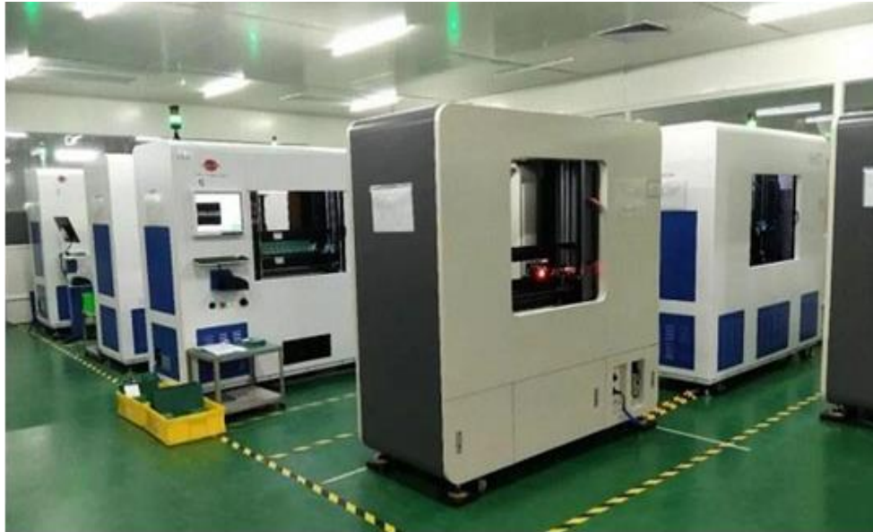
Figure 6: Automatic PCB testing system. Personal archive
