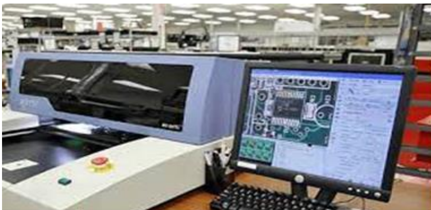
Figure 5: AOI System. Personal archive
