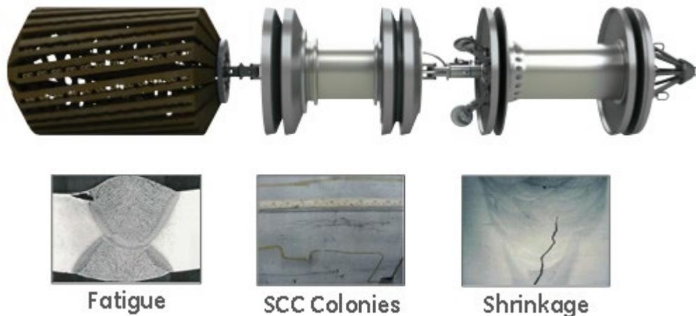
Figure 1. UltraScan CDP [2] (top) and sample crack categories [11] (bottom)
