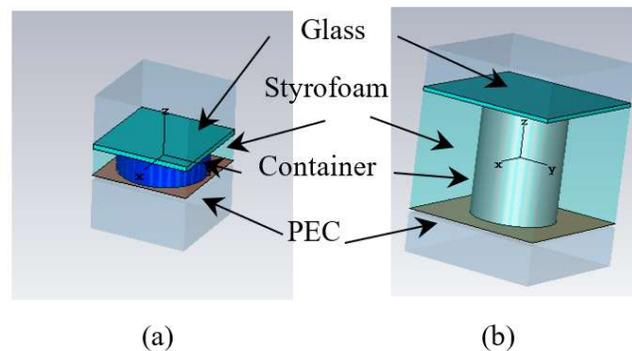
Figure 19. CAD model of the unit cell of the absorber based on liquids:
