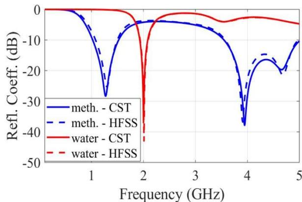
Figure 21. Joint representation of the reflection coefficient obtained by two different simulation software packages [Dsa, 2024]
