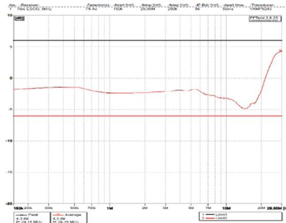
Figure 7. The measurement result with metal strips added to the antenna counterweight [silaghi, 2019]: X-axis: Frequency (Hz); Y-axis: Equivalent Electric Field Intensity (dBµV/m)
