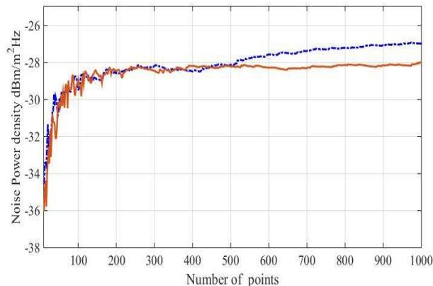
Figure 13. Noise level function of number of measure points [pacurar,2020,2]
