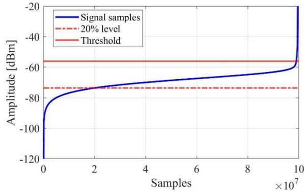
Figure 14. Sorted samples and threshold level [pacurar,2020,1]
