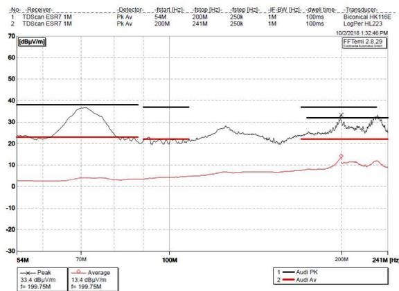
Figure 8. Initial far field measurement [pacurar, 2019]: X-axis: Frequency (Hz); Y-axis: Electric Field Intensity (dBµV/m)
