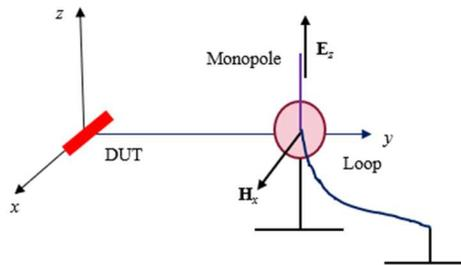
Figure 11. Spatial placement of the DUT and antennas. [pacurar,2022]
