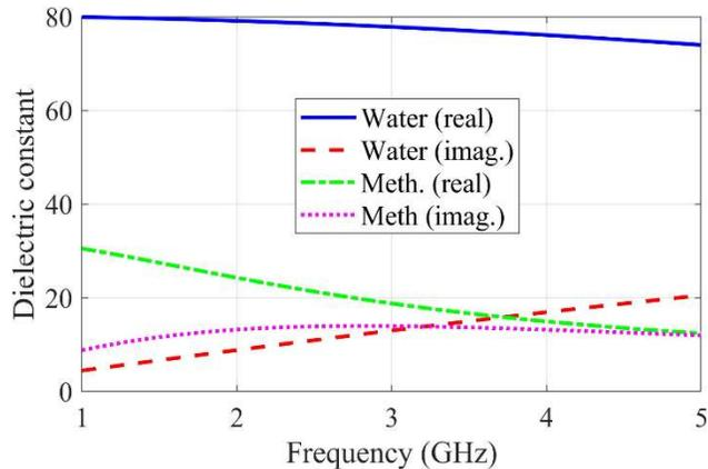
Figure 20. Dielectric constants of water and methanol at 20°C [Dsa, 2024]
