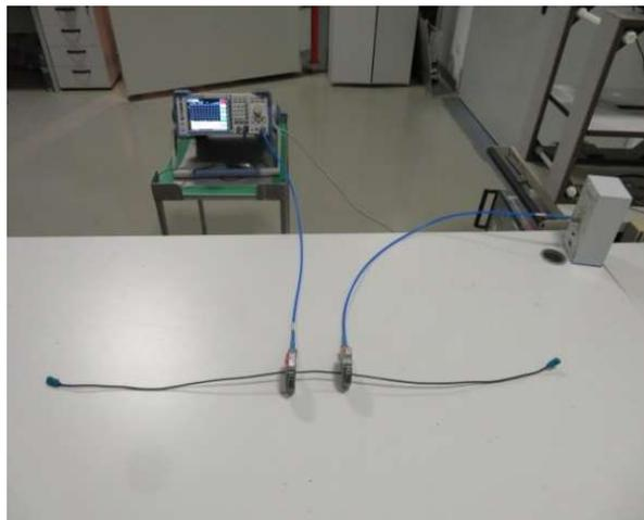
Figure 3. Experimental setup for measuring the resonant frequency in cables
