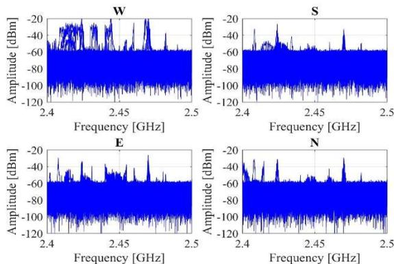
Figure 16. The spectrum of the signal from the four geographical directions [pacurar,2020,1]
