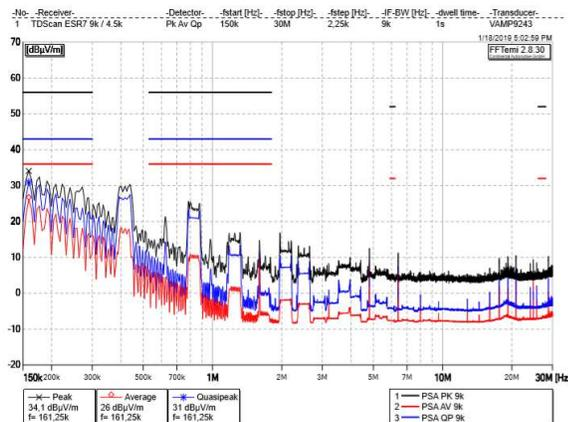
Figure 5. Radiated emissions measurement with Monopole Antenna:
