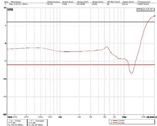
Figure 6. Initial measurement [Silaghi, 2019]: X-axis: Frequency (MHz); Y-axis: Equivalent Electric Field Intensity (dBµV/m)
