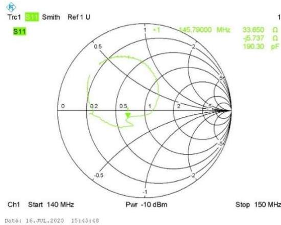
Figure 2. Smith Chart for the 145 MHz NMHA Antenna
