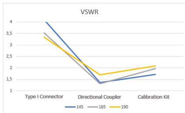
Figure 1. Variation of VSWR using different types of connectors
