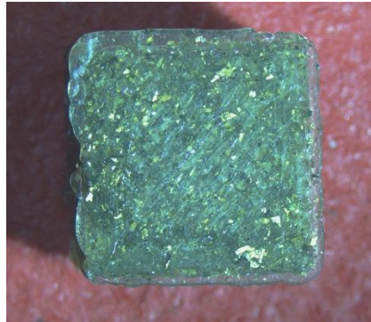
Figure 18. Macroscopic image of the distribution of particles and short bands in the 3D printed sample
