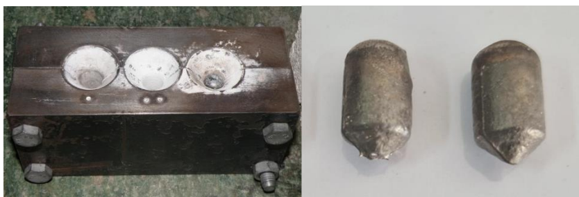
Figure 10 Casting form of primary alloy and solidified primary alloy
