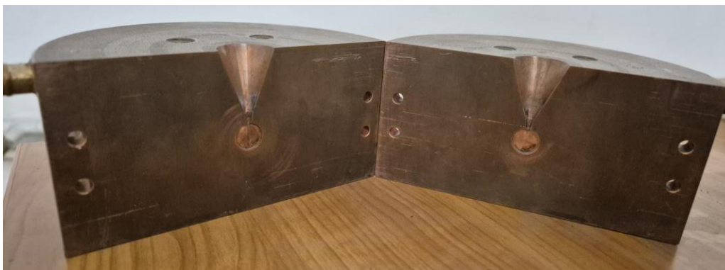
Figure 12. Copper mold for obtaining massive amorphous alloys in the form of discs
