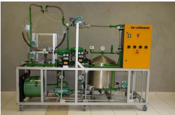
Fig. 1. Pilot plant for industrial process control.
