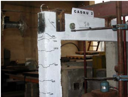
Damage of un-strengthened frame
