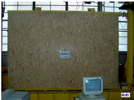
Full scale testing of wall-panel
