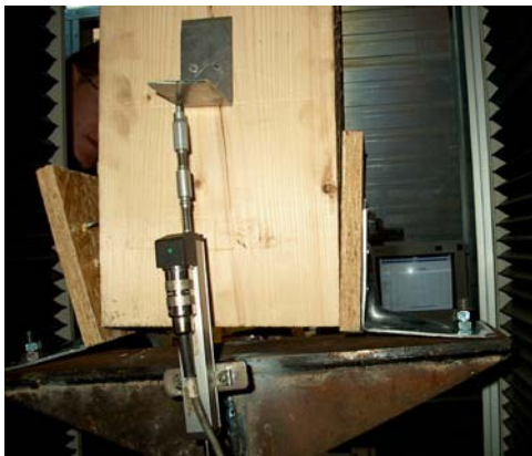
Failure of corner specimen due to eccentricity
